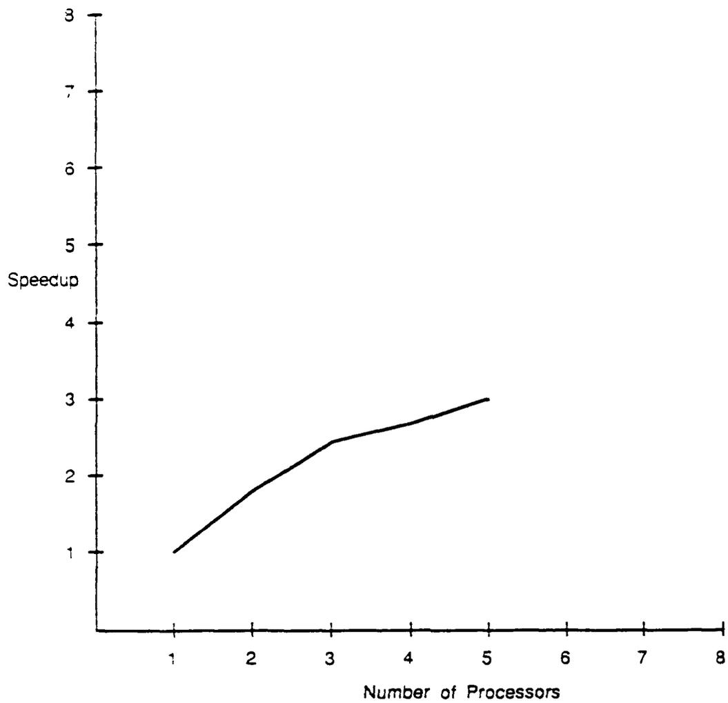
Figure 7: Speedup curve of LANZ on a Cray Y-MP
