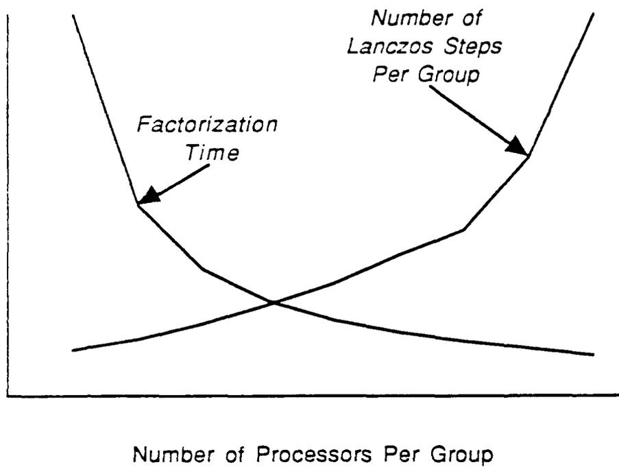
Figure 14: The tradeoff between factorization time and the number of Lanczos steps
