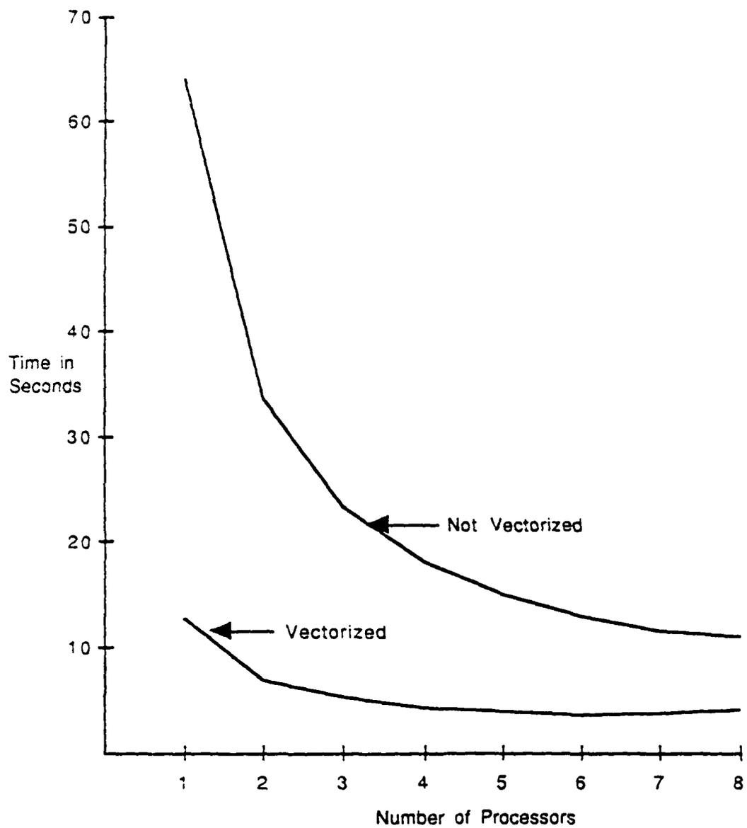
Figure 8: Estimated performance of vectorized vs. unvectorized versions
