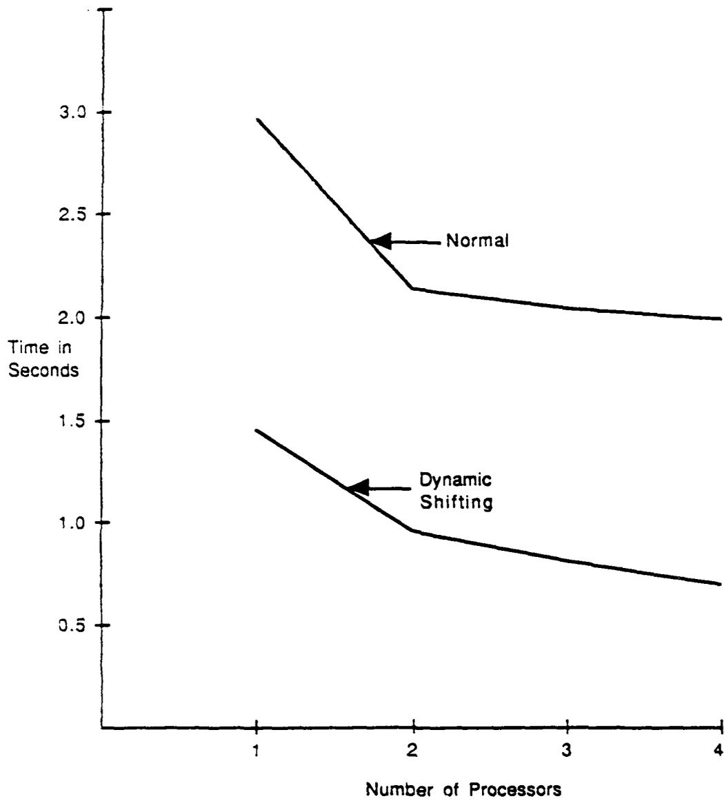
Figure 10: Execution time with and without dynamic shifting
