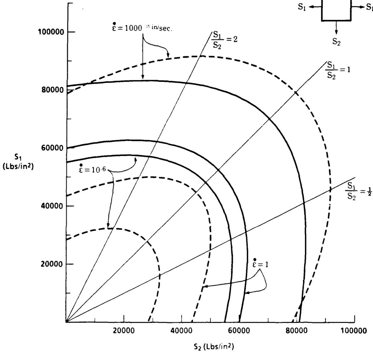
FIGURE 4. PLANE STRESS YIELD AND FRACTURE CRITERIA OF MILD STEEL AT VARIOUS STRAIN RATES
