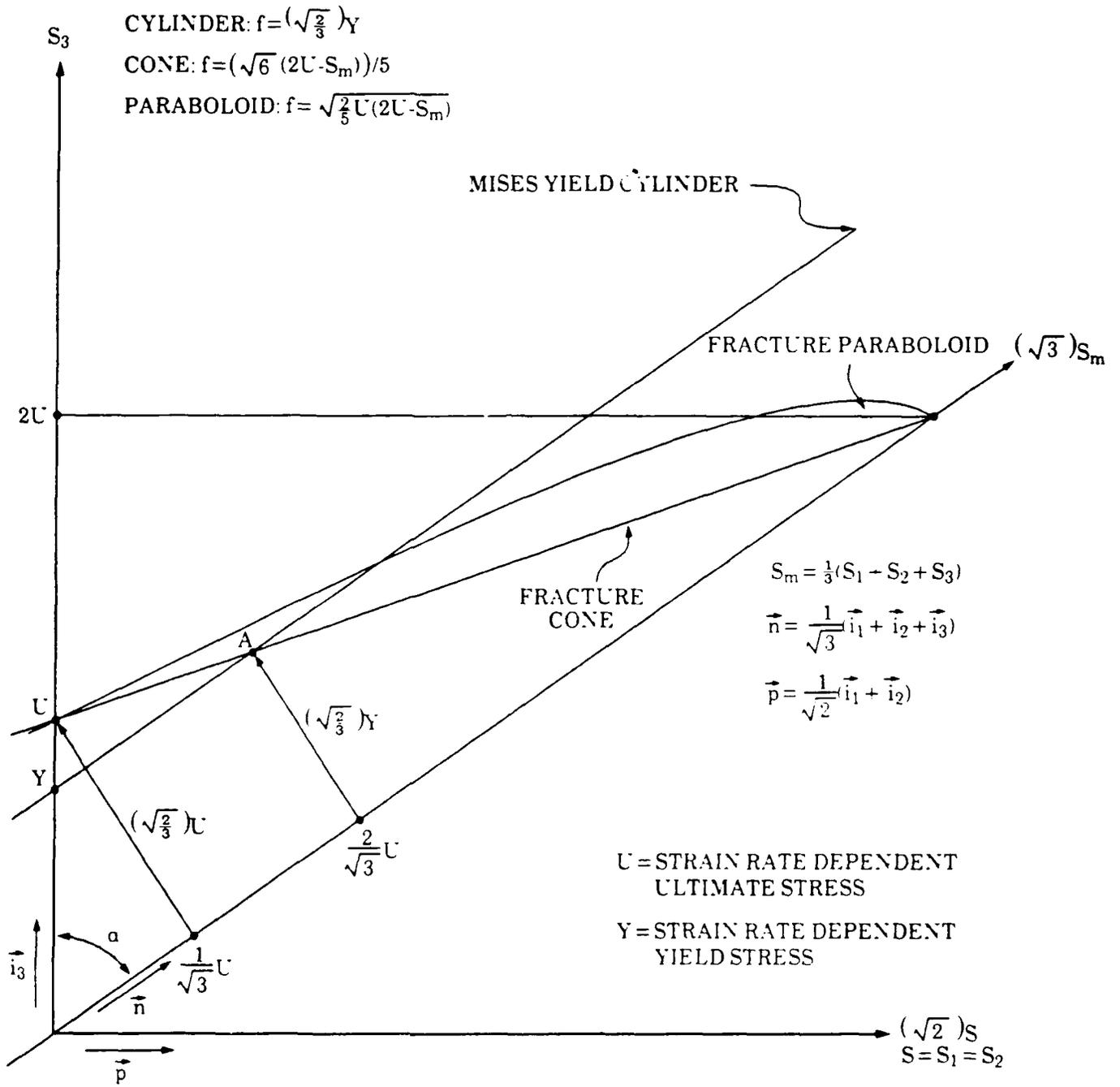
FIGURE 3. REPRESENTATIONS OF CRITERIA IN  $S_1$ - $S_m$  PLANE
