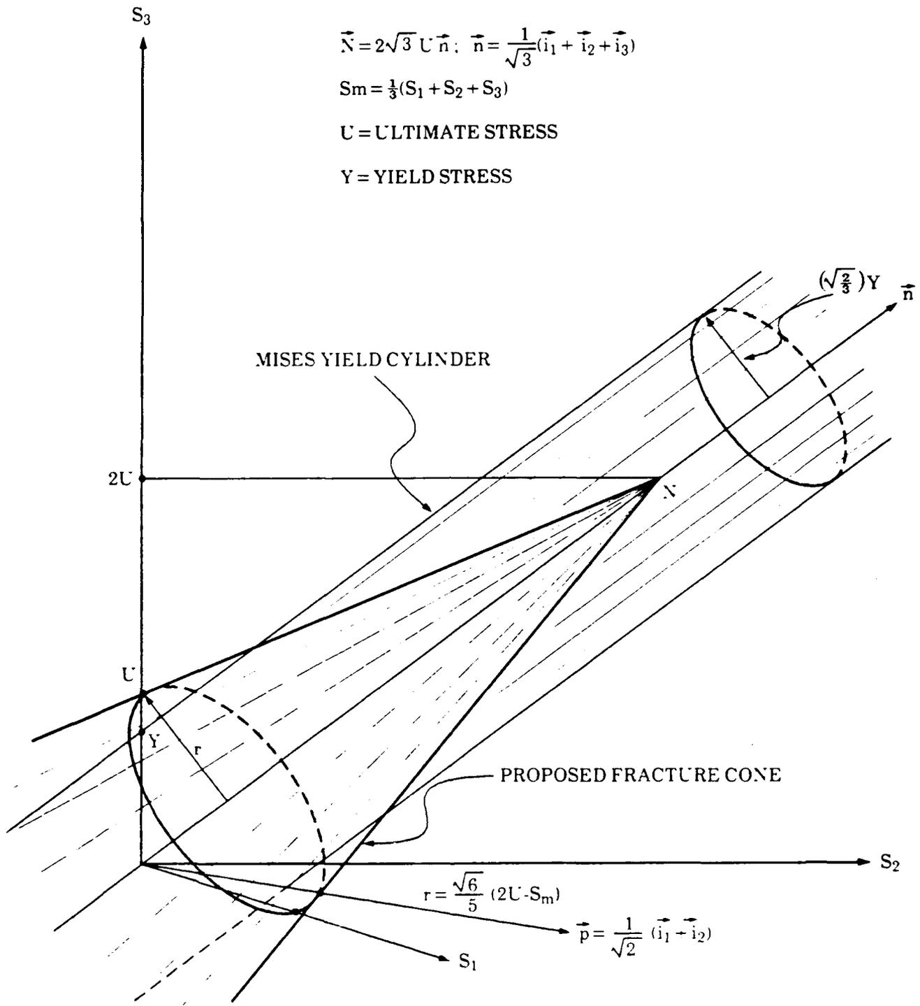
FIGURE 2. GEOMETRICAL REPRESENTATION OF FRACTURE AND YIELD CRITERIA
