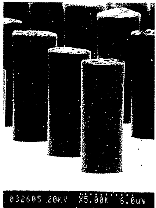
Fig. 9 Nickel plated LIGA-like test structure. Fig. 9 illustrates plating resolution. The structures are nickel columns of 5\ \mu\text{m} diameter and 18\ \mu\text{m} height.
