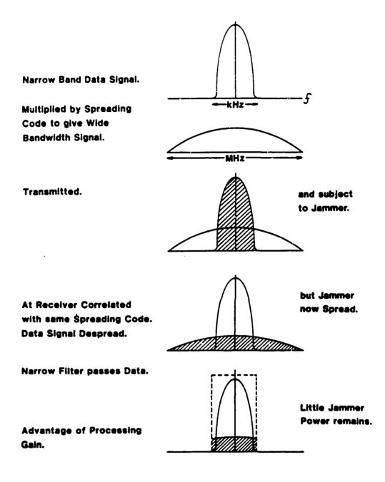
Figure 2. Jamming Protection Through Spread Spectrum
