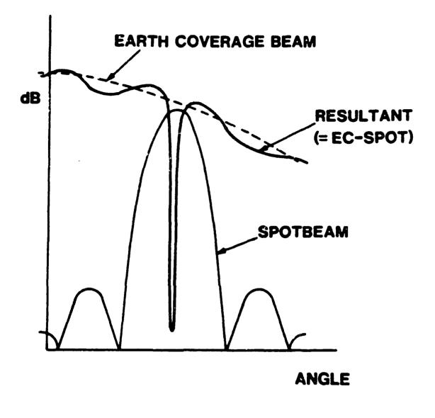
Figure 1. Illustration of Antenna Null Realization
