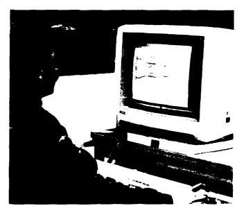
The ATOS operator can scan, key in, or import text and graphics from a variety of sources. The result is a photo-ready paper master copy. The USAF acquired ATOS for use in making changes to paper TOs. A system that can accept, store, distribute, and manage digital TO data still is required.
