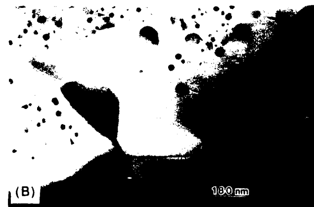
Fig. 1. Typical microstructure of ZrO_2 -toughened Al_2O_3 showing (A) intergranular and (B) intragranular ZrO_2 particles; a few particles are arrowed.
