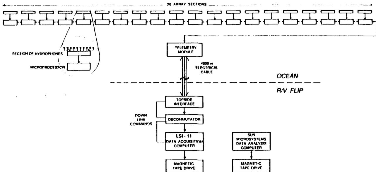
Fig. 3. Array System Diagram. The data path from the hydrophones through the telemetry module to the magnetic tape drive is shown. Further analysis of the data is accomplished by a Sun Microsystems computer.
