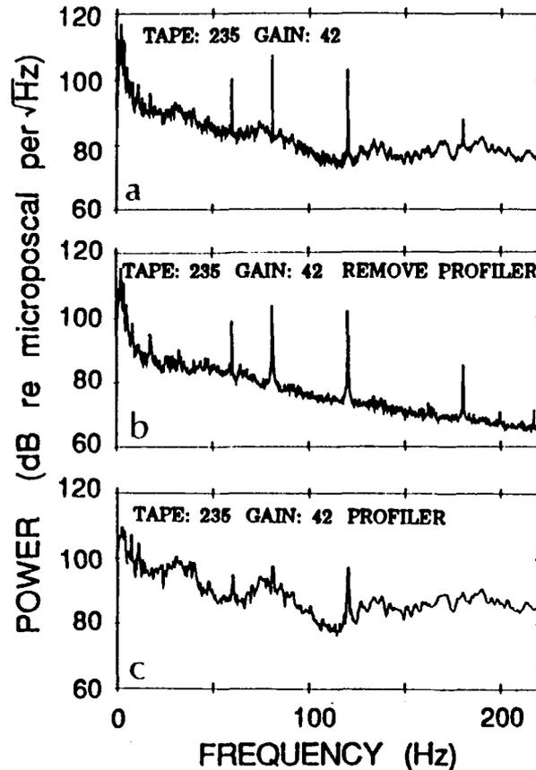
Fig. 9. Seismic profiler contamination. The effect of the air gun signal is seen to be clearly contaminating the ambient noise spectra. (a) Original data acquired at array channel 24. (b) Same data as (a) with profiler signal removed. (c) Profiler signature as seen at the array.
