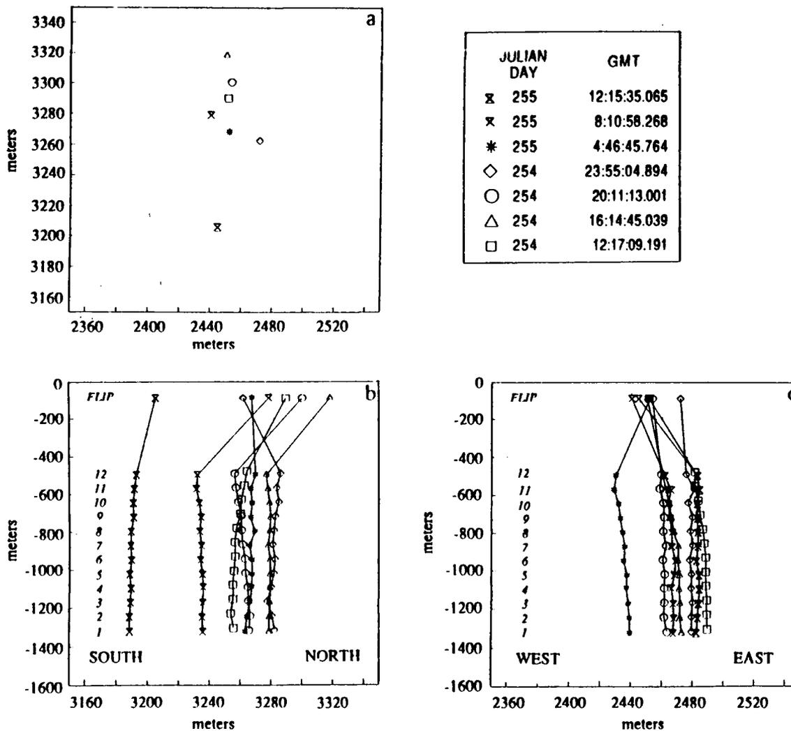
Fig. 5. Navigation Results. A time series of the array position sampled approximately every four hours. The three plots represent (a) a plan view in  $X$  (increasing toward the east) and  $Y$  (increasing toward the north), (b)  $X$  versus depth, and (c)  $Y$  versus depth. The scale in (b) and (c) is enhanced in the vertical direction by 8:1.
