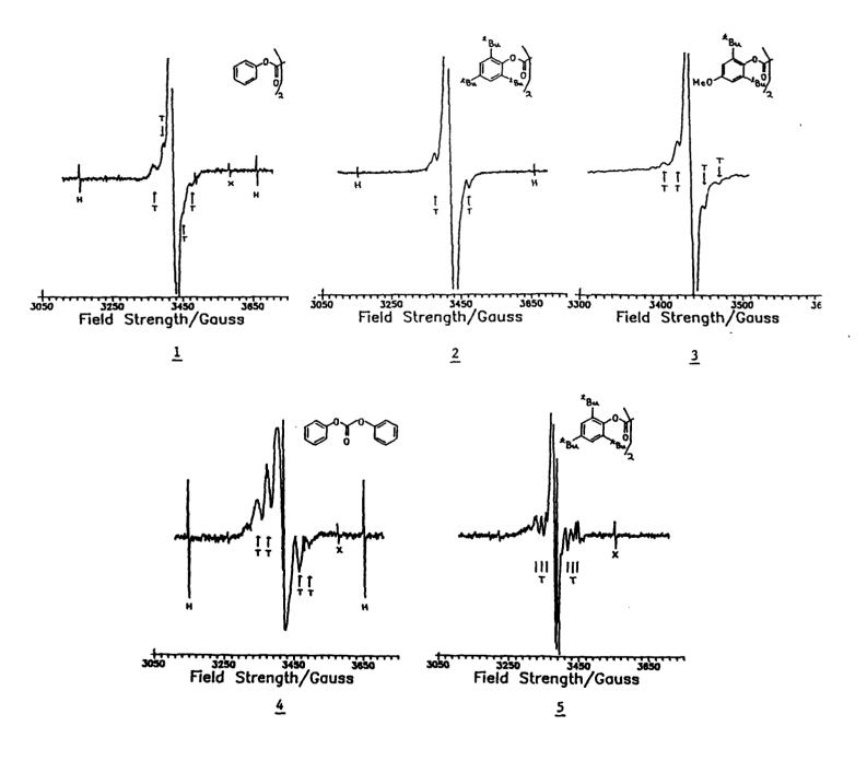
Spectra 1-3 are of neat powder samples, spectra 4-5 are taken for crystalline samples aligned with long axes approximately parallel to the sample tube. Triplet radical pair transitions are marked with "T". Peaks marked "X" or "H" are due to impurities unrelated to the phenoxyl radicals.
