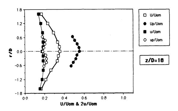
Figure 6. Radial distributions of streamwise velocities of single-phase and particle flows at z/D=18
