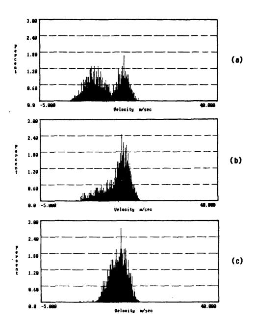
Figure 2. Effect of trigger level on "cross-talk"
