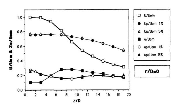
Figure 3. Centerline distributions of streamwise velocities of single-phase and particle flows
