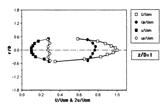
Figure 4. Radial distributions of streamwise velocities of single-phase and particle flows at  $z=1\,\mathrm{D}$
