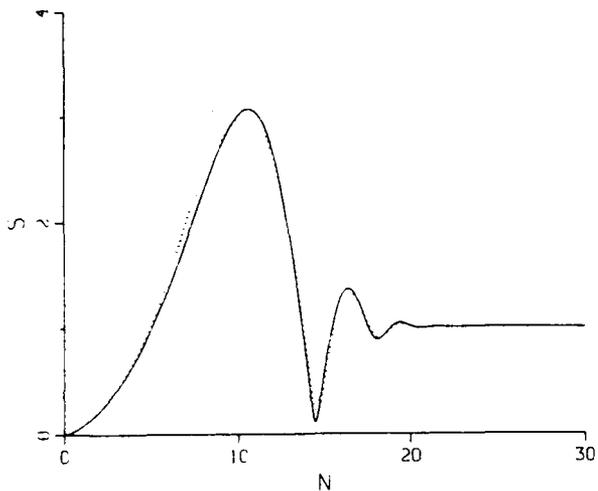
FIG. 1. Magnitude  $S$  in (1) vs  $N$  in kHz at range  $\rho = 320$ . The parameters are as in (17) for all figures, and  $h_r = h_r = 0.835$  for Figs. 1-7. The solid curve is based on (5), and the dotted curves (that equal the solid at large and small  $N$ ) are the large and small  $s$  approximations (8) and (11) with  $\bar{\zeta}' = 0$  (top), or (10) and (12) (bottom).
