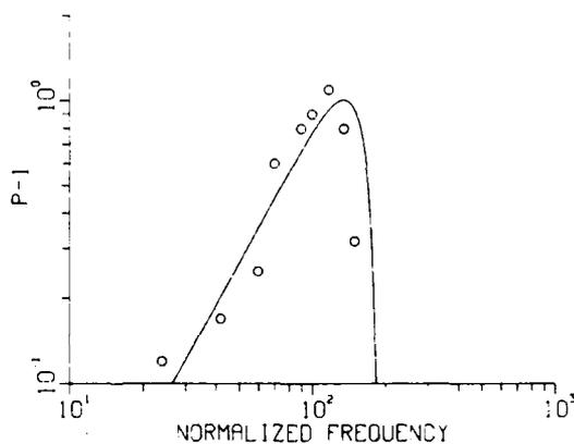
FIG. 8. Curve of  $P - 1$  of (1) based on (5) for  $h_1 = h_2 = 0.3$  compared with Fig. 4:10 data (for #1 gravel, at  $Z_1 = Z_2 = 0$  and  $\rho = 40$ ) versus  $k\rho = 7.32N$  and  $N$  varying from 4 to 20 in steps of 2.
