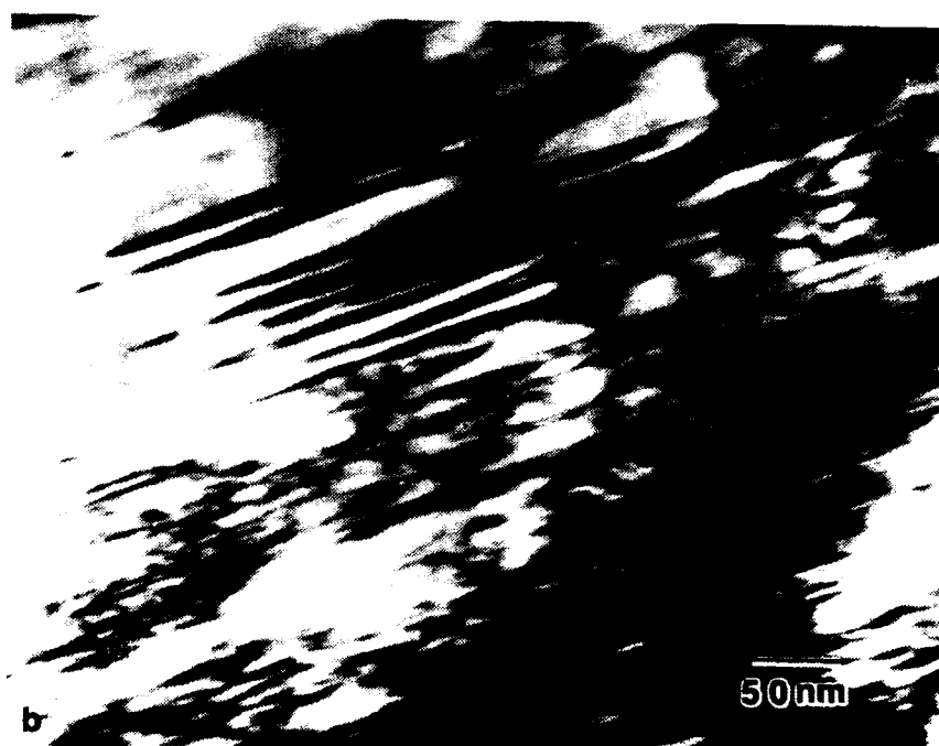
Fig. 8 Heavily twinned martensitic grains in the slow cooled microstructure: BF micrographs show (a) very fine twins about 5 nm wide and (b) larger twins.
