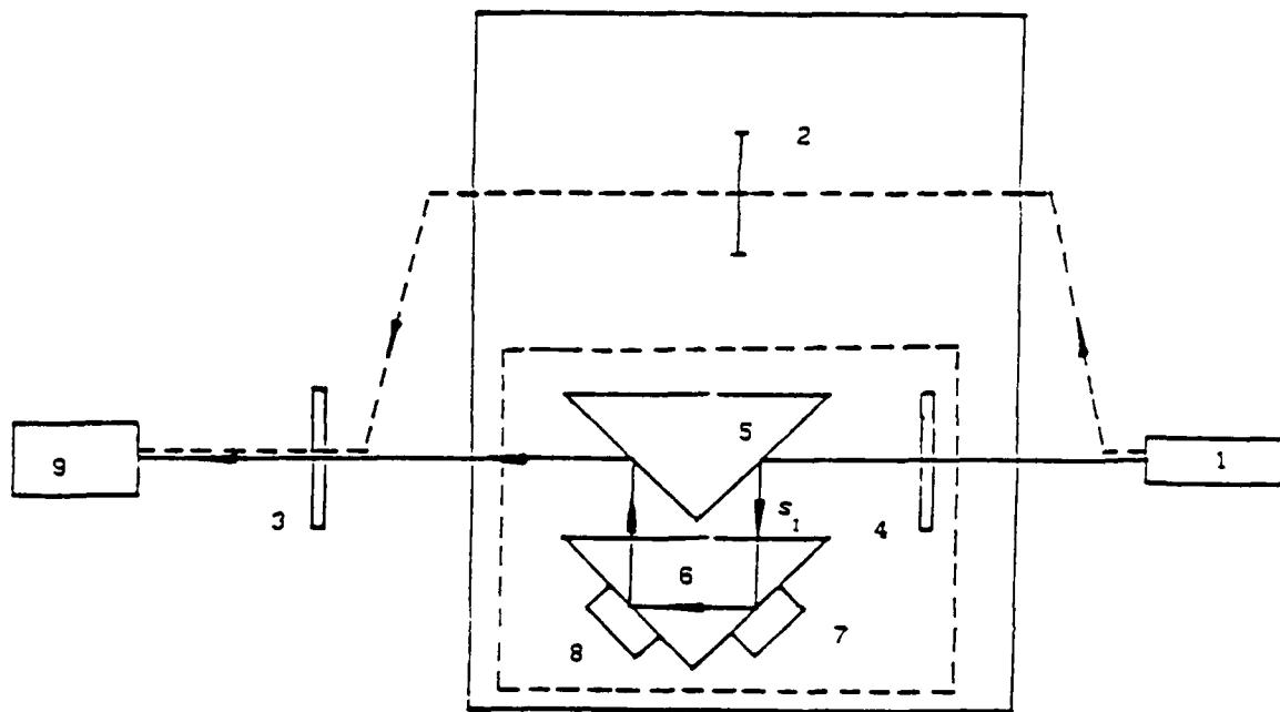
Fig. 5--The internal reflectance accessory installation in the spectrophotometer and schematic of the sample and reference beam.
