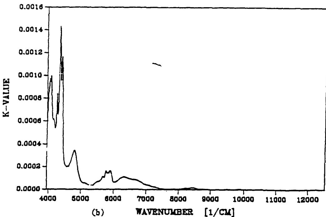
Fig. 5. Extinction coefficient  $k$  of ethyl alcohol: (a) in the  $500-3950 \text{ cm}^{-1}$  wave-number region; (b) in the  $3950-12500 \text{ cm}^{-1}$  wave number region.
