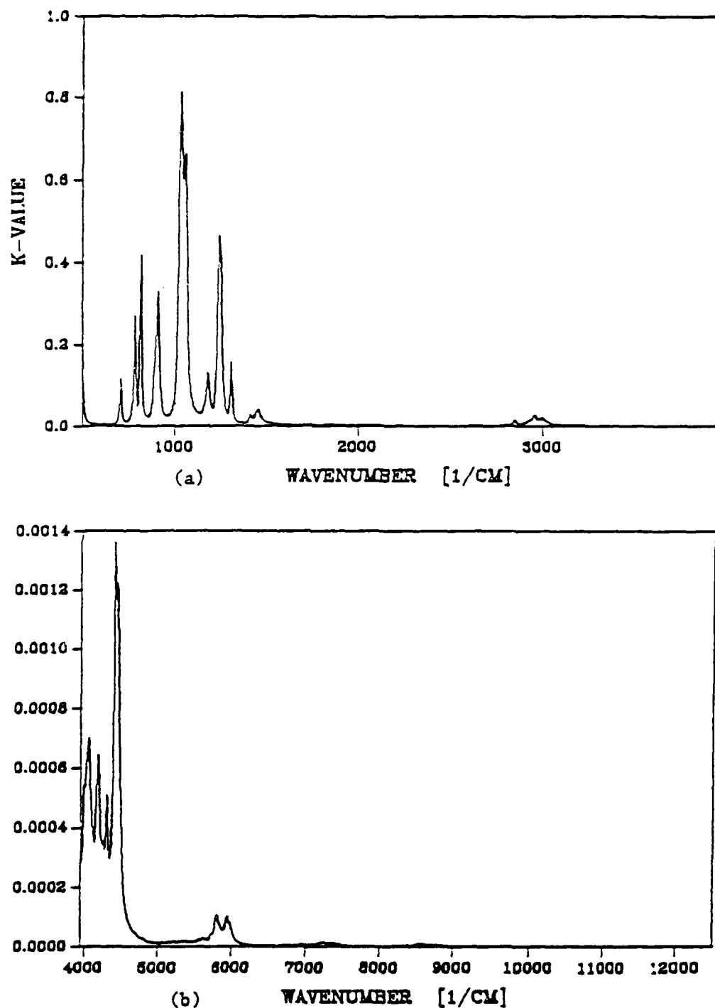
Fig. 19. Extinction coefficient  $k$  of dimethyl methylphosphonate: (a) in the  $500-3950\text{ cm}^{-1}$  wave-number region; (b) in the  $3950-12500\text{ cm}^{-1}$  wave-number region.
