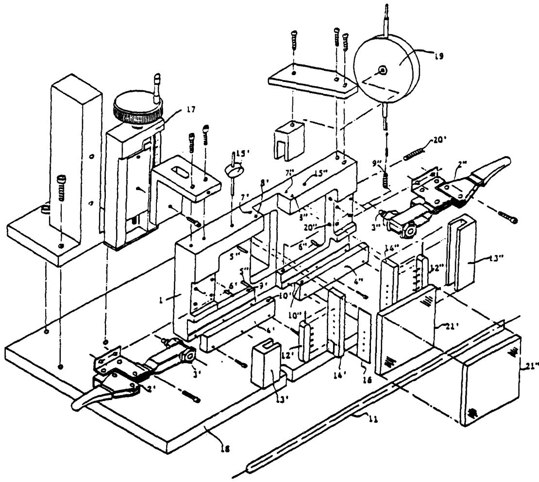
Fig. 2. An exploded drawing of components comprising a wedge-shaped cell unit for measuring the Lambert absorption coefficient of low and high absorbent liquids.
