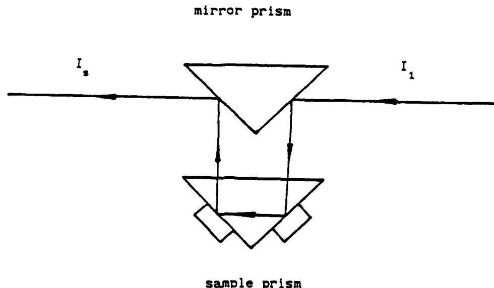
Fig. 16--The diagram of beam routine in the internal reflection accessory.
