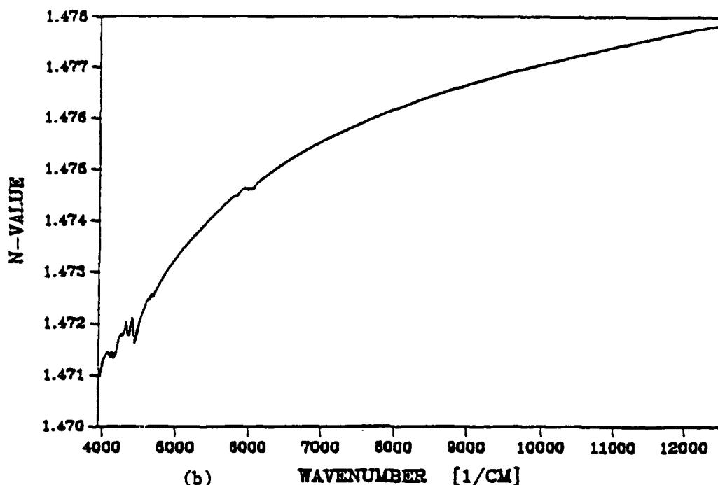
Fig. 18. Index of refraction  $n$  of diethyl phthalate: (a) in the  $500-3950\text{ cm}^{-1}$  wave-number region; (b) in the  $3950-12500\text{ cm}^{-1}$  wave-number region.
