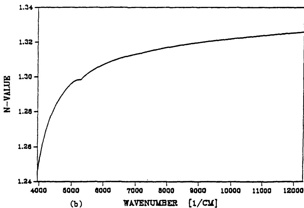
Fig. 4. Index of refraction  $n$  of water: (a) in the 500-
