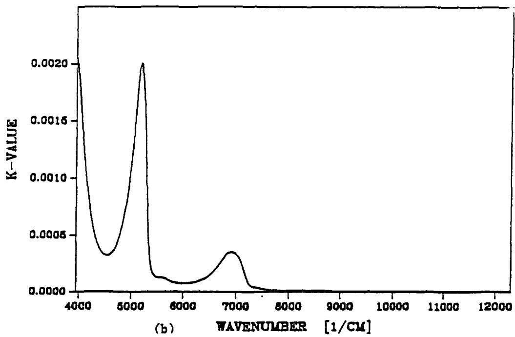
Fig. 3. Extinction coefficient  $k$  of water: (a) in the  $500\text{-}3950\text{ cm}^{-1}$  wave-number region; (b) in the  $3950\text{-}12500\text{ cm}^{-1}$  wave-number region.
