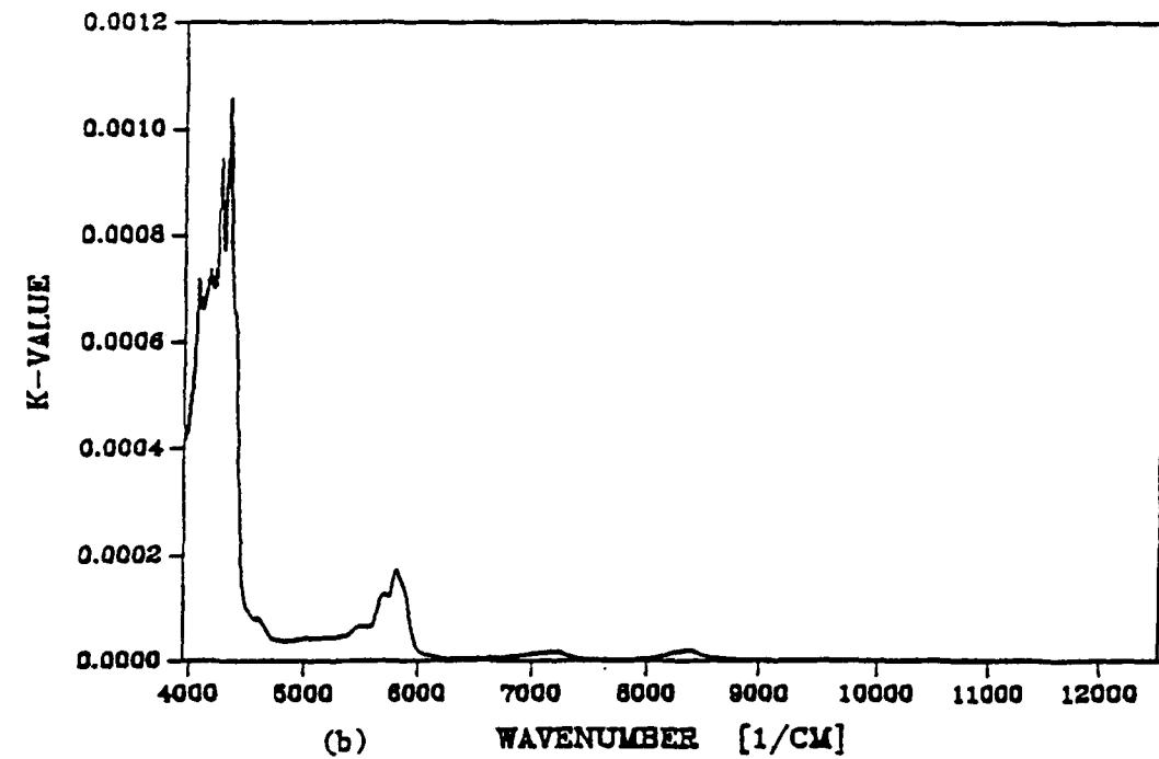
Fig. 13. Extinction coefficient  $k$  of fog oil: (a) in the  $500\text{-}3950\text{ cm}^{-1}$  wave-number region; (b) in the  $3950\text{-}12500\text{ cm}^{-1}$  wave-number region.
