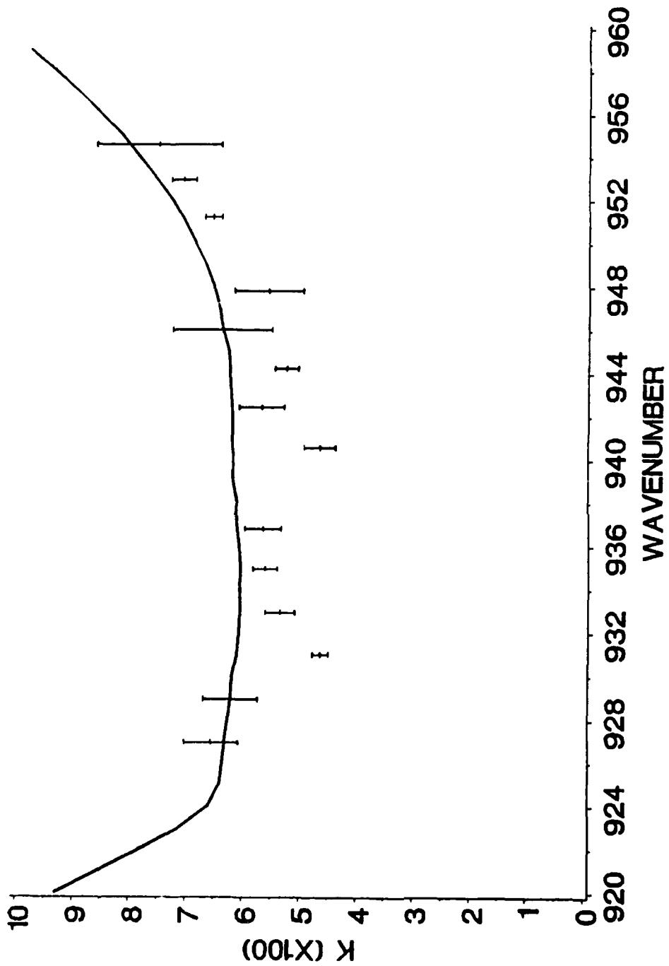
FIG. 1.13 Extinction coefficient for DIMP in the wavenumber region 920 to 960  $\text{cm}^{-1}$ . The  $\kappa$  values have been multiplied by 100. The solid line is data from Shengshan Weng's thesis. The data obtained with the  $\text{CO}_2$  laser is represented by the plus symbols and the error bars are  $\pm$  one standard deviation.
