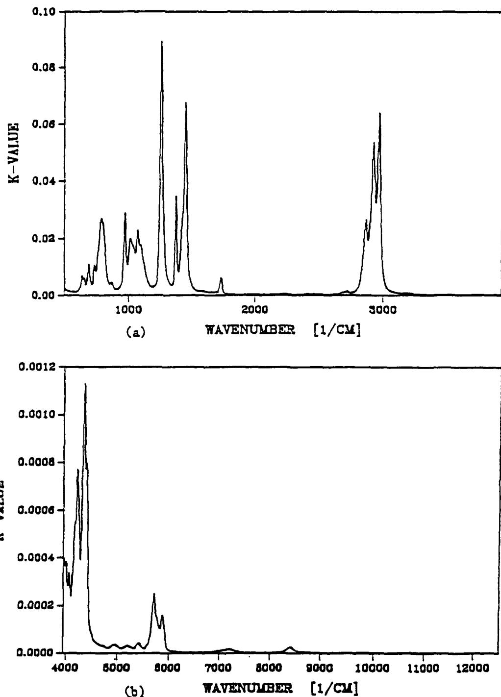
Fig. 15. Extinction coefficient  $k$  of ethyl sulfide: (a) in the  $500\text{-}3950\text{ cm}^{-1}$  wave-number region; (b) in the  $3950\text{-}12500\text{ cm}^{-1}$  wave-number region.
