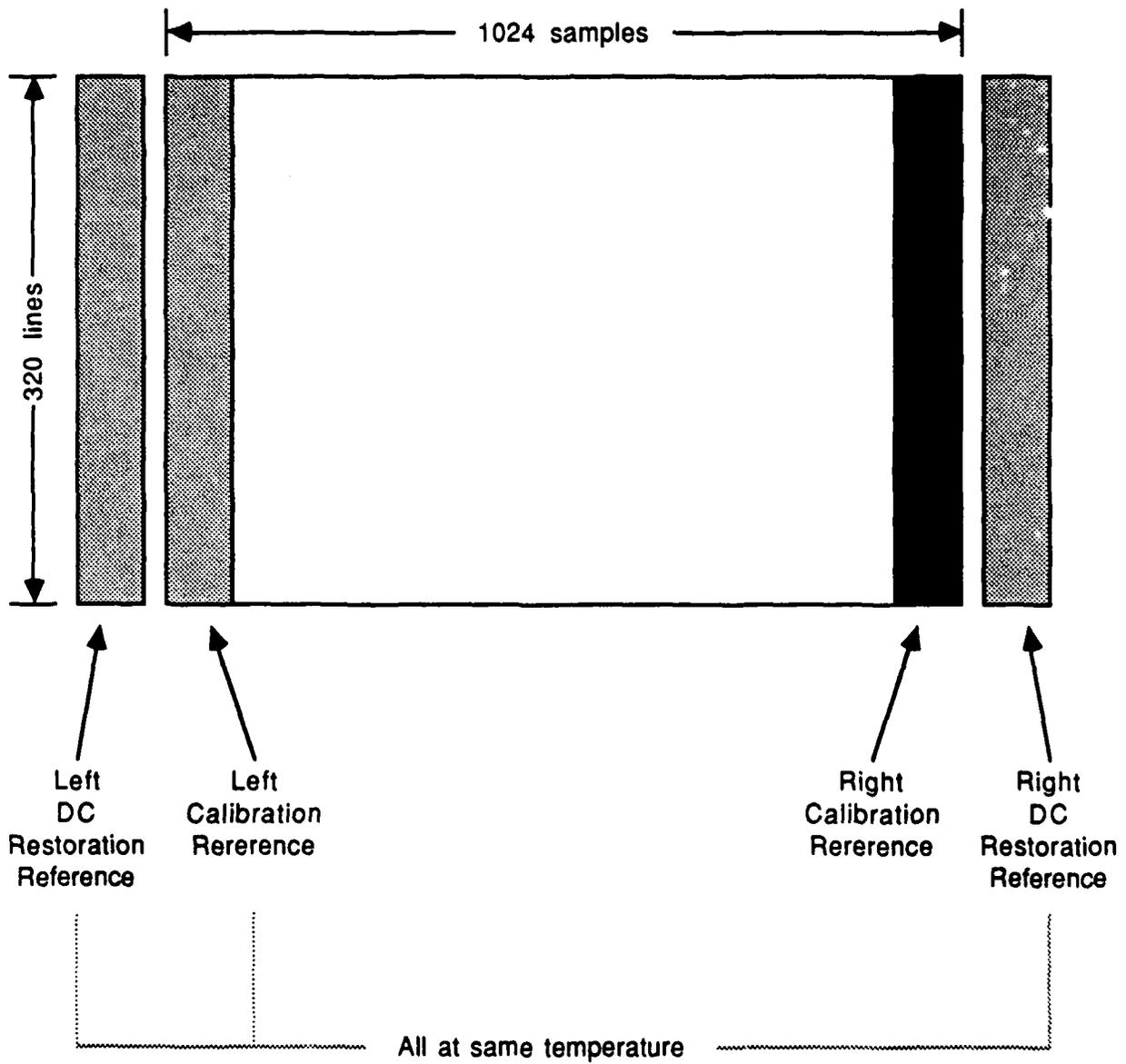
**Figure 3. CD-FLIR Reference Plane Source Configuration**
