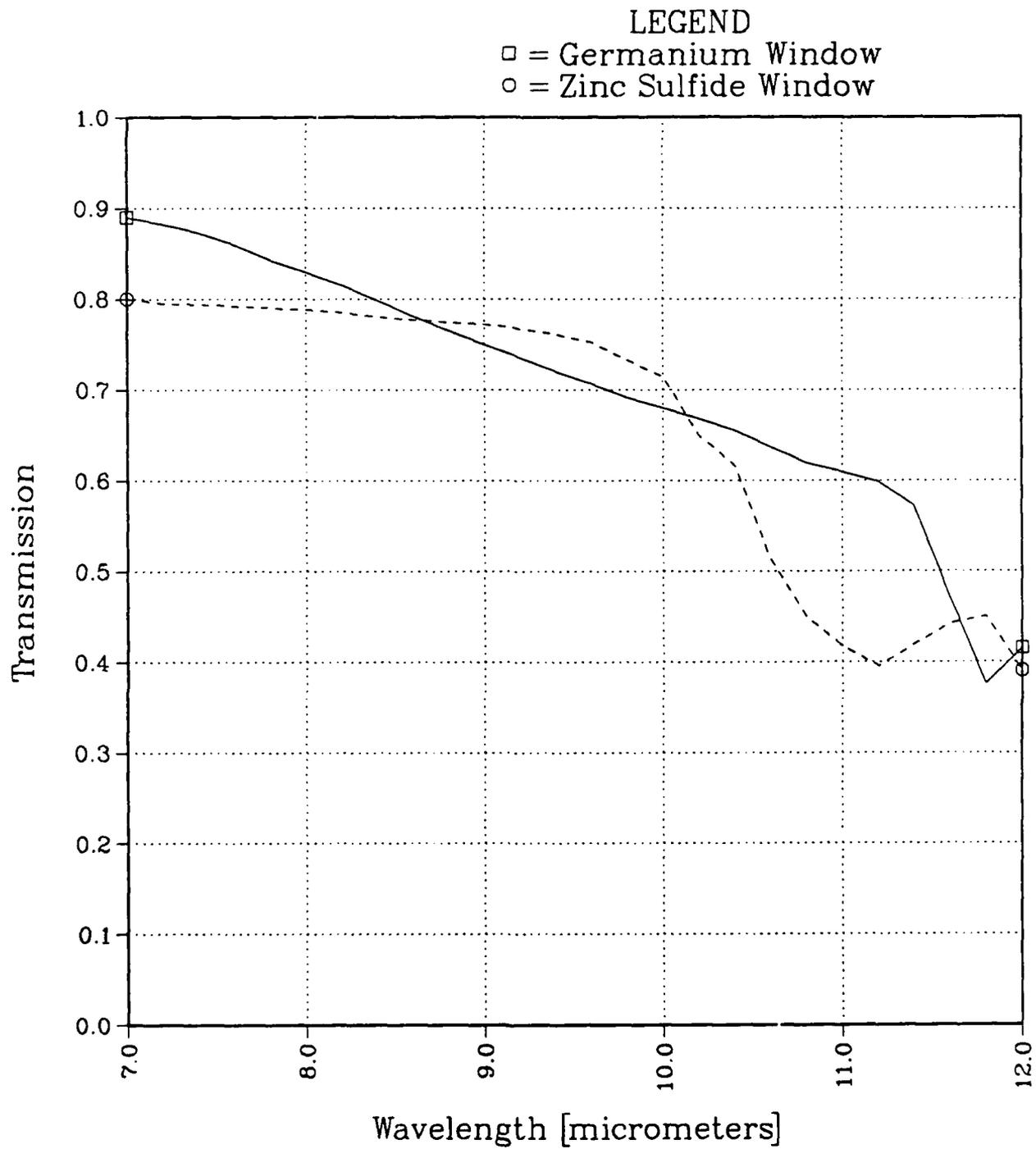
Figure 13. Aircraft Window Spectral Transmissivities
