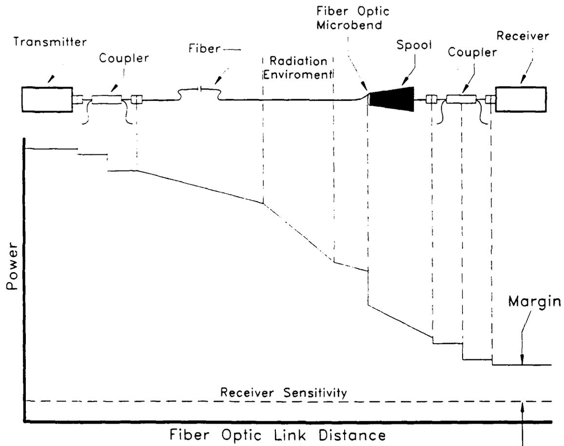
Fig. 3. Estimated power budget of a typical FOG-M fiber optic link.
