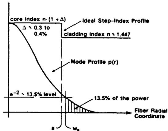
Fig. 2. Mode profile of electromagnetic radiation located in the cladding of a step-index singlemode fiber as a function of radial distance outward. (Lin et al.<sup>42</sup>)
