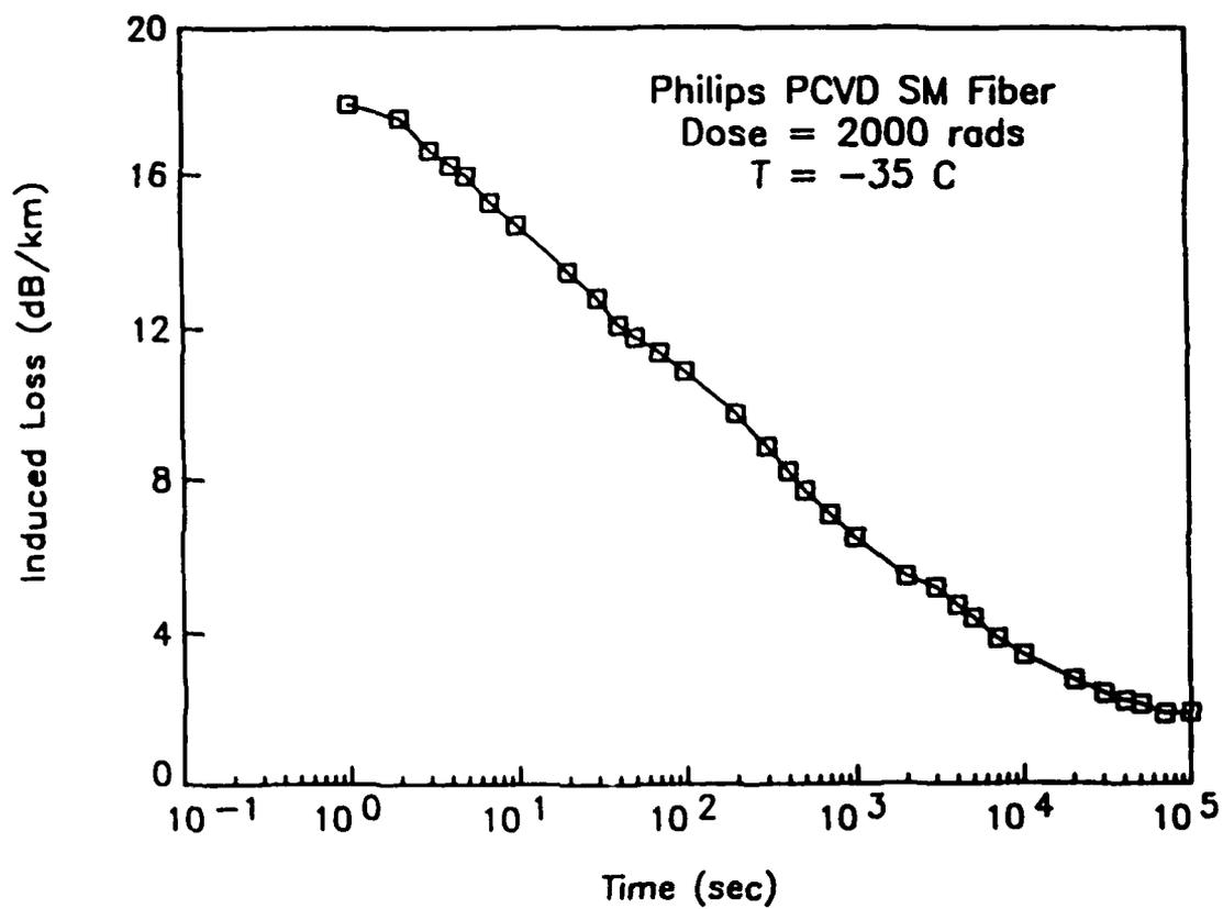
Fig. 11. Recovery data of a Phillips singlemode fiber made by the plasma chemical vapor deposition process. (Frebiele<sup>28</sup>)
