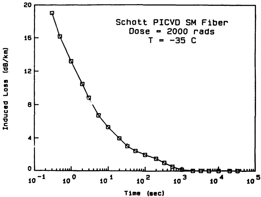
Fig. 10. Recovery data of a Schott commercial singlemode fiber made by the plasma impulse chemical vapor deposition process. (Frebiele<sup>28</sup>)
