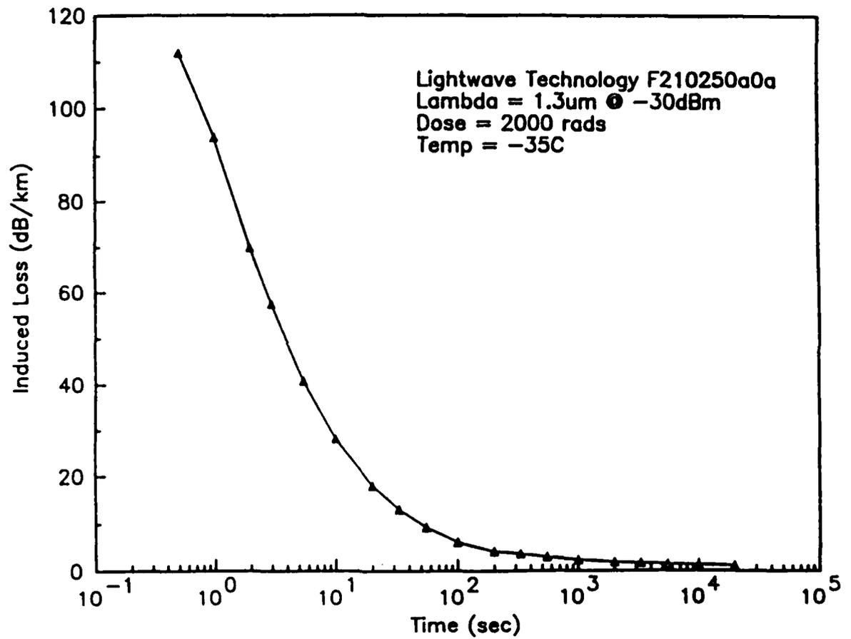
Fig. 9. Recovery data of Lightwave Technologies, Inc., commercial singlemode fiber. (Friebiele<sup>28</sup>)
