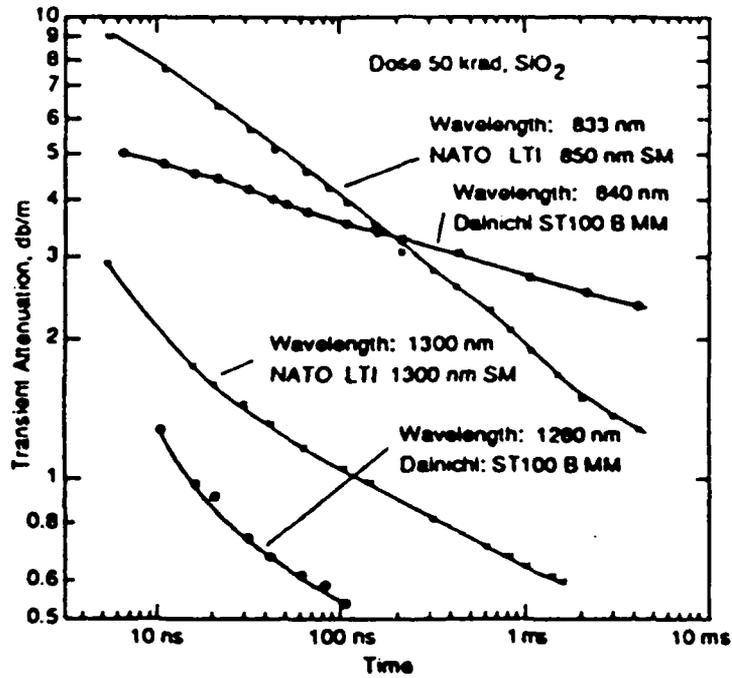
Fig. 4. Radiation induced attenuation as a function of time for various optical fibers. (Looney et al.<sup>40</sup>)
