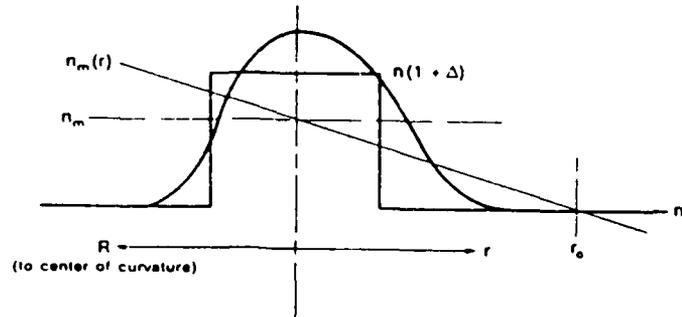
Fig. 1. Mode profile of electromagnetic radiation propagating through a step-index singlemode optical fiber at a bend located in the fiber as a function of radial distance outward. (Lin et al.<sup>42</sup>)
