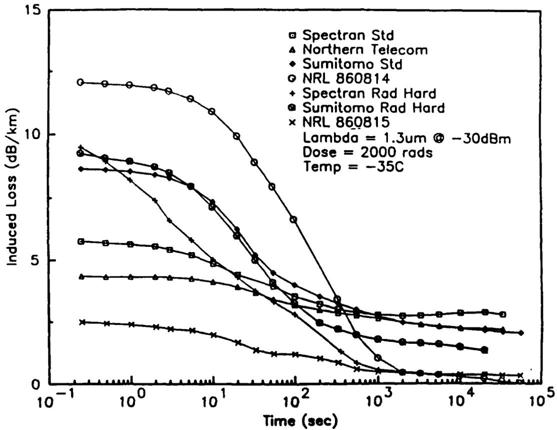
Fig. 6. Recovery Data of Northern Telecom, NRL, Spectran, and Sumitomo singlemode fibers and two NRL prototypes. (Friebiele<sup>28</sup>)
