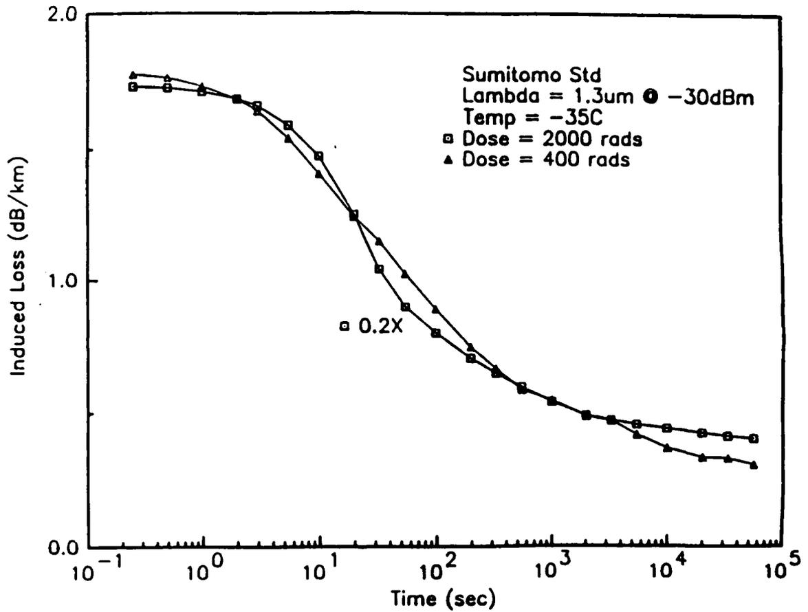
Fig. 5. Recovery of the attenuation induced in a Sumitomo singlemode fiber by doses of 2000 and 400 rads. (Frebiele<sup>28</sup>)
