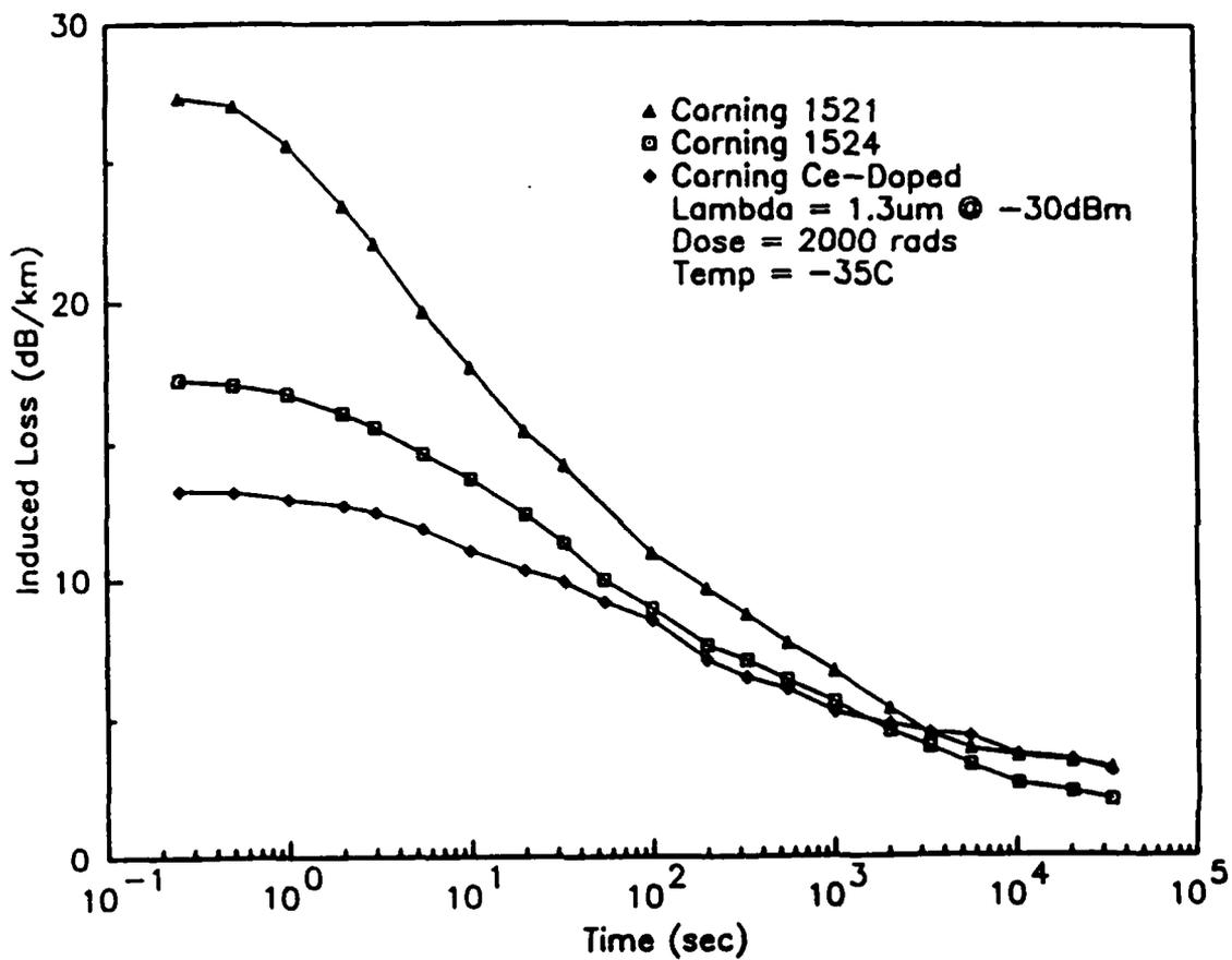
Fig. 7. Recovery data of Corning commercial singlemode fibers. (Frebiele<sup>28</sup>)
