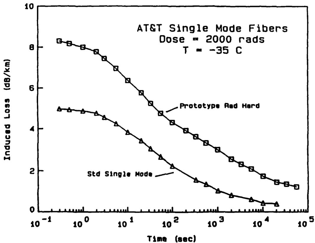
Fig. 8. Recovery data of AT&T standard and rad-hard singlemode fibers. (Frebiele<sup>28</sup>)
