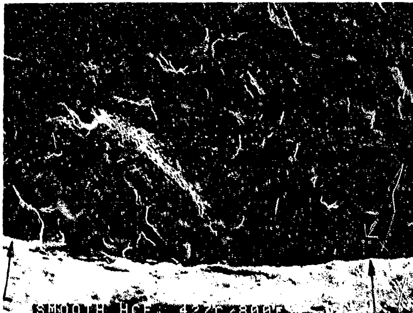
FIGURE 8-48: Higher magnification photograph of the localized origin area. Several stage I fatigue facets are visible at the surface (arrows).
