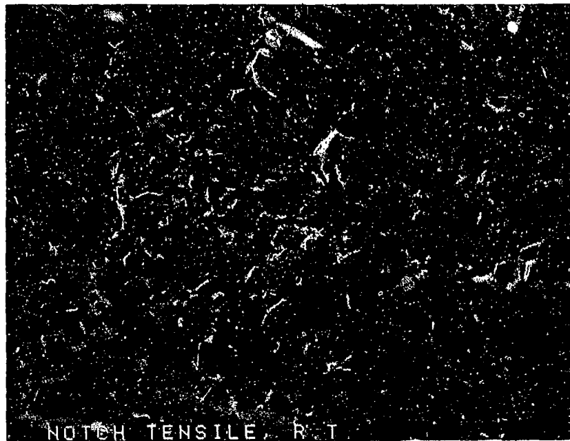
FIGURE 5-17: No shear lip is present in this low magnification photograph.
