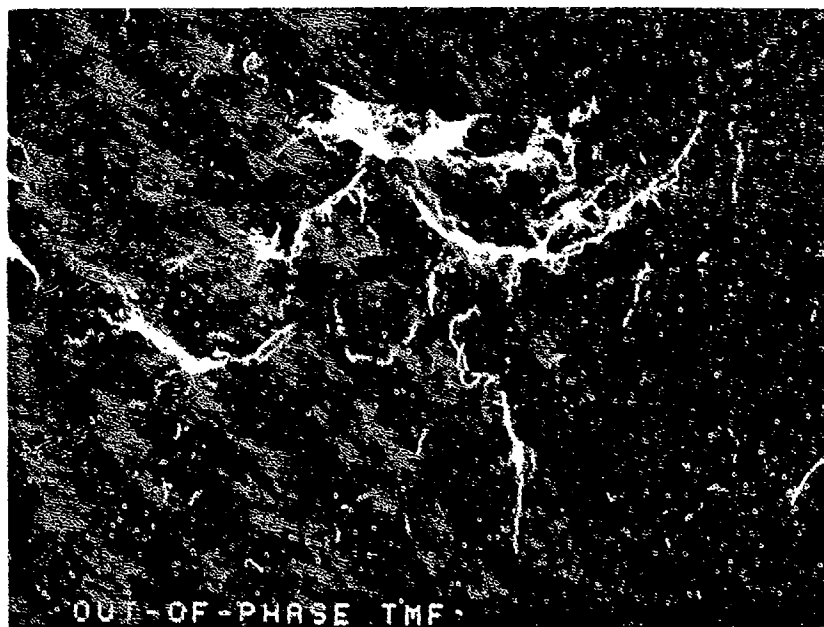
FIGURE 6-30: Oxidized fatigue thumbnail area. The flat oxidized appearance indicates O.D. origins (bottom). No localized origins are discernible.
