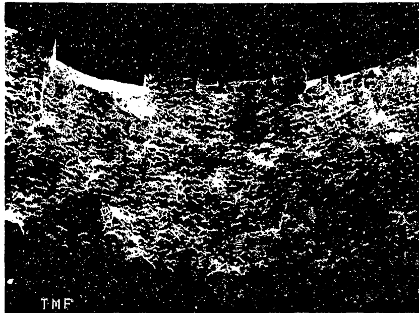
FIGURE 8-121: Overall photograph of the fracture surface showing tensile overstress features with no fatigue present.
