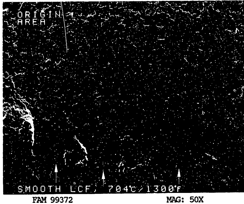
FIGURE 8-111: Overall photograph of the origin area and initial fatigue propagation zone. Several localized origins separated by steps are visible. The origins are indicated by arrows.
