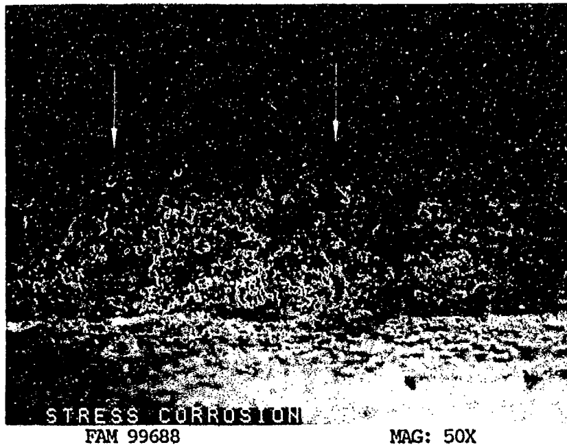
FIGURE 2-3: Low magnification photograph of the fracture surface exhibiting intergranular features. The final overstress area is visible as a thin band at the upper edge of the specimen (arrows).
