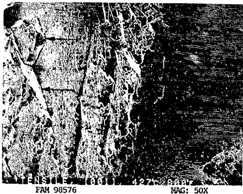
FIGURE 10-4: Higher magnification photograph of the area shown in Figure 10-3, showing abrupt changes in fracture path (arrows) associated with fracture along close-packed planes.
