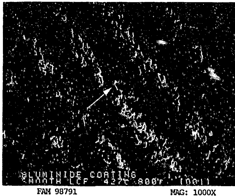
FIGURE 10-38: The fatigue striations consist of lines of smeared features with cleavage in between. The direction of propagation is shown by an arrow.
