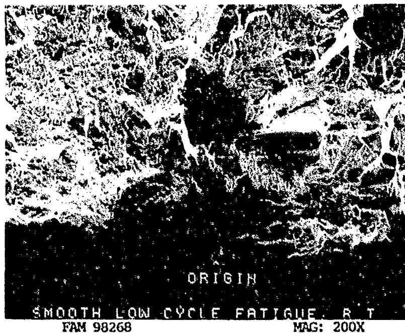
FIGURE 7-40: Fracture origin shown in Figure 7-39, exhibiting smooth cleavage facets (Stage I fatigue).
