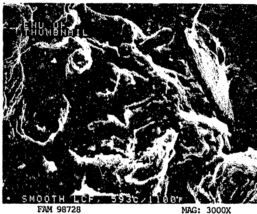
FIGURE 9-113: Higher magnification photograph of the area shown in Figure 9-112, showing remnant fatigue features.
