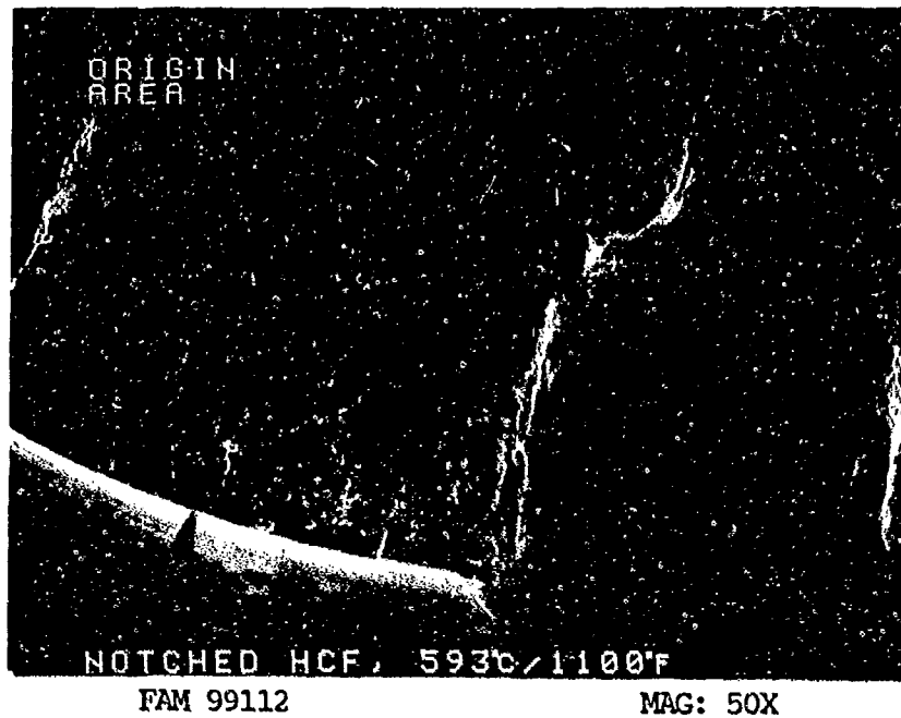
FIGURE 9-88: One of several fatigue origins separated by fatigue steps. Features can be seen radiating from a small localized (point) origin (arrow).
