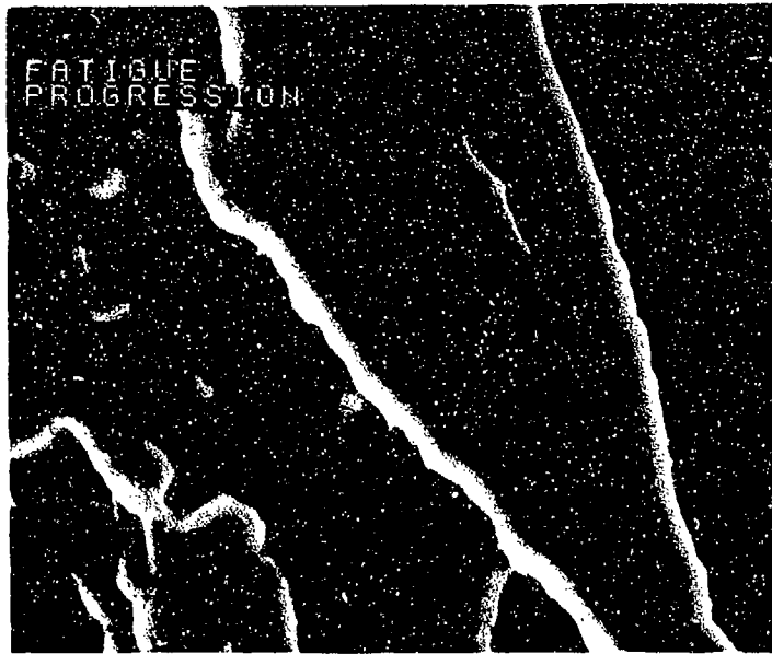
FIGURE III-31: Typical stage II transgranular fatigue progression in an HCF fatigue specimen.
