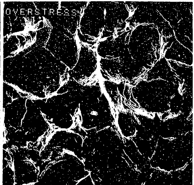
FIGURE III-8: Coarse dimpled overstress.
