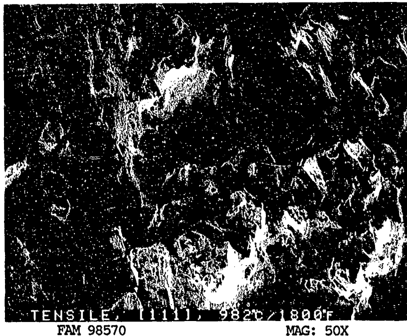
FIGURE 10-23: Oxidized fracture surface with deep jagged appearance resulting from localized cleavage along crystallographic planes. Compare this appearance with the 800°F specimen (Figures 10-16 through 10-19).
