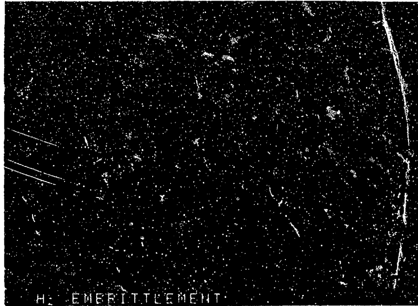
FIGURE 3-69: Low magnification photograph of the fracture surface exhibiting ductile overstress with patches of cleavage.
