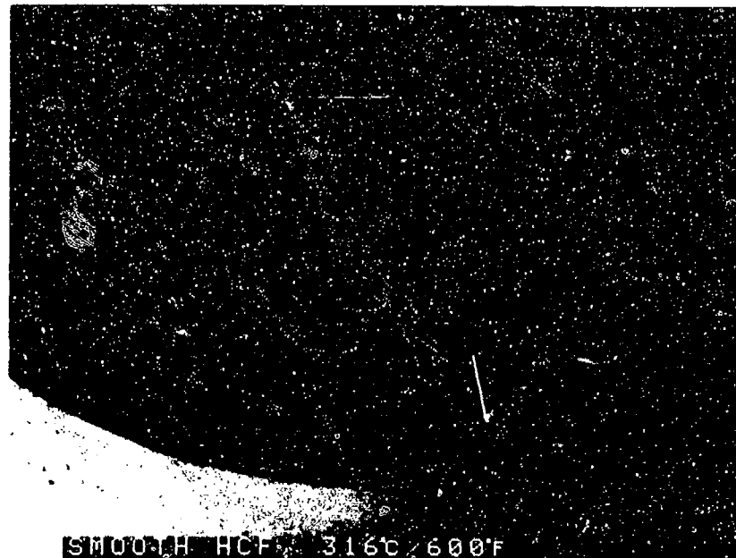
FIGURE 1-26: Low magnification photograph showing fatigue initiation and progression on a plane perpendicular to the stress axis. Features can be seen radiating from a subsurface origin. A small shear lip is visible on either side of the origin.
