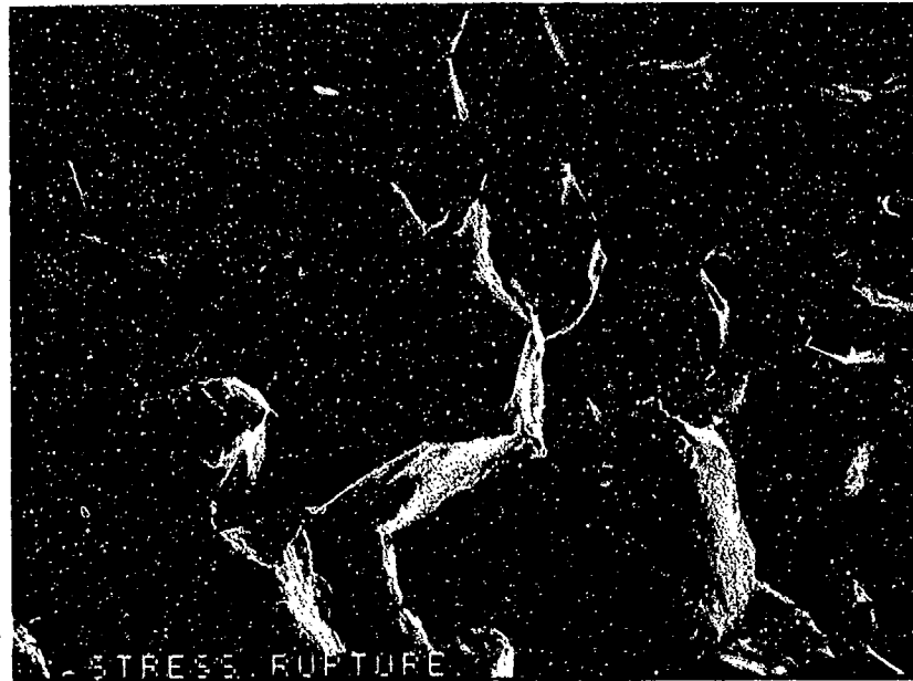
FIGURE 5-31: Intergranular rupture with intergranular secondary cracking.
