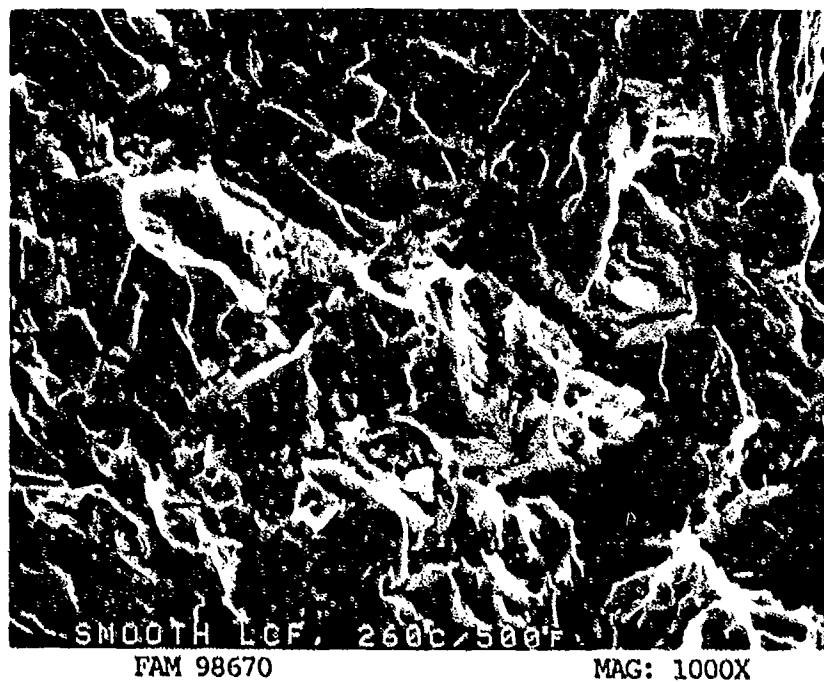
FIGURE 12-95: Remnant fatigue striations in the fatigue thumbnail region. An arrow indicates one patch. The direction of local propagation varies from one patch to another.
