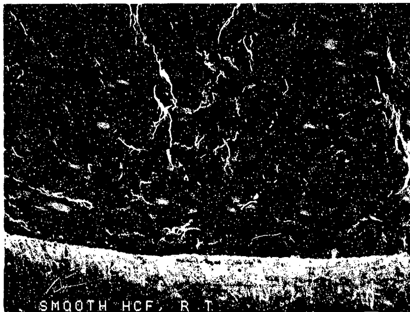
FIGURE 8-38: Higher magnification photograph of the localized origin area exhibiting feathery cleavage.
