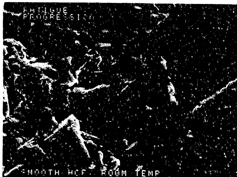
FIGURE 11-31: Higher magnification view of the area shown in Figure 11-30, showing fatigue striations and crack-like striations.
