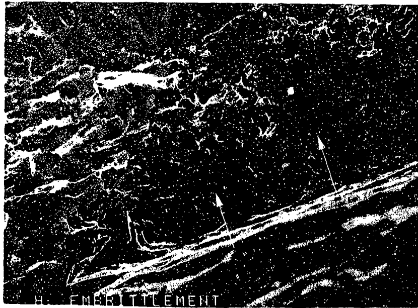
FIGURE 2-11: Possible remnant cleavage features at the edge of the specimen (arrows).
