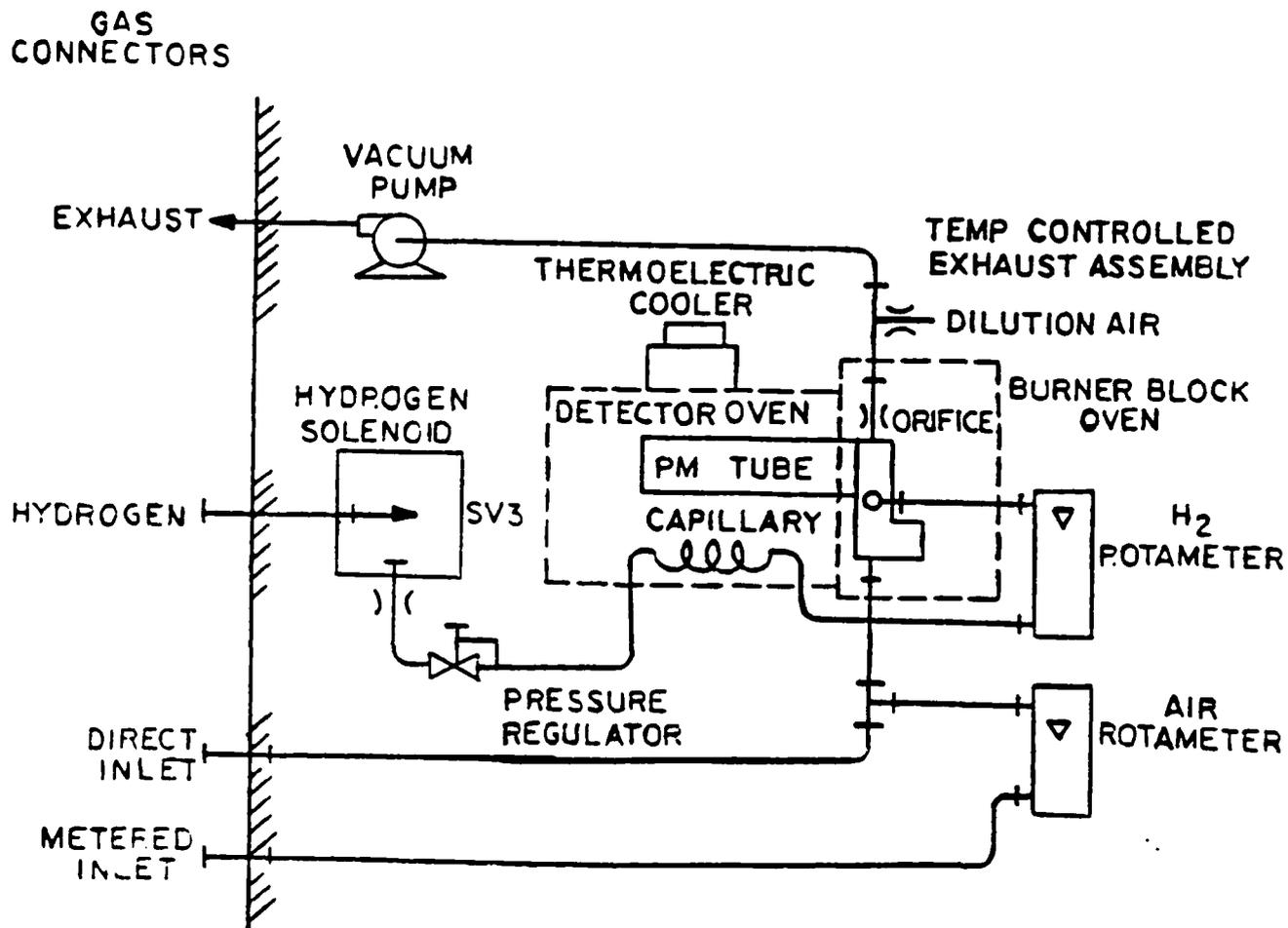
Figure 2. Pneumatic Network of PA260
