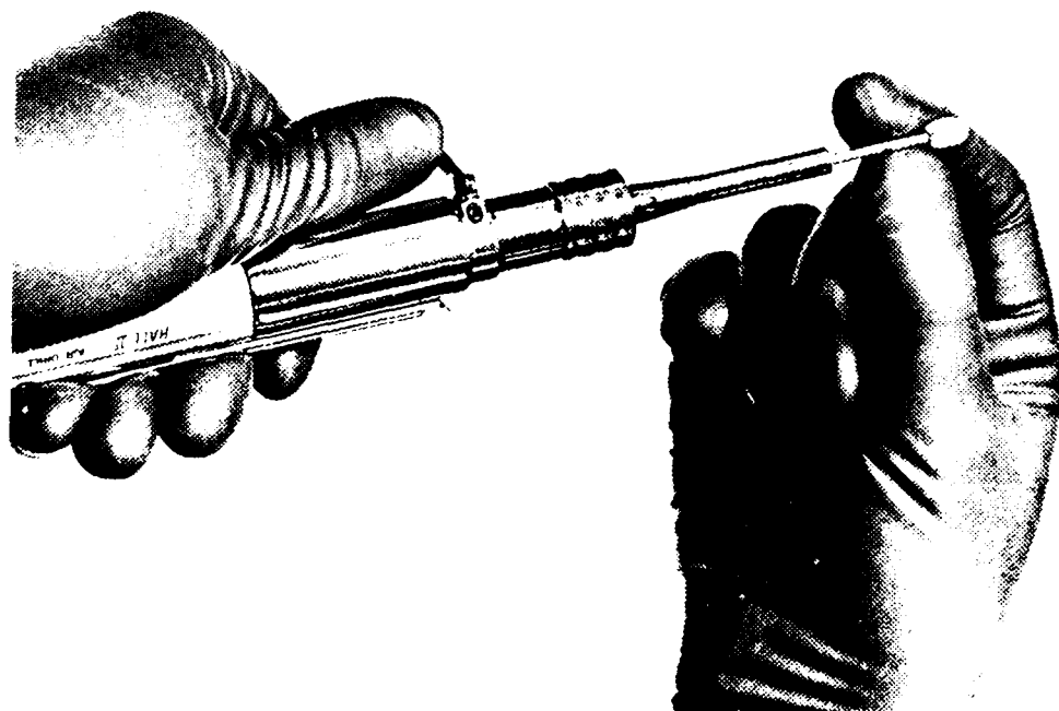
Figure 5-7.—Placing bur guard on air drill.
