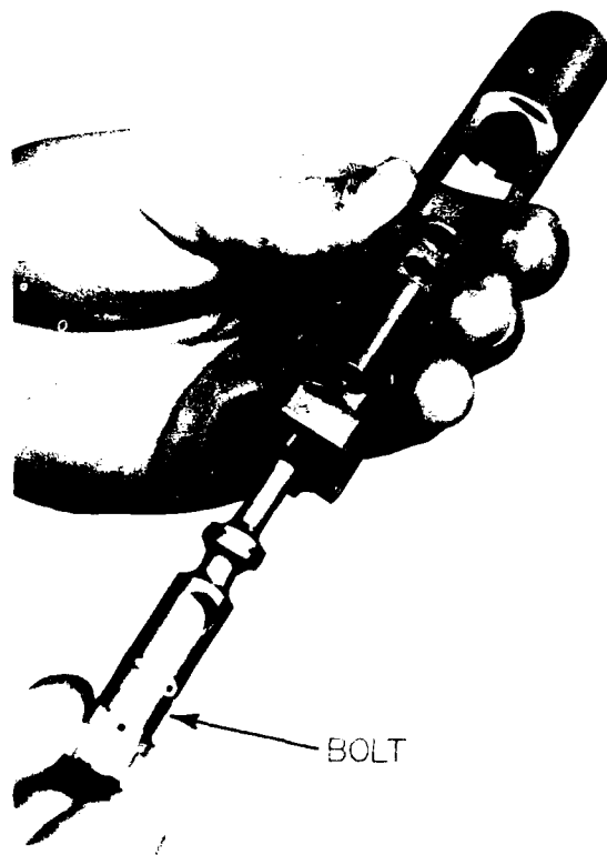
Figure 4-18. --Removing the bolt from the bolt carrier.
