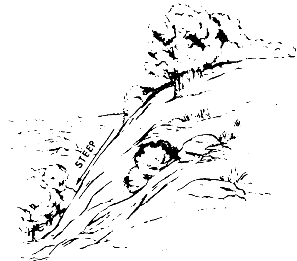
Figure 15-6.—Estimating elevations between contour lines.
