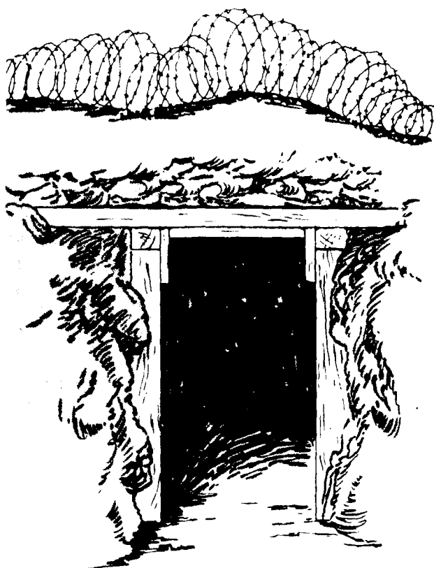
Figure 9-27. —Protective wire on top of overhead cover.
