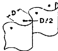
SINE-WAVE BEAM (TANGENT-HALF CIRCLE)
