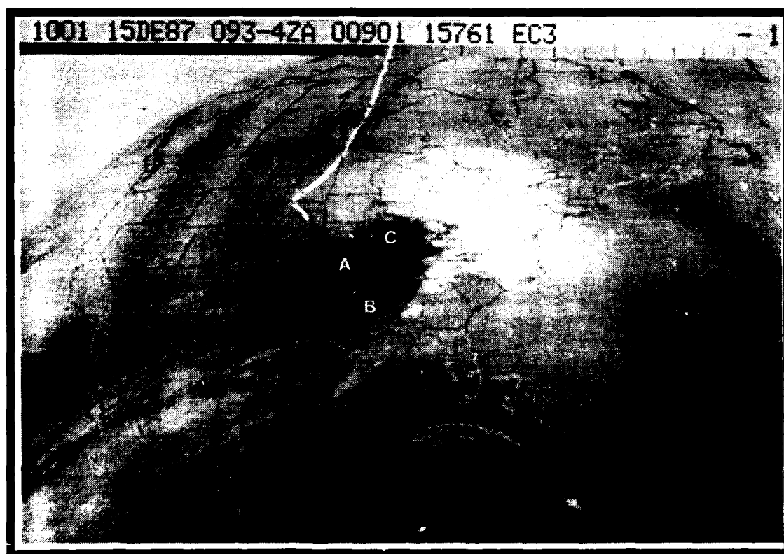
Figure 4.9b. GOES-East 6.7 \mu\text{m} water vapor satellite imagery for 10:00 UTC 15 December 1987. Lettered areas are referenced in the text.
