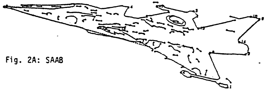
Fig. 2A-2D: Segmented images of 4 aeroplanes. Specific points are denoted by numbers, edge terminators by +, and straight edges approximations by dashed lines.
