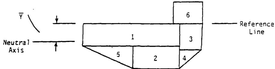
$\bar{Y}$  is the distance from the neutral axis to a reference line.  $\bar{Y}$  can be calculated for simple figures such as rectangles, triangles, and circles. By taking the complex cross-sectional geometry of face A-A and dividing it into sections of rectangles and triangles,  $\bar{Y}$  can be found by the formula:
