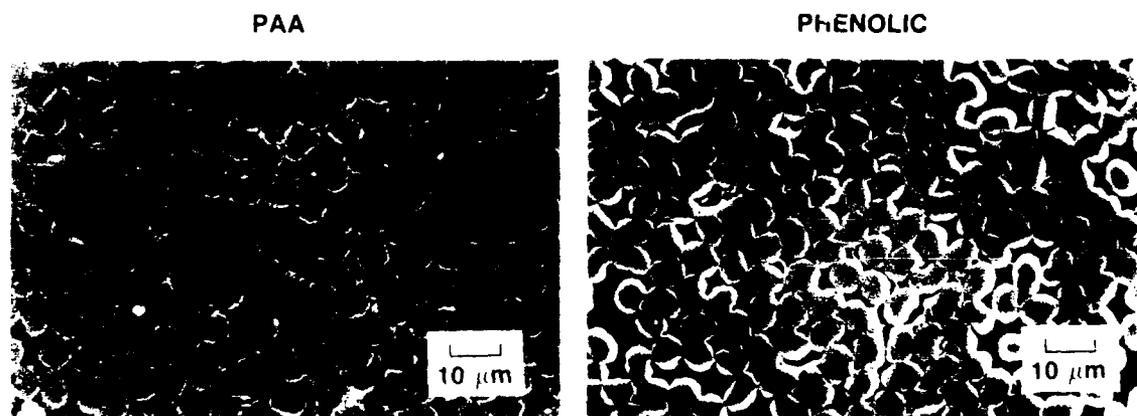
Figure 12. PAA and Phenolic Derived C-C Composites Heat Treated to 1800°C
