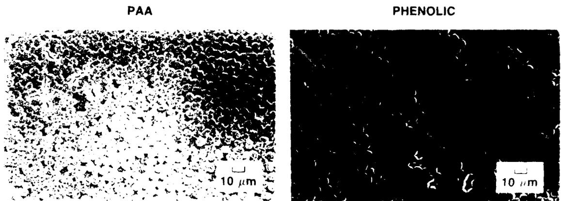
Figure 11. PAA and Phenolic Derived C-C Composites Heat Treated to 1200°C
