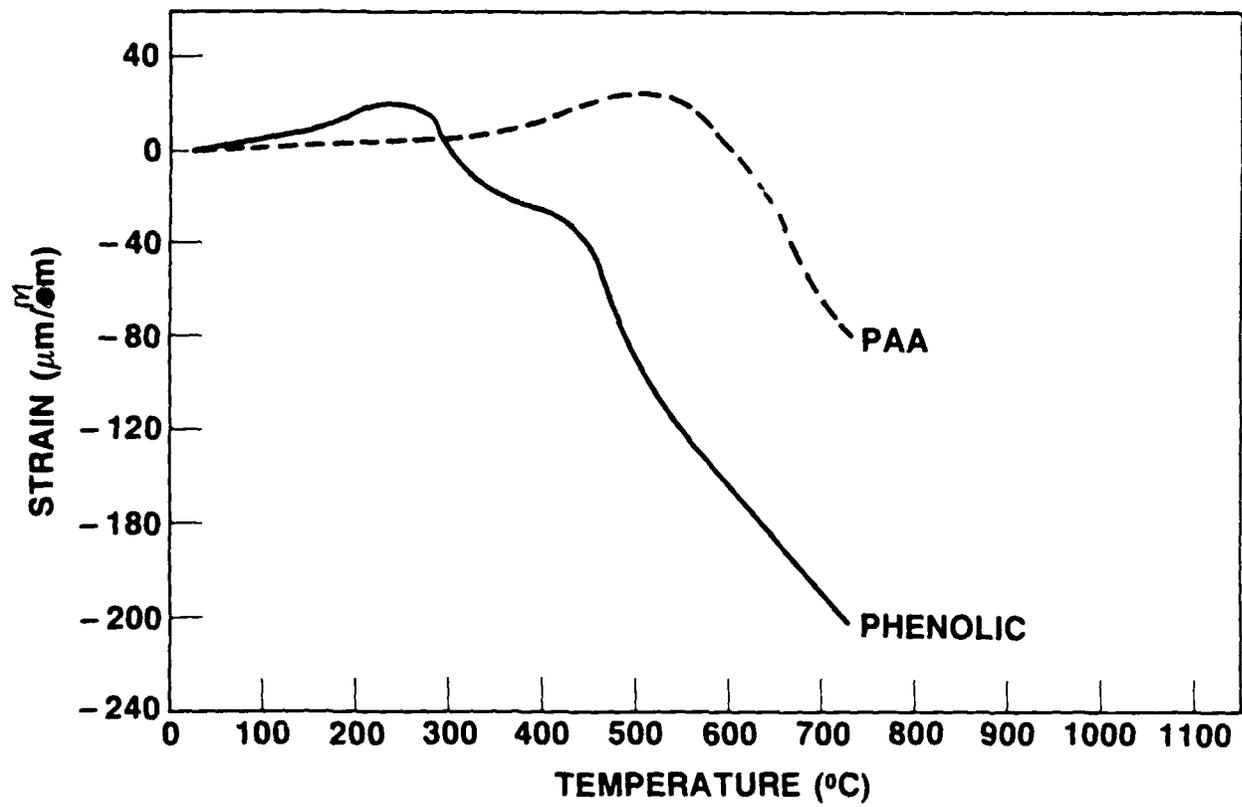
Figure 5. Thermomechanical Analysis of PAA and Phenolic Resins
