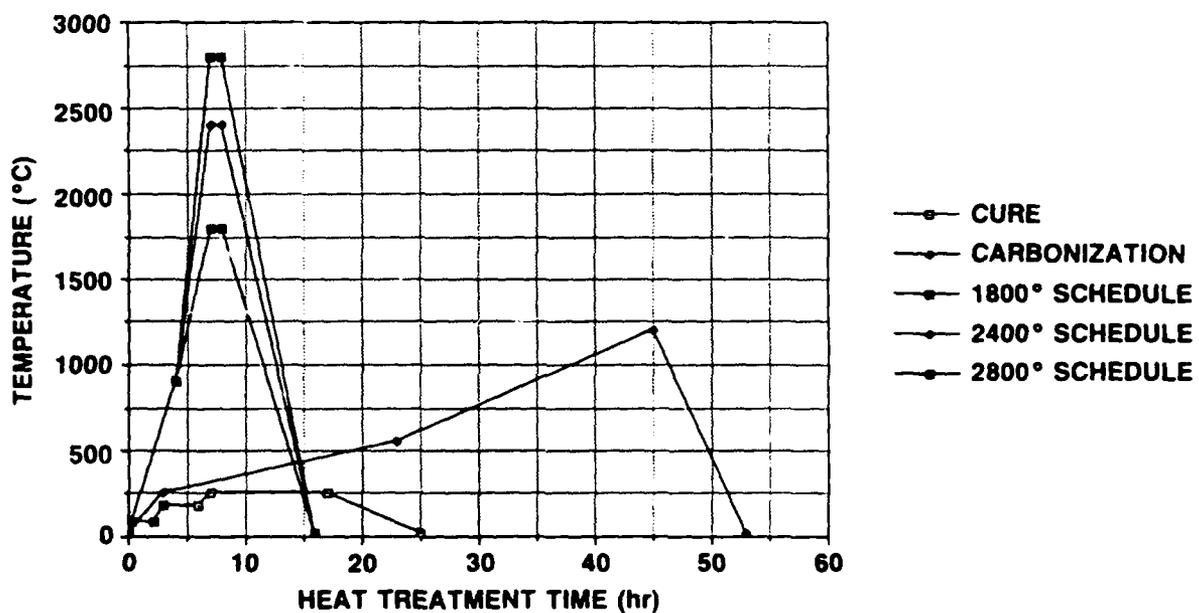
Figure 7. Heat Treatment of PAA/T-50 Composites
