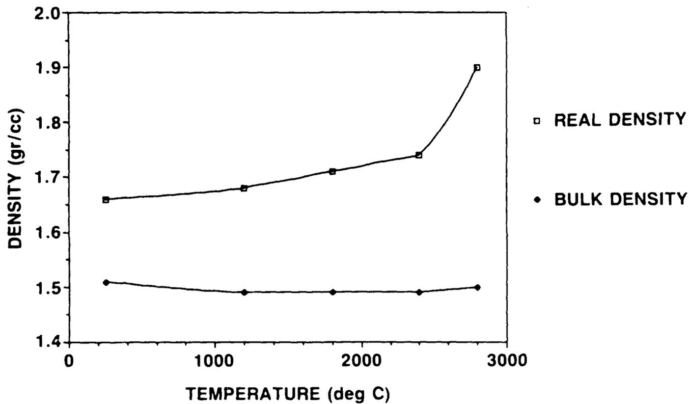
Figure 10. Real and Bulk Densities vs Heat Treatment Temperature for Phenolic/T-50 Composites
