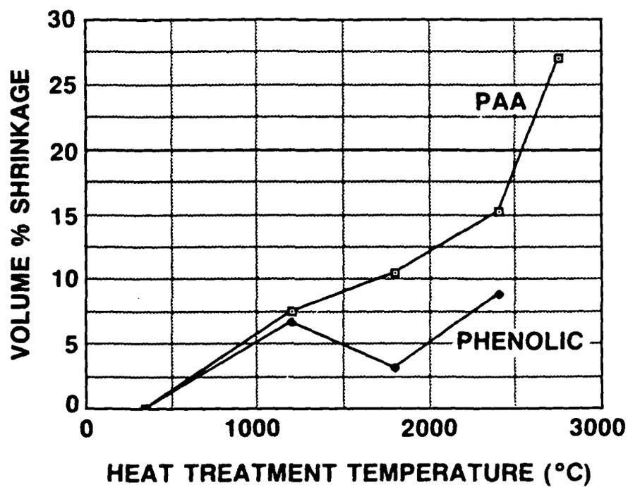
Figure 8. Composite Shrinkage Due To Heat Treatment
