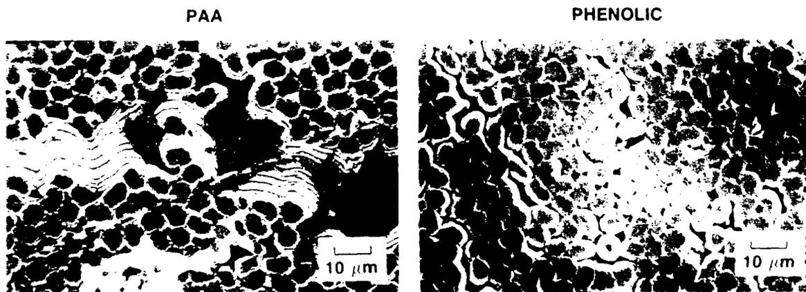
Figure 13. Development of Anisotropic Orientation in PAA and Phenolic C-C Composites Heat Treated to 2400°C
