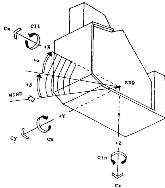
Fig. 5 SHABP input geometry model with aerocoeficients.
