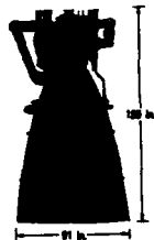
Figure 10. RL10 Liquid Hydrogen Rocket Engine
