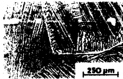
(a) Slow cooled, fully transformed \beta microstructure - IMI685
