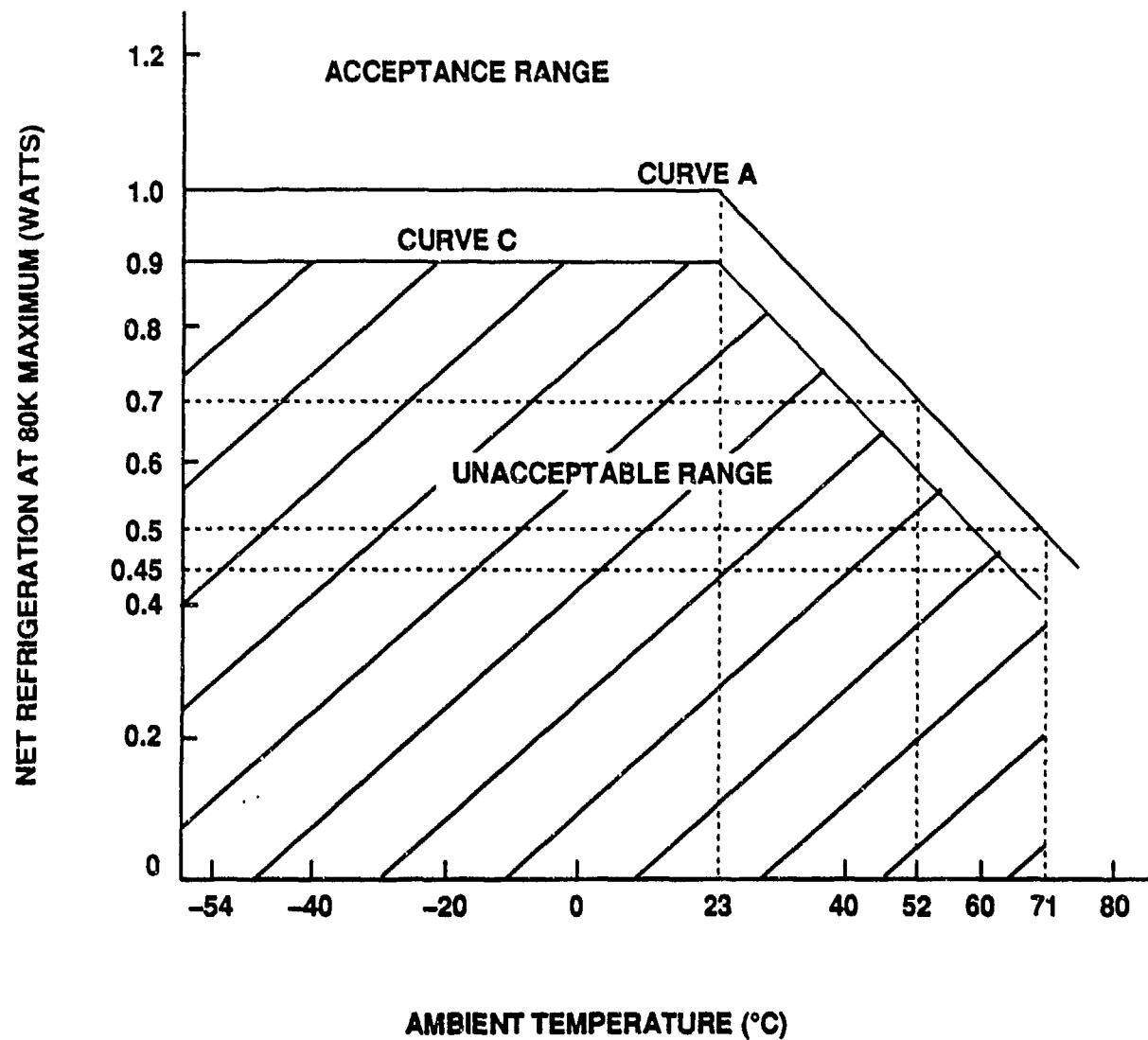
Figure 2. Cooling Capacity
