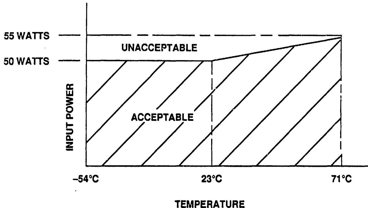
Figure 3. Input Power with Heat Load Applied
