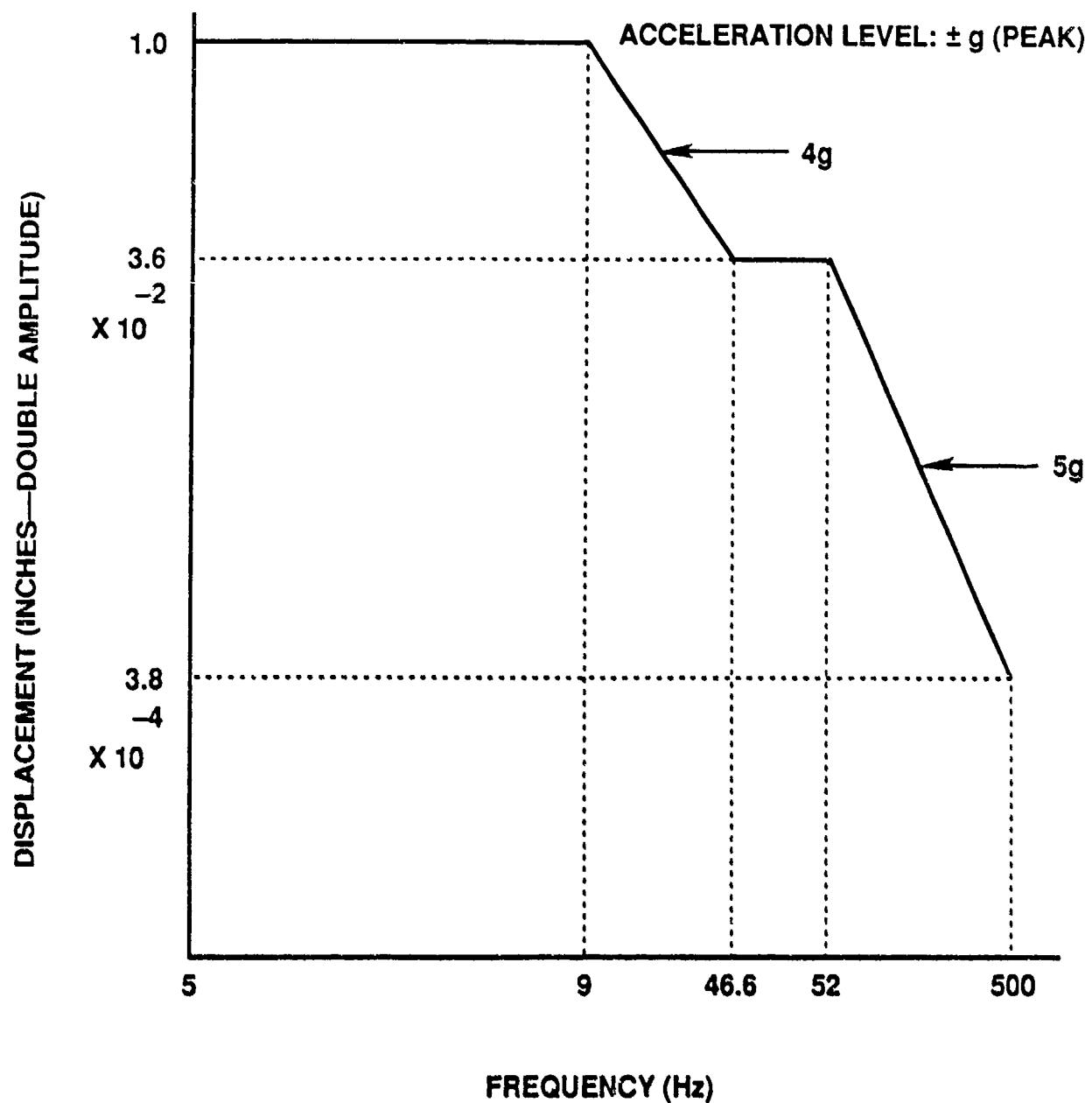
Figure 4. Vibration Test Profile
