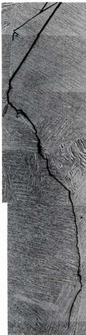
Fig 6 Microstructural influence on crack path in a Ti alloy
