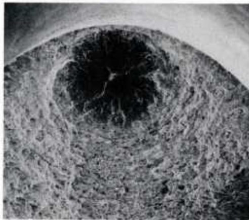
Fig 4 Subsurface failure in powder Ni-base alloy
