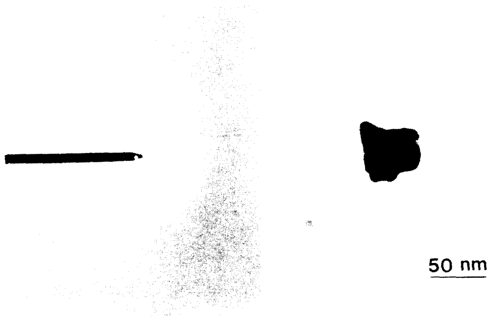
Fig. 3. Morphology of a YBa 2 Cu 3 O 7-x crystallite and its [001] diffraction pattern showing that it is tetragonal
