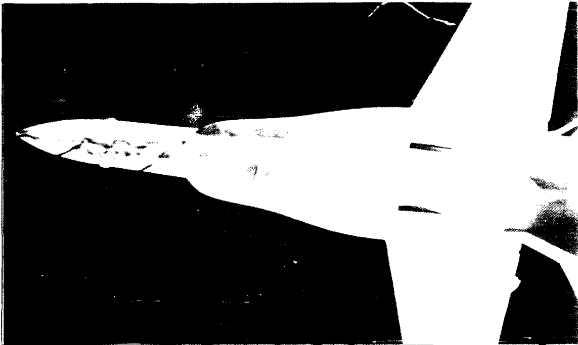
Figure 97. Forebody, High Pitch Down, AOA = 50 deg , YAW = 20 deg.
