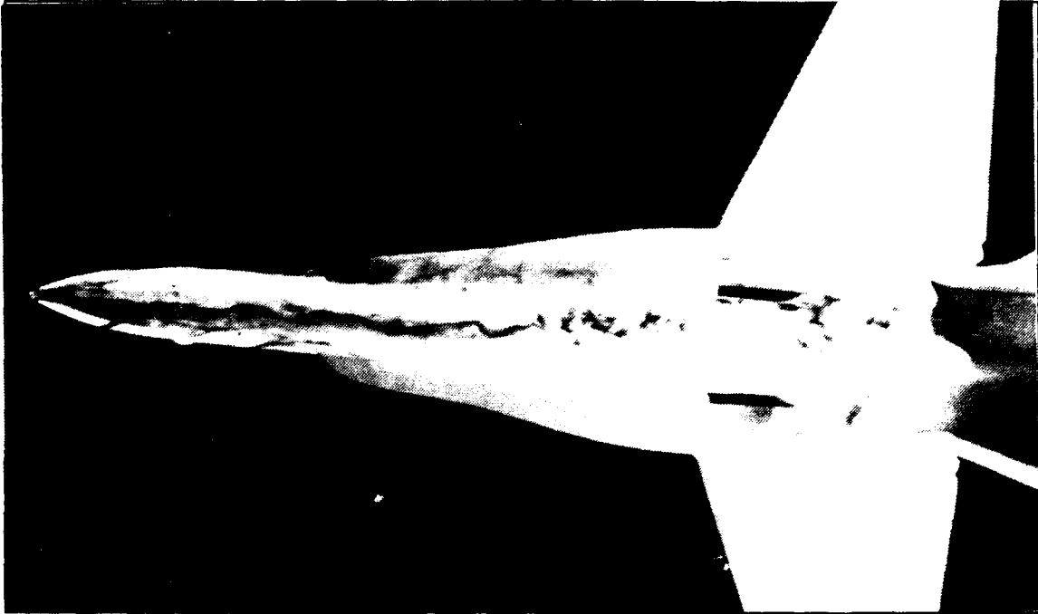
Figure 76. Forebody, High Pitch Up, AOA = 40 deg , YAW = 10 deg.
