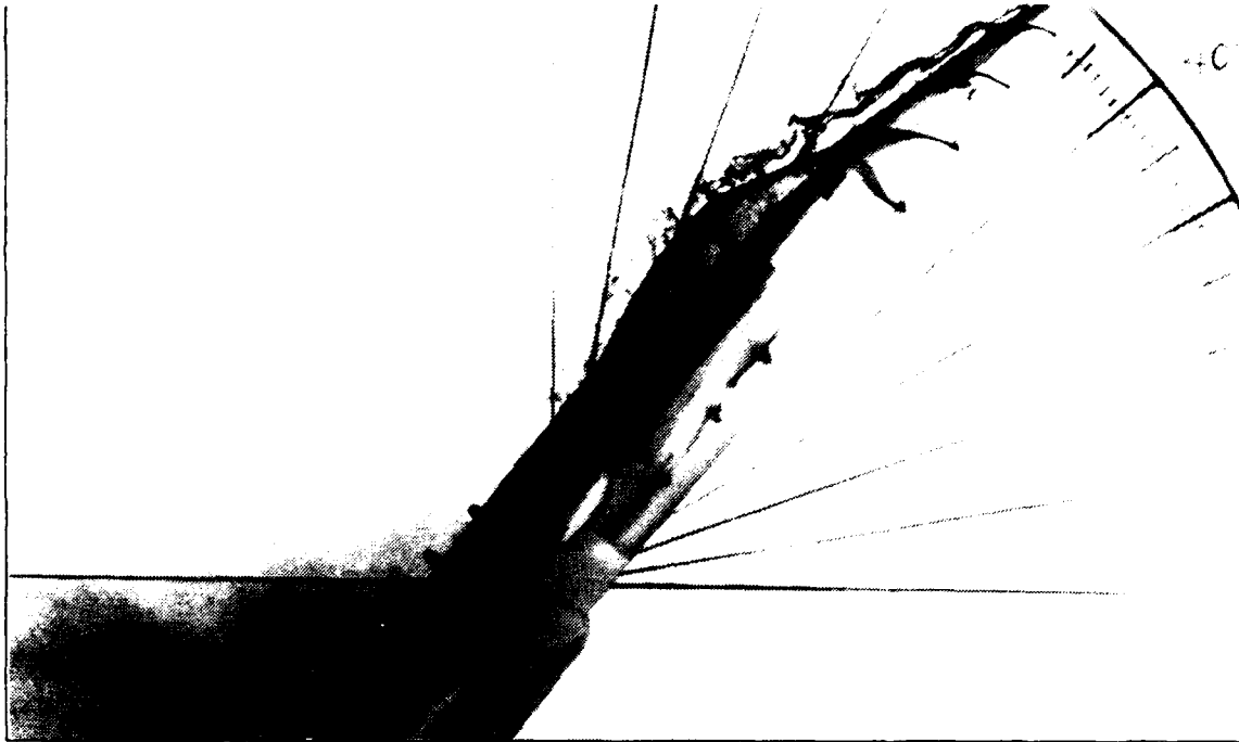
Figure 84. Forebody, High Pitch Up. AOA = 50 deg , YAW = 0 deg.
