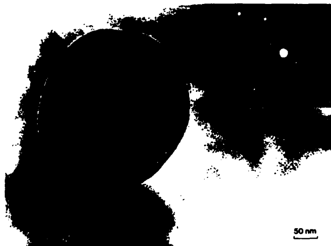
FIG. 10. Transmission electron micrograph of a spherical inclusion of Nd_2O_3 of hexagonal crystal structure embedded in the hard magnetic grain. Such Nd oxides are found with different diameters in the NFB magnet as well as in the Al-doped magnets.
