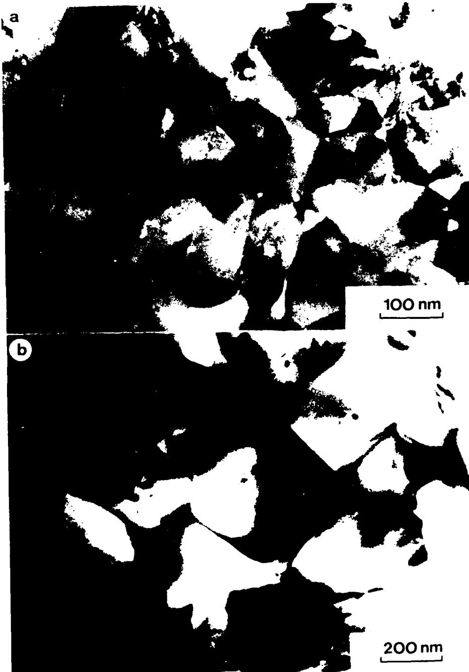
Fig.4: Transmission electron micrographs of a "melt-spun" (a) and a mechanically alloyed (b) Nd-Fe-B magnet.
