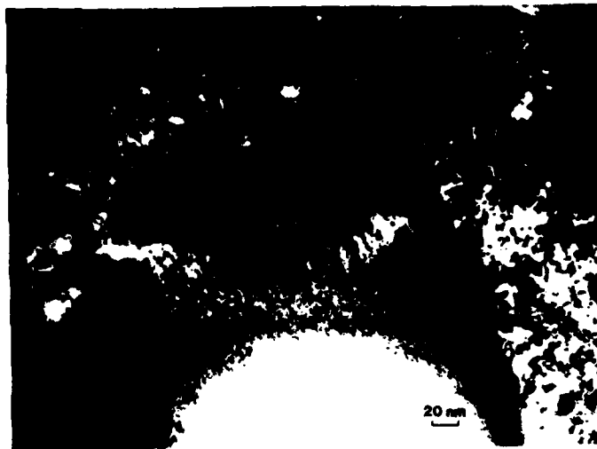
FIG. 4. Transmission electron micrograph of the NFB-Al magnet showing the Nd(Fe, Al) 2 phase (a1), embedded in the Nd-rich intergranular phase n1. The lattice fringe contrast within this phase corresponds to an interplanar spacing of about 1.2 nm.
