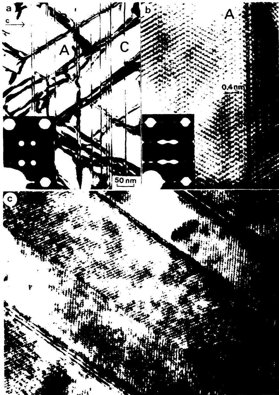
Fig.1: Electron micrographs showing the cellular precipitation structure of a \text{Sm}(\text{Co,Fe,Cu,Zr})_{7.5} magnet.
