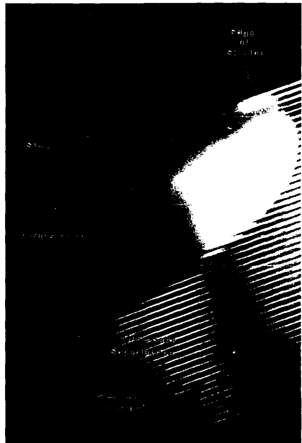
Fig. 1 — Transmission electron micrograph of a GaAs-AlAs superlattice compositionally mixed by diffusion from an Si stripe. The mixed region extends to a depth of 400 nm, while the lateral spread away from the Si stripe is less than 100 nm.
