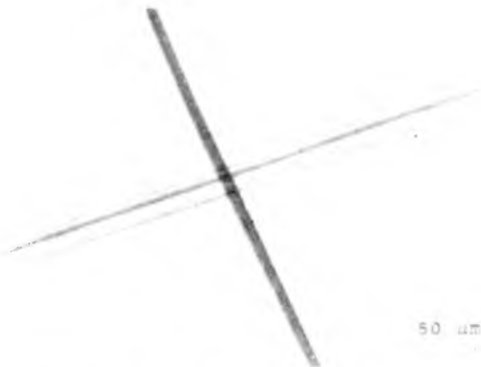
Figure 2. Transmitted light optical photomicrograph of parts of short (100-mm long) Y-Si-Al-O-N glass fibers drawn from a glass rod. Fiber quality and uniformity are good, and the small diameter ( 10\ \mu\text{m} ) of one fiber indicates that fine fibers can be formed from this glass.
