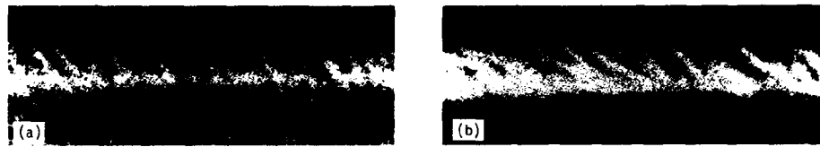
Figure 3. Enlarged schlieren photographs of flow (a) on the floor of the duct and (b) on a flat plate (from Deckker 1980).
