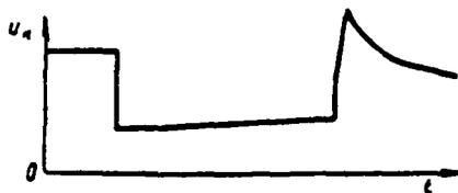
Figure X.55. Resistance  $R_a$  Voltage Curve in the Figure IX.21 GPN Circuit.
