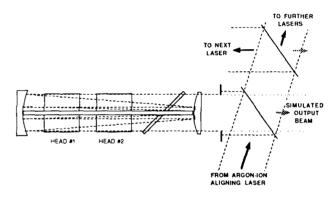
Fig. 5: Alignment with argon-ion laser.
