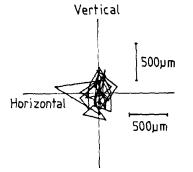
Fig.3a A trace of the peak position of the far field spot at 250Hz pulse rate
