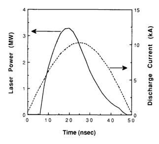
Fig.4 Discharge-current-pulse and calculated laser power output for the peak current of 10 kA.
