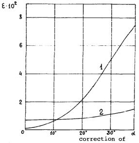
Fig.11 R.m.s. error of defocus (1) and astigmatism (2) by the adaptive mirror with 19 actuators vs the angle between the normal to the mirror surface and the axis of the incident beam. THE ROLE OF PLASMOCHEMICAL REACTIONS IN THE FORMATION OF SPER-LASER ACTIVE MEDIUM
