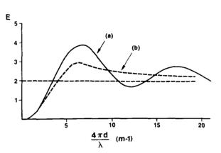
Fig. 3: Variation of the light-extinction coefficient E in a transparent medium containing dispersed spherical particles as a function of the particle mean diameter d and relative refractive index m for (a) a monodisperse and (b) a polydisperse distribution.
