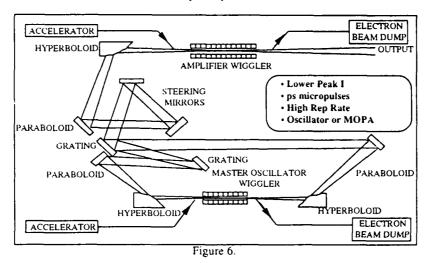
In more recent results, Boeing has upgraded their power conditioning system to provide flat top macropulses more than 100 microseconds long. The peak micropulse current is more than 300 A and the SpectraTechnology permanent magnet wiggler has a maximum field error of less than 0.5%. The system was recently modified to lase at 0.62 micross.
