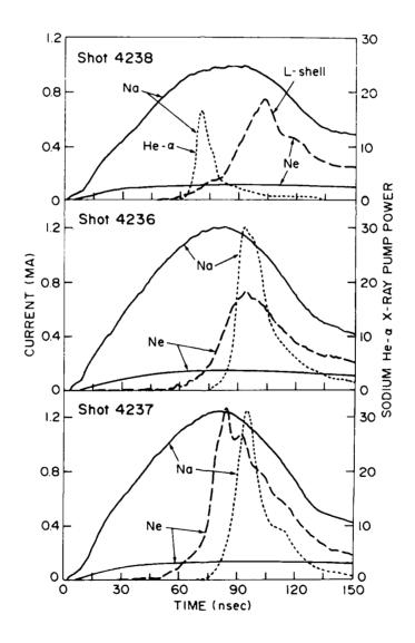
Figure 6. Current and x-ray traces for three shots with both sodium and neon implosions. The solid curves are current traces. The short-dash curves are the sodium He- $\alpha$  x-ray power. The long-dash curves are the neon L-shell x-ray emission.
