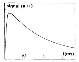
$\underline{Fig. 6}$  - Photothermal signal vs time, after 100 scans, for a mirror of 20 ppm absorption level.
