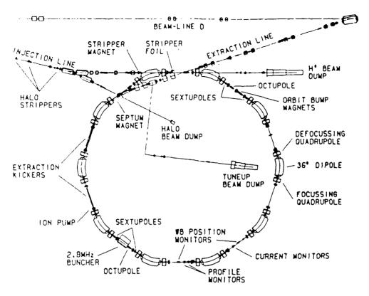
Figure 4: Shematic overview of the PSR facility at LAMPF.
