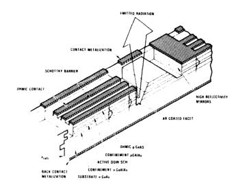
Figure 2- Transverse and Lateral Device Geometry
