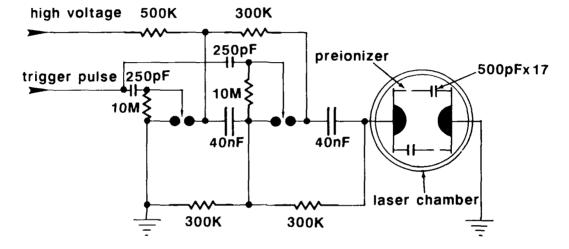
Fig. 1. Electrical circuit diagram of the XeCl laser.
