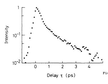
Fig. 2: Semi-logarithmic plots of the delay time dependence of signal intensity obtained from CS<sub>2</sub>
