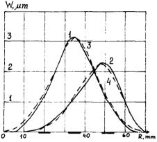
Fig.3A Adaptive mirror influence function profiles obtained experimentally (1,2) and drive voltage on central  $(\bullet)$  from the theory of thin plate and peripherial  $(\blacktriangle)$  actuator. (3,4).
