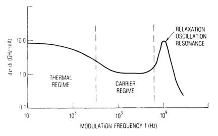
Figure 3. Typical AlGaAs modulation depth vs modulation frequency curve.
