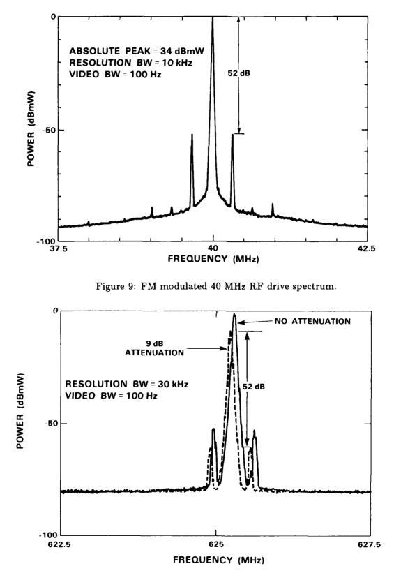
Figure 10: Heterodyne spectrum with FM modulation of the 40 MHz RF drive signal and attenuation of the isotope reference laser.
