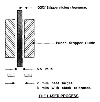
To cut the one ounce cold rolled (2.8 mil thick) copper dambar a Q-switched YAG laser beam is used.
