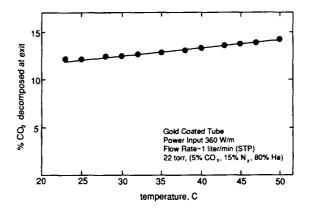
Figure 6: Effect of cooling water temperature on the measured CO2 decomposition in Laser A. The catalytic effect decreases with increasing temperature.
