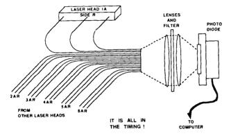
Fig. 7: Fiber optic multiplexing for monitoring flash-lamp performance.
