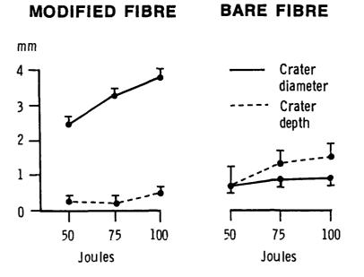
Fig. 9 - Diameter, size and depth of the craters shown in Fig. 8
