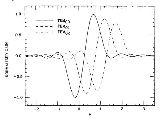
Figure 6. Laser gain normalized to the  $TEM_{00}$  mode for the first three Gauss-Laguerre modes of a FEL with cylindrical symmetry. The parameter v is the frequency or energy detuning. Larger values of v correspond to longer wavelengths.
