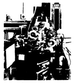
Fig. 9 Flashlamp Pumped Dye Laser Built at ARL Which Implements a Three-Channel Slab Design
