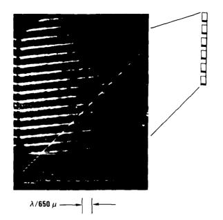
Figure 8- Far-Field Interference Pattern for a 1x6 Row of Unit Cells
