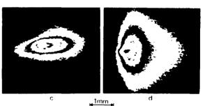
Fig. 7: Image obtained with an apparatus of the kind shown in Fig. 6 for PP/PC ribbons drawn with an HSR equal to 5 (pictures a and b) and 1 (c and d). The He-Ne laser beam was incident from the left at 45° from the normal, and the fibrillar particles in the ribbons were oriented either in the vertical (a and c) or in the horizontal (b and d) directions.
