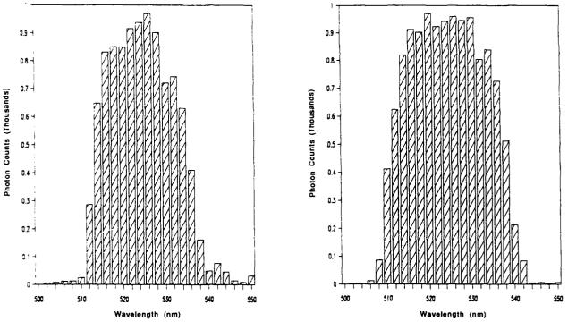
Fig. 2. Lasing characteristics of 5.6 mM dye 1 in dimethylformamide.
