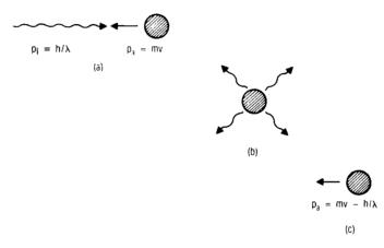
Figure 4. Laser cooling. (a) photon absorption, (b) photon emission, (c) average velocity reduction.
