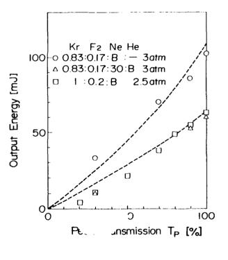
Fig. 7 Output energy v.s. peak transmission
