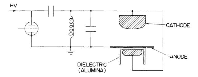
Fig. 1 Electrical Circuit and Discharge Electrodes.
