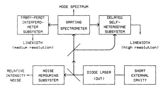
Fig. 1 Scheme of experimental set-up
