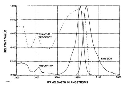
Fig. 10 Spectral Data for RH590 in 50% MeOH/50%  $\rm H_2O.$  Detailed Spectra Are Stored on Disk for the Computer Simulation Codes
