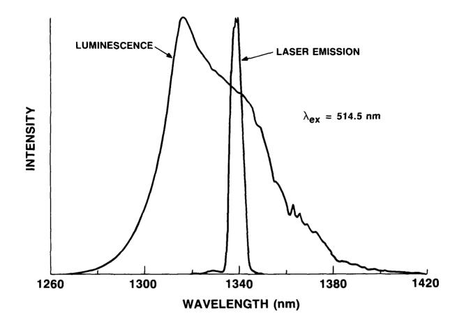
Figure 2. Spectral output of untuned Nd<sup>3+</sup> ZBLAN fiber laser below threshold showing broad spontaneous emission and above threshold showing bimodal stimulated emission at 1.33 and 1.34 micron.
