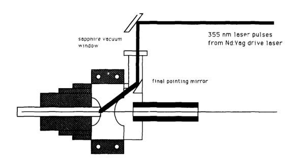
Figure #2 Illustration of the final pointing mirror and the microwave gun
