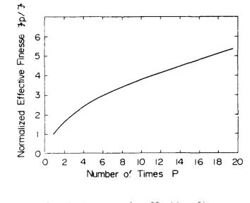
Fig. 6 Increase in effective finesse v.s. number of times passing through etalon.
