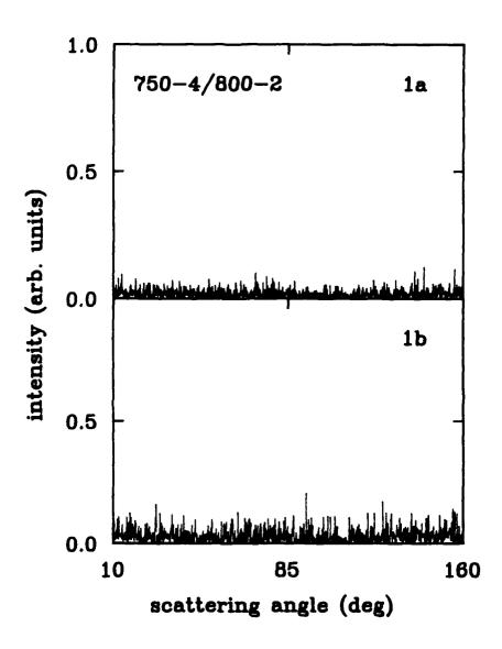
Fig. 1. Angular scattering spectra measured for mullite glass-ceramic sample (750-4/800-2) with 0.1 mm pinhole size: (1a) the horizontal component, (1b) the vertical component.
