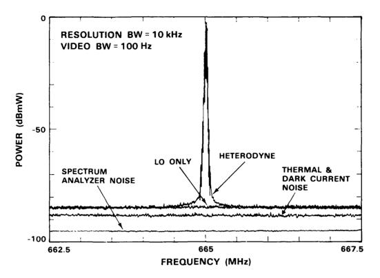
Figure 5: Heterodyne spectrum with an unmodulated LO laser.
