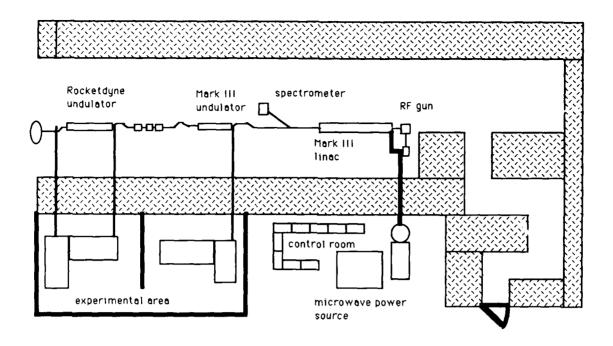
Figure #4 Layout of the SPRL FEL facility.
