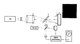
Fig. 13: Apparatus for laser generation and detection of convergent SAW's with a negative axicon. a: axicon, d: dichroic mirror.
