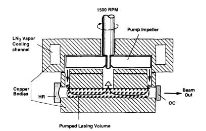
Figure 1. A schematic of the laser cell, which was 2 cm long. The entire assembly was enclosed in an evacuated chamber for thermal isolation. The normal operating conditions were 104 K and 2.8 atm. In this view the e-beam entered from the back; the foil is shown as the checked area behind the lasing volume.
