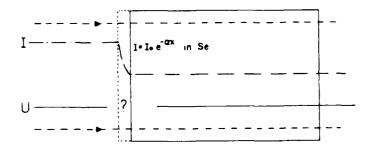
The resolution of the heat diffusion differential equation with Newton's law of continuity at the interfaces (see equations 1) has been acheived using the Green's functions method<sup>6</sup>.
