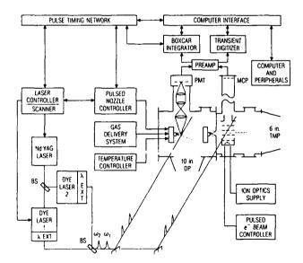
Fig 1. Schematic of the experimental apparatus. In the present work, 2-C excitation was achieved using a single dye laser and the 2nd, 3rd, or 4th harmonic of the Nd:YAG laser. Symbols are defined as follows: MCP = microchannel plate detector; PMT = photomultiplier tube; TMP = turbomolecular pump; DP = diffusion pump; BS = beamsplitter;  $\lambda$  EXT = wavelength extension components. Free jet fluorescence detection was not used in the present study.
