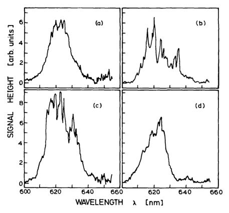
Fig.7: Spectral distributions of 0.01 molar rhodamine B in HFIP. Cell lengths  $\ell = 2$  cm. Pump pulse peak intensities  $I_{OL} \approx 1.5 \times 10^{11}$  W/cm<sup>2</sup>. (a) TPI-ASE. (b) TPI-SPA. (c) amplified ASE signal. (d) amplified SPA-signal.
