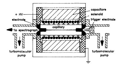
Figure I- Schematic diagram of the capillary discahrge
