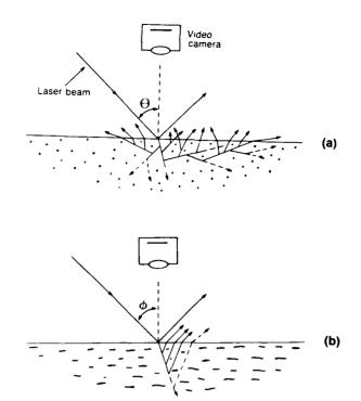
Fig. 6: Schematic diagram of light beam scattering within an oriented material for a beam incident (a) in the plane perpendicular to the fiber orientation, or (b) in a plane parallel to the fiber orientation.
