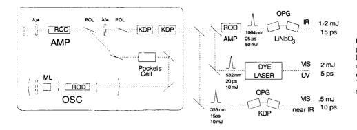
Fig. 2. Schematic for generating 3pulse sequence, using a pulsed modelocked (ML) Nd:YAG laser, shortcavity dye laser, and optical parametric generation (OPG) devices. Typical pulse energies and durations are indicated.
