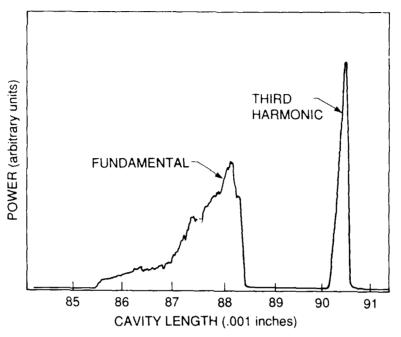
Figure 4. Laser power vs. oscillator cavity length in thousandths of an inch. A larger value for the length indicates a longer cavity. The power is not to scale. Different filters were used for the third harmonic power and fundamental power. The actual maximum powers are listed in table II.
