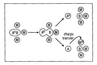
Fig. 5. Pictorial view of the process of dissociation and electron (or charge) transfer in microsolvated molecular clusters.  $AB^+$  represents the aniline cation dissociating to C<sub>5</sub>H<sub>6</sub> (A) and HNC (B). The solvent molecules M are shown preferentially bonded to B as determined experimentally.
