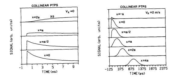
Fig. 2: Computed PTPS signals with pulsed excitation for a (a) stationary medium, and (b) for a medium flowing with a velocity of 2 m/s.
