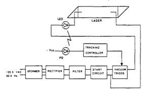
Fig. 5. Power Supply with Wideband Regulation.
