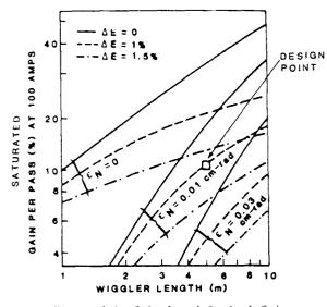
Figure 2.1 Calculated Optical Gain
