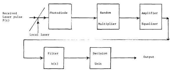
Figure 1. Laser receiver model
