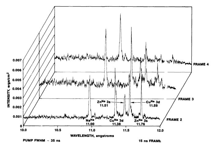
Figure 7. Time Resolved X-ray Crystal Spectra
