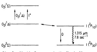
Fig. 2. Kinetic Processes in the Chemically-Pumped Oxygen-Iodine Laser (COIL).
