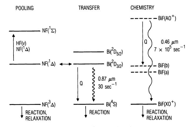
Fig. 3. Kinetic Processes in the NF<sup>\*</sup>-Pumped Bi<sup>\*</sup>, BiF<sup>\*</sup> Laser Candidate System.
