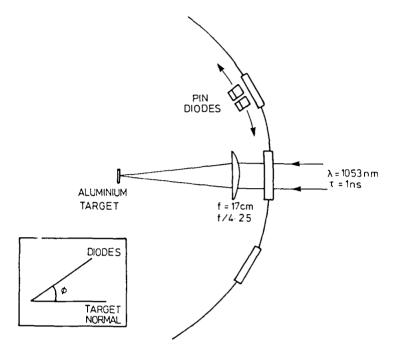
Fig.4 Experimental Arrangement for Source Distribution Measurement
