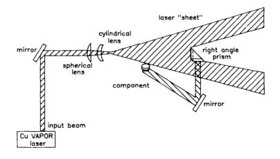
Figure 1 - Optics for high speed filming of components.
