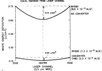
Fig. 12 Calculated Waste Heat Deposition across Laser Channel with and without Converter Dye. Dye Concentrations Have Been Adjusted for Equal Emission from the Laser Channel
