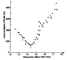
Figure 5. Variation of Autocorrelation FWHM with intracavity glass path.
