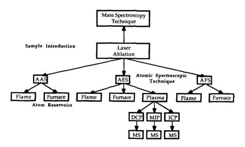
Figure 1. Atomic and mass spectroscopic techniques used with laser vaporization for sample introduction.
