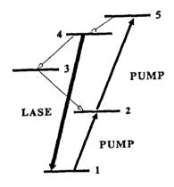
Fig.6 - Cavity lasing field which builds up for five level system discussed earlier (see Figs. 1 and 2)
