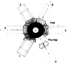
Fig. 6. Top view of the SKUA burst assembly.
