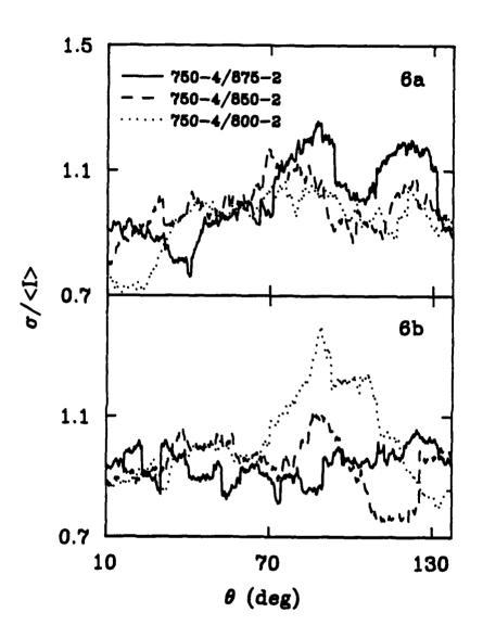
Fig. 6. Angular spectra of the ratio of intensity standard deviation and mean scattered intensity (speckle contrast) calculated for scattering spectra on Fig. 1, 2 and 3 for three mullite glass-ceramic samples: (6a) the horizontal component, (6b) the vertical component.
