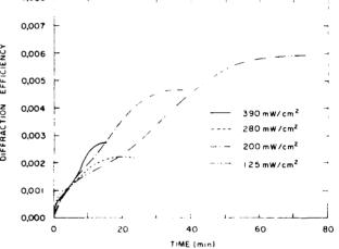
Figure 10. Diffraction efficiency vs time, in Seg1Geg thin films for various writing beams intensities.
