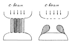
Fig.4 Pattern of a discharge glow in atmospheric pressure nitrogen at 1st and 20th microsecond  $j = 70 \text{ A/cm}^2$ , = 45 ns.
