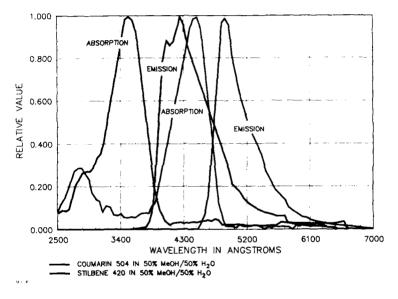
Fig. 3 Spectral Matching of Converter and Laser Dyes
