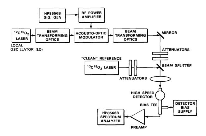
Figure 4: Experimental noise measurement setup.
