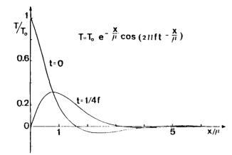
Fig. 1 - Thermal wave : spatial distribution of the periodic temperature at two different times, for a planar heat source T<sub>0</sub> cos2nft located at x = 0.
