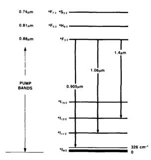
Fig. 1 Low lying energy levels of trivalent neodymium and the laser emissions in silicate glasses.
