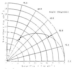
Fig.5 Angular Distribution from an Aluminium Plasma
