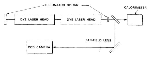
Figure 2. Schematic diagram of the arrangement used to measure the laser's far-field energy distribution.
