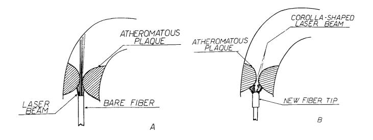
b) Special fiber tip radiating sideways a "corolla" shaped beam with no risk of perforation.
