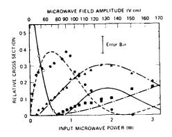
Figure 6 - Observed and calculated values of the cross section for zero photon (resonant) collisions ( $\bigcirc, ---$ ) one photon assisted collisions ( $\bigcirc, ---$ ), two photon assisted collisions ( $\triangle, ---$ ), and three photon assisted collisions ( $\square, ---$ ).
