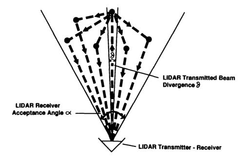
Fig.3. Reduction of received multiple backscatter by decreasing the receiver acceptance angle
