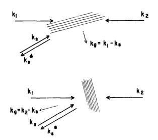
Fig. 2 Degenerate four wave mixing, (top)  $k_1$  interferes with  $k_s$  to form the grating, (bottom)  $k_2$  interferes with  $k_s$  to form the grating.
