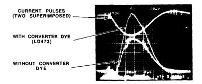
Fig. 1] Neasured Laser Output for the Multichannel Slab Device with and without Converter Dye TOTAL LAMP FLUENCE = 1 J/cm<sup>2</sup> EQUAL EMISSION FROM LASER CHANNEL
