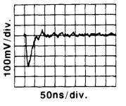
Fig. 2. A typical pulse shape of the XeCl laser output.
