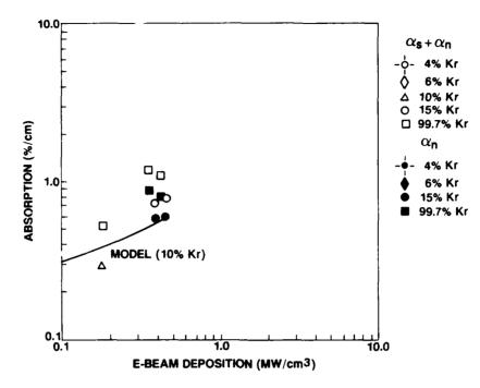
Fig. 3. Absorption data as a function of the e-beam deposition. The solid curve is the prediction from the LANL model for a 10% Kr mixture.
