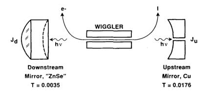
Figure 3. Schematic drawing of resonator configuration.
