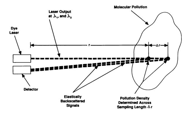
Fig.1. The Differential Absorption Lidar (DIAL) scheme.
