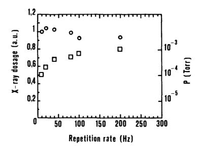
Fig. 10 - X-ray dosage ( $\circ$ ) and vacuum level in the diode chamber ( $\Box$ ) vs the repetition rate. The pressure values were measured after a few seconds of working, when the equilibrium condition was reached
