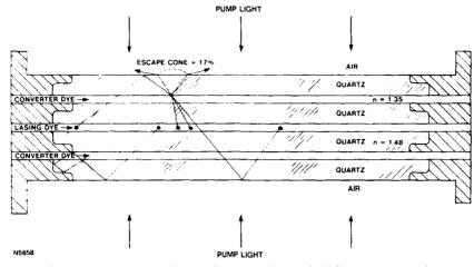
Fig. 8 Slab Configuration Showing Multiple Dye Channels
