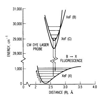
Figure 1. Partial Potential Energy Diagram of the XeF Molecule.
