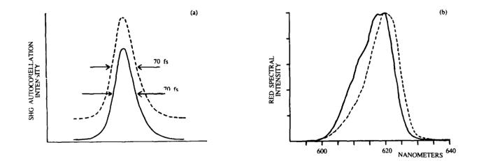
Fig.4. (a) Autocorrelation trace and, (b), spectral profile, with (solid lines) and without (dashed lines) the intracavity frequency doubling crystal.
