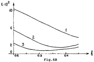
Fig.6A Fig.6A Fig.6 R.m.s. error of defocus (A) and spherical aberration (B) correction by the adaptive mirror with 19 actuators vs the distance between actuators: 1-A=Rm; 2-A=0.8Rm; 3-A=0.6Rm 6 10 A
