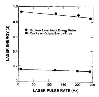
Fig. 1. Dye laser input and output.
