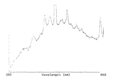
Figure 5 - Laser interaction emission spectrum of TATB.
