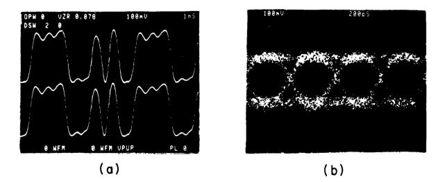
Figure 5 - Signal amplification experiment at 2 Gbit/s in an Er-doped fiber amplifier: (a) oscilloscope traces showing input and output ASK bit sequence (Hor. scale: lns/div); (b) eye diagram of output signal (Hor. scale 200 ps/div, arbitrary vertical scales). The pump wavelength was 514.5 nm and the gain +15 dB (after ref. [25]).
