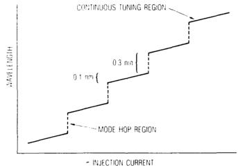
Figure 2. Illustrative diode laser tuning curve.
