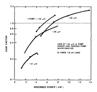
Fig. 9 Gain at 1.55  $\mu$ m versus pump power at various wavelengths for 118 cm long Er fiber laser with 3x10<sup>19</sup> ions/cc in SiO<sub>2</sub> with 3.7 wt % Al<sub>2</sub>O<sub>3</sub>.
