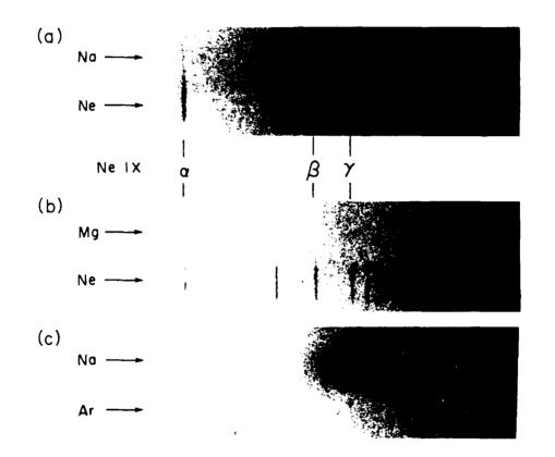
Figure 7. Film record of neon K-shell x-ray spectra (a) for shot 4236 in Figure 6, (b) for a shot with  $MgF_2$  in place of NaF, and (3) for a shot with argon in place of neon. The locations of the a-, 2-, and  $\gamma$ -lines of heliumlike neon are identified.
