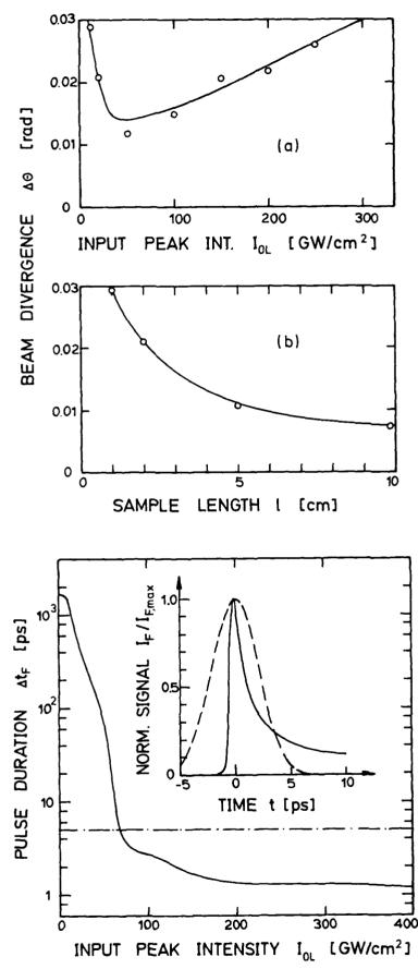
Fig.8: Beam divergence &0 of TPI-ASE signal versus (a) pump pulse peak intensity I<sub>0L</sub> (l = 2 cm) and (b) sample length l (I<sub>0L</sub>  $\approx 1.5 \times 10^{11}$  W/cm<sup>2</sup>). Dye: 0.01 molar rhodamine B in HFIP.
