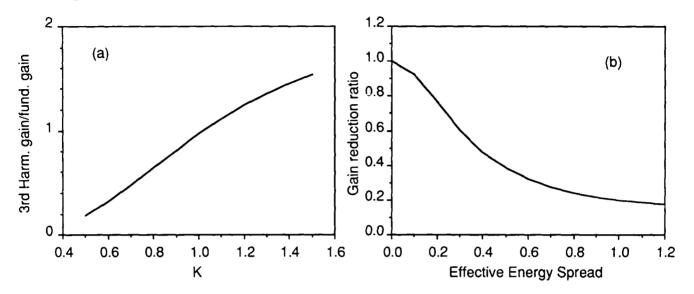
Figure 1. (a) Ratio of the third harmonic gain to the fundamental gain for an ideal electron beam and undulator. (b) Reduction in the gain ratio caused by the electron beam effective energy spread  $2N\delta\gamma/\gamma$ .
