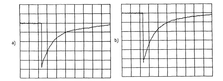
Fig. 9 - Measured voltage drop generated by the X-ray pulse in the circuit of Fig. 8. Vertical 200 mV/div, horizontal 2 ms/div; a) Plasma trigger voltage V=24 kV. Preionization electron number density n=3.5·107 cm<sup>-3</sup> b) V=16 kV, n=4.2·107 cm<sup>-3</sup>
