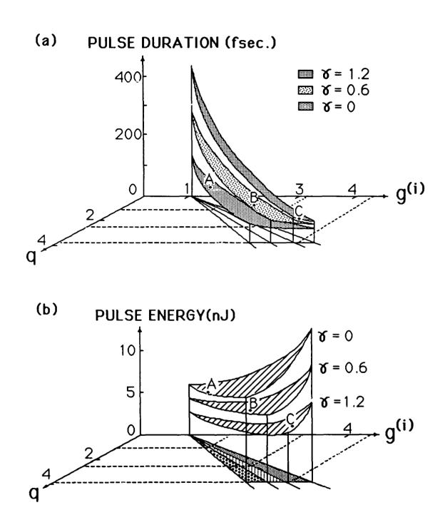
Fig. 2 Fundamental pulse, (a), duration and, (b), energy as a function of saturable loss, q, saturable gain, g(i), and the dimensionless parameter for second harmonic conversion efficiency,  $\gamma$ .
