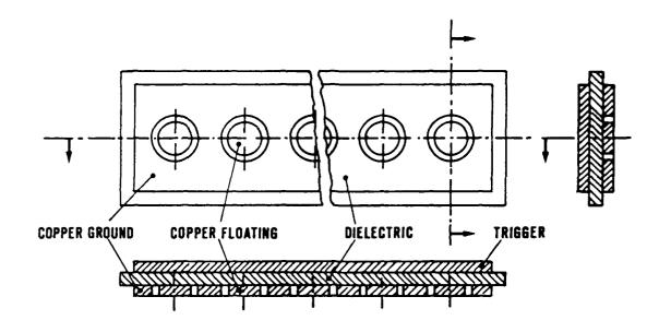
Fig. 2 - Scheme of the surface plasma cathode
