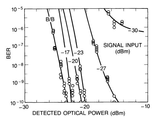
Figure 5 = Bit error rate curves obtained for different signal input powers ranging from -30 dBm to -17 dBm. B.B: back-to-back BER curve obtained without fiber amplifier. The amplifier g in is -15 dB (atter ref. [25]).
