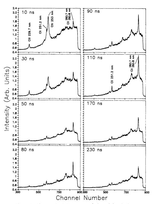
Figure 4- Time resolved UV spectra of the axial emission from a 500 um diameter, 5 cm long polyethylene capillary emitted by a 15 kV pulse. The external magnetic field applied is B=0. The time delay respect to the peak of the current pulse is indicated for each spectrum.
