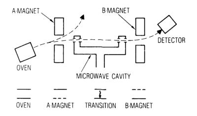
Figure 5. Conventional Cesium-Beam atomic clock.
