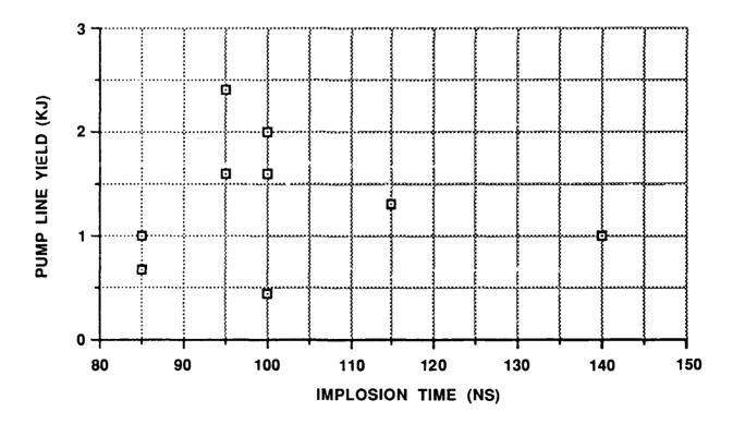
Figure 9. Sodium  $\mbox{He}_a$  Line Yield vs. Implosion Time
