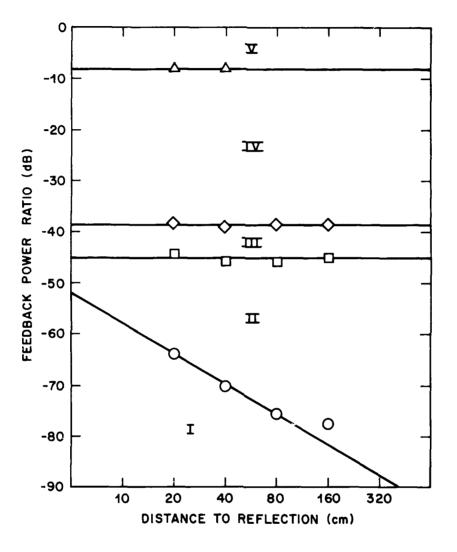
Figure 1: Plot of feedback power levels at which transitions between regimes occur, as a function of the distance to the reflection. Lines are drawn through the data points for clarity.
