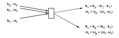
Figure 1.1 Schematic showing a general four-wave mixing scheme.
