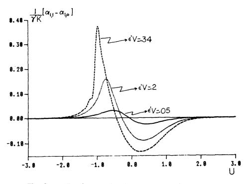
Fig. 3 The phase portion due to nonzero relaxation time, in the presence of self steepening, as function of U.
