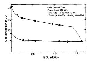
Figure 5: The oxygen poisoning of gold catalyst coating is shown by a hysteresis effect with O2 addition. The lower curve starts with an activated catalyst (note arrows). Decreasing the O2 pressure produces the upper curve.
