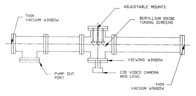
Figure 6: Schematic view of the tuning beam line.
