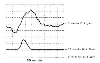
Figure 7. Typical time evolution of C-A gain 476.5 nm) and B-X fluorescence as a function of time in 1MV/cc power deposition device.
