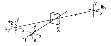
Fig. 1: DFWM in the Kerr-shutter configuration
