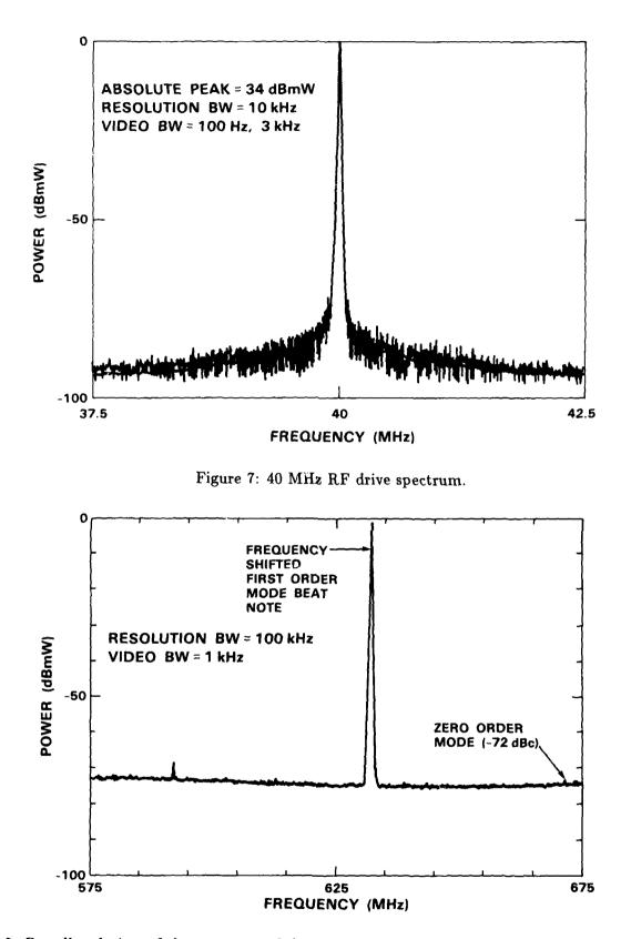
Figure 8: Broadband view of the spectrum of the reference laser heterodyned with an LO laser which is AO modulated by the 40 MHz sinusoidal RF drive signal.
