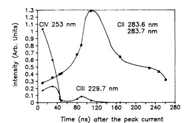
Figure 5- Evolution of the intensity of the emission from lines corresponding to different degrees of ionization of carbon in a polyethylene capillary discharge for 15 kV excitation in the absence of an externally applied magnetic field. The time is measured respect to the peak of the current pulse.
