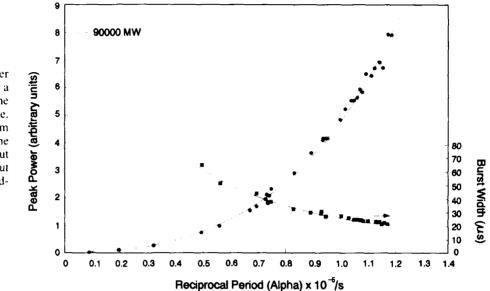
Fig. 5. Burst width and peak power of the GODIVA assembly plotted as a function of the reciprocal period. The dashed line is simply a guide for the eye. The solid curve has the functional form  $P \approx (\alpha^2/2b\alpha_r) (1 + \alpha^2\tau^2)$ , where b is the thermal quench rate of the device (about -0.2 cf<sup>c</sup>C),  $\alpha_r$  is the Rossi alpha (about 0.86 x 10<sup>6</sup> sec<sup>-1</sup>), and  $\tau$  has been adjusted for best fit to a value of 8.9 µs.
