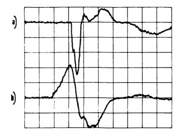
Fig. 4 - Current (a) flowing in the diode and voltage (b) measured at the transformer output of Fig. 3. Horizontal 1 µs/div. Vertical 240 A/div for the current, 30.8 kV/div for the voltage
