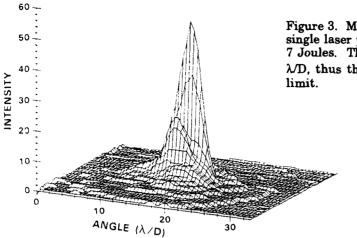
Figure 3. Measured far-field energy distribution for a single laser pulse. The total energy in this pulse was 7 Joules. The 64 x 64 CCD array subtends about 35  $\lambda$ /D, thus the laser is about 15 times its diffraction limit.
