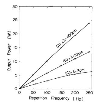
Fig. 8 Output power v.s. repetition frequency.
