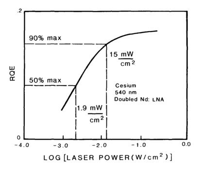
Figure 4. RQE versus laser pump power for the 540-nm transition when the cell signal transmission probability,  $P(\lambda_0)$ , is 0.1 and the reflectivity of the cell walls at the pump wavelength, R, is 0.98.
