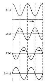
Fig. 1 Formation of a photorefractive index grating. (From ref. 1)
