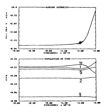
Fig. 7 - Cavity field and level populations for various cavity lifetimes, obtained by adiabatic (logarithmic) variation over indicated timescale from  $\tau_c = 100ps$  (beginning of interval) to  $\tau_c = 100ns$ .
