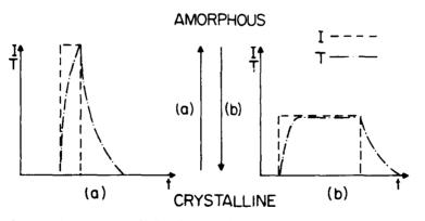
Figure 1. Reversible laser-induced phase transition.
