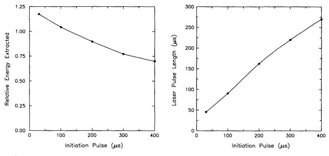
Fig. 1. Efficiency of energy extraction as a function of initiation pulse length. Total energy deposited was the same for all calculations.
