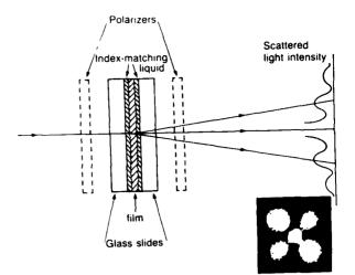
Fig. 2: A Mie-scattering setup for the optical characterization of a thin polymeric sheet.
