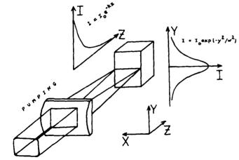
Fig. 1 The coordinates used and the distribution of the pumping intensity in the active medium.
