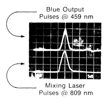
FIGURE 8: Generation of a short blue pulse by direct modulation of the laser diode (5 ns/div).
