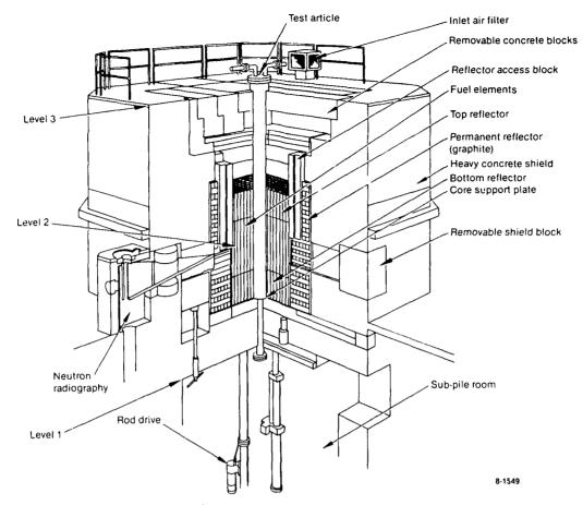
Figure 1. Cutaway view of the TREAT reactor.
