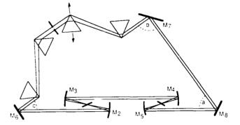
Figure 2. Dispersion-optimised cavities: a) linear configuration; b) CPM ring configuration.
