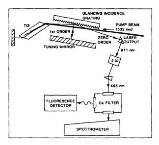
Figure 3. Schematic of experimental arrangement used to generate and monitor the narrow-band blue source.
