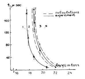
Fig.6 Time formation of the channel as a fuction of a quasi-stationary value of  $E_k/p$  at the beam current density 6 A/cm<sup>2</sup> C = 2.5 ns and p = 1 atm.
