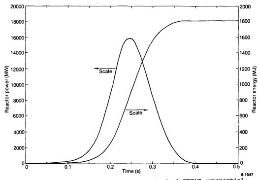
Figure 7. Reactor power and energy for a typical TREAT exponential burst transient.
