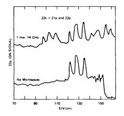
Figure 4 The  $22s+22s \rightarrow 22p+21p$  resonant collision signals with and without ImW of microwave power. With ImW of microwave power the radiatively emitted collisions are nearly as probable as the resonant collision process.
