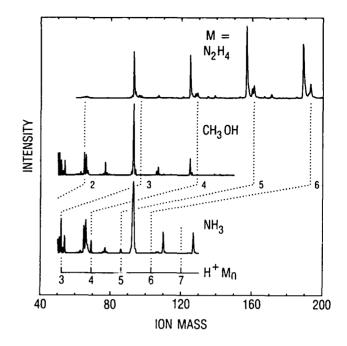
Fig. 3. 1-C REMPI/MS of  $A^+M_n$  clusters showing evidence for a critical solvent size in various solvents for dissociative proton transfer to form  $H^+M_n$ . Pulse energies were about 1.0 mJ (295 nm) for  $M = NH_3$  and  $CH_3OH$ , and 0.40 mJ (233 nm) for  $N_2H_4$ .
