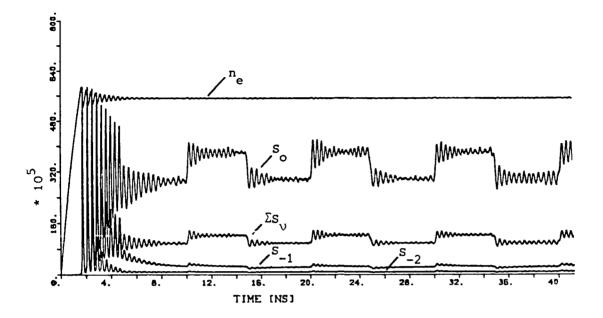
Fig. 3 Time dependence of the number of carriers and photons in the -2, -1 and main mode (total number of photons is plotted additionally).
