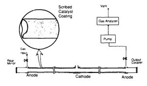
Figure 1: Schematic of the CO2 laser used for experiments. Details of the scribed gold catalyst coating are shown in inset.
