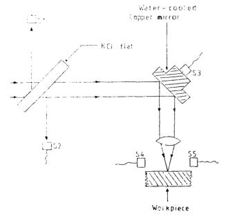
Figure 1: Experimental set-up for laser weld monitoring (gas shield nozzle not shown).
