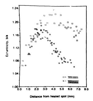
Fig. ll: Experimental plots of thermalpattern eccentricity vs. radial distance as obtained on a unidirectional single-sheet and on a  $(0^\circ, 90^\circ)$  double-sheet steelpolypropylene sample.
