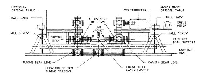
Figure 7: Schematic view of the overall mounting system for both the cavity and tuning beam lines.
