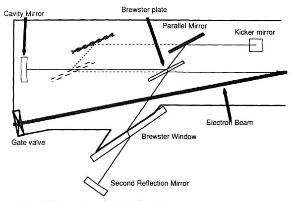
Figure 2. Schematic layout of the Mark III optical cavity. The undulator and moveable cavity mirror are to the right. Dashed lines indicate removeable output coupler. The second reflection mirror was not used in these experiments.
