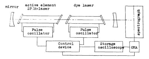
rig.1. Schematic diagram of intracavity absorption spectrometer
