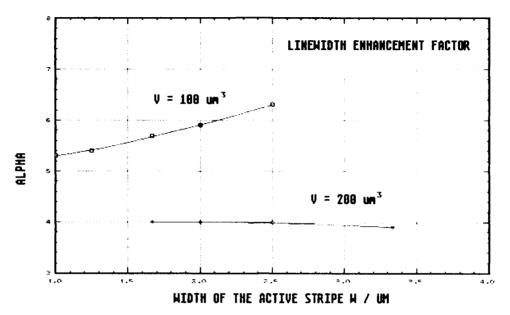
Fig. 5 Intrinsic linewidth enhancement factor  $\alpha$  versus width of the cavity for a volume V - 100  $\mu$ m<sup>3</sup> and V - 200  $\mu$ m<sup>3</sup> respectively.
