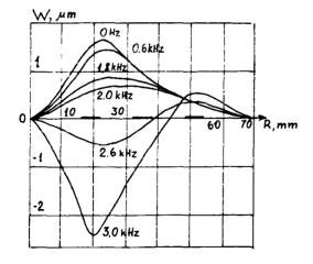
Fig.4 Profiles of vibrating adaptive mirror surface with sinusoidal drive voltage 400 V on peripherial actuator.
