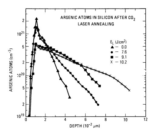
For the TUS reasons and of arsenic atoms as a function of depth for samples irradiated at different ensuch beauties. The tour curves show the arsenic profiles for the following samples:  $\blacktriangle$ , an unirradiated satisfy  $\bullet$ , a sample irradiated at  $E_L=7.6$  J/cm<sup>2</sup>;  $\blacksquare$ , a sample irradiated at  $E_L=9.1$  J/cm<sup>2</sup>; and X, a sample irradiated at  $E_L=10.2$  J/cm<sup>2</sup>.
