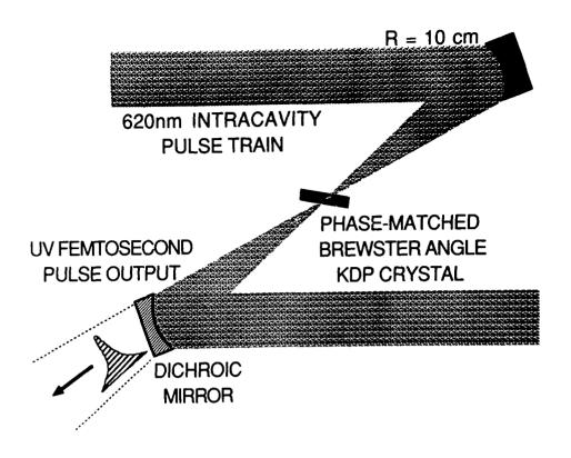
Fig. 3 Intracavity frequency doubling subresonator schematic.
