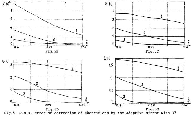
Fig.5 R.m.s. error of correction of aberrations by the adaptive mirror with 37 actuators vs the distance between actuators: 1 - A=Rm; 2 - A=0.8Rm; 3 - A=0.6Rm A - defocus, B - spherical aberration, C - distortion, D - coma, E- astigmatism.
