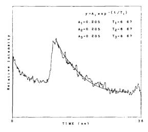
Figure 4. Relaxation decay curve of BP in methanol solution.
