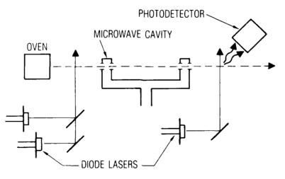
Figure 6. Diode Laser Cesium-Beam atomic clock.
