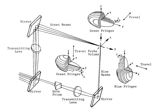
Figure 2: Formation of Three Supreimposed Sets of Interference Fringes in the Three-Dimensional Laser Doppler Velocimeter System.
