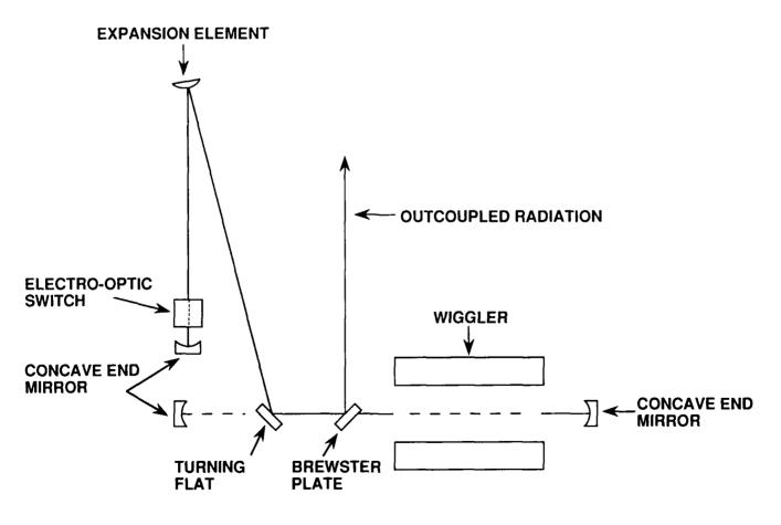
Figure 3. Schematic of the modified Mark III FEL optical cavity.
