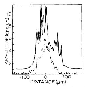
Figure 4. Predicted laser output power versus time (measured from the peak of the optical heating pulse) for the 209.78 A J=2-1 transition (solid line), and the 182.43 A J=0-1 transition (dotted line). Figure 5. Intensity versus position in the plasma for the 209.78 A J=2-1 transition (solid line) and the 182.43 A J=0-1 transition (dotted line). The two curves have been offset for clarity.
