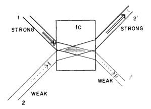
Fig. 3 Two beam coupling, aberrated beam 1 amplifies unaberrated beam 2.
