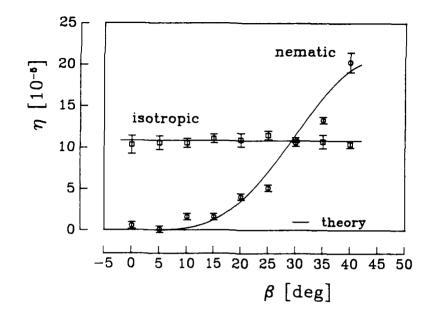
Fig.3: Diffraction efficiency vs. angle of incidence  $\beta$  measured with nematic and isotropic 5CB at Win  $\approx 0,54 mJ.$
