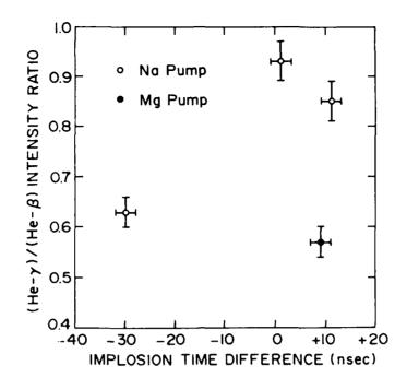
Figure 8. Ne IX line intensity ratios,  $\gamma/\beta$ , for the three shots in Figure 6 (open circles) and for the shot with MgF<sub>2</sub> in place of NaF (solid circle).
