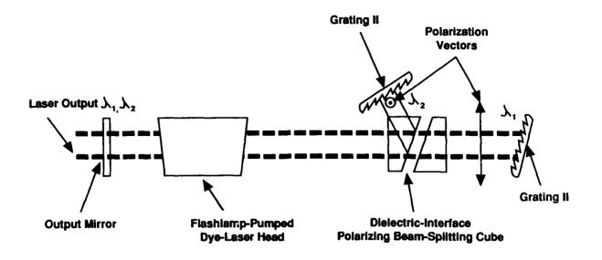
Fig.4. Optical arrangement for two simultaneous orthogonally polarized wavelength outputs
