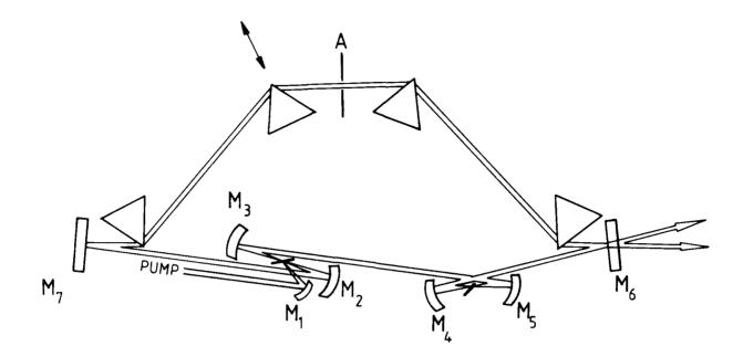
Figure 10 CPM ring cavity used for Coumarin featosecond dye lasers.
