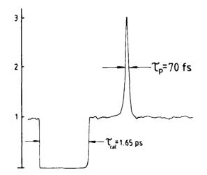
Figure 3. Autocorrelation trace of pulses of 70fs duration obtained at 573nm.
