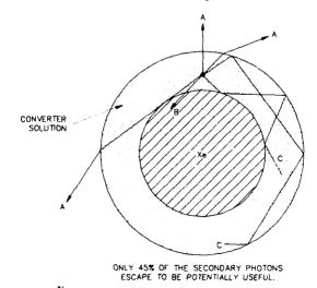
Fig. 7 Converted Photon Usage with Converter Solution in Flashlamp Water Jacket. See Table 1 for Explanation of Rays.
