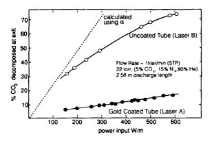
Figure 3: Measured CO2 decomposition at the laser exit as a function of input power for Laser A and Laser B in slow flow condition. A line, calculated from a and the CO2 flow rate, is also shown for comparison.
