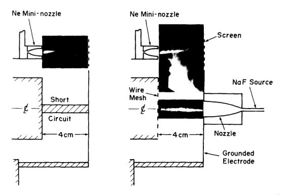
Figure 5. K-shell x-ray images of neon and NaF implosions superimposed across the diode gap of Gamble II. (a) Short circuit on axis and (b) NaF capillary plasma on axis.
