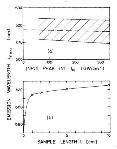
Fig.6: Wavelength of peak TPI-ASE emission versus (a) pump pulse peak intensity  $I_{0L}$  ( $\ell = 2 \text{ cm}$ ) and (b) sample length  $\ell$  ( $I_{0L} = 1.5 \times 10^{11} \text{ W/cm}^2$ ). Hatched region of (a) indicates spectral width (FWHM). Dye is 0.01 molar rhodamine B in HFIP.
