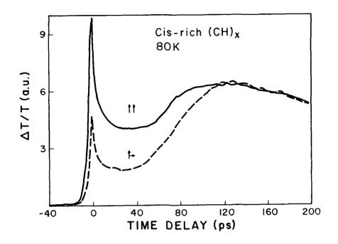
Fig.4: Transient  $\Delta T/T$  in a film of 80% cis/20% trans-(CH) with perpendicular (1) and parallel ( $\parallel$ ) pump-probe polarizations at  $\lambda = 620$  nm.
