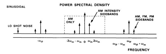
Figure 2: Heterodyned detector output power spectrum for small phase deviation sinusoidal PM or FM and for sinusoidal AM.
