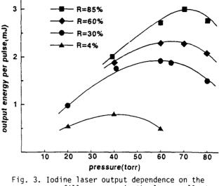
19. 3. Logine laser output dependence on the gas fill pressure in the laser cell at each output mirror reflectance when the iodine laser was pumped longitudinally.
