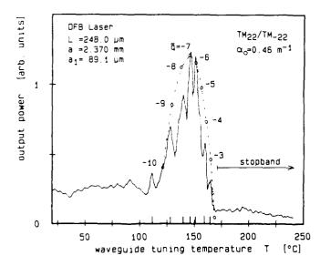
Fig. 1: Experimental demonstration of nonlinear gain saturation in an optically pumped 496 μm CH<sub>3</sub>F-DFB laser [33-35]
