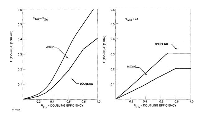
Figure 2. The frequency mixing approach (Option 2) can be more efficient than the frequency doubling approach (Option 1) but has higher complexity.
