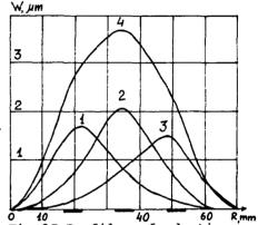
Fig.3C Profiles of adaptive mirror surface at +400 V drive voltage applied on 1 - left actuator, 2 - central actua-tor, 3 - right actuator, 4 three actuators semiltaneously
