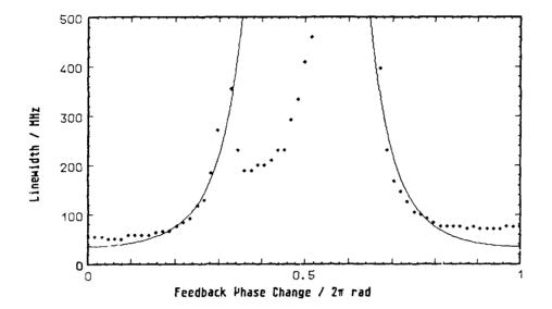
Fig. 4 Linewidth vs. feedback phase for medium feedback (C - 0.85)
