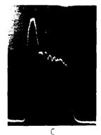
Figure 10: Weld pulses on a stationary target positioned on either side of the focus (a and c) and at the focus (b). Signal: 53, 50 msec/div. The pulse starts from the left.
