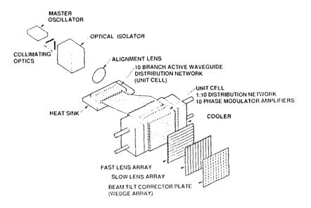
Figure 3. Ten Unit Cells are stacked to form the 100-emitter two-dimensional array. An eleventh cells serves as an active distribution network for the master oscillator.
