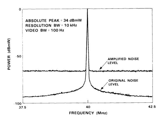
Figure 13: Very noisy 40 MHz RF drive signal.
