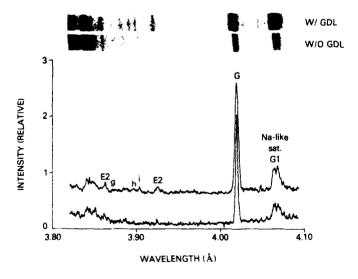
Fig. 2. Silver spectra obtained with the Si crystal spectrograph both with (top spectrum, shot 2) and without (bottom spectrum, shot 3) the midpulse irradiation by the 1.06  $\mu$ m GDL beam. Line G and electric quadrupole lines E2 arise from the neonlike stage; identifications of the fluorinclike lines g-i are given in Table 2.
