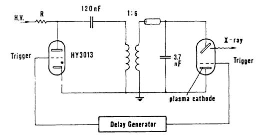
Fig. 3 - X-ray preionizer equivalent circuit
