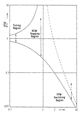
Fig. 7 Normalized linewidth vs. feedback parameter. Solid lines:  $\cos \Delta \varphi_x = \pm 1$ , dashed line:  $\cos \Delta \varphi_x = -1$ .
