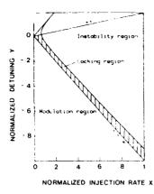
Fig. 8 Typical locking bandwidth for injection locking of diode lasers, the shaded region is where a lock occurs. (After ref. 14)
