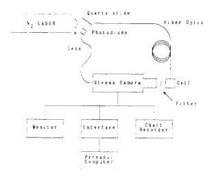
Figure 1. Schematic diagram of the time-resolved fluorimeter.
