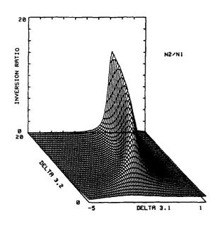
Fig.4 - Inversion of system in Fig. 3 as a function of the two detunings for  $k_3 = .0016$ ,  $k_2 = .0001$ ,  $\beta_1 = 1.0$ ,  $\beta_2 = 4.0$
