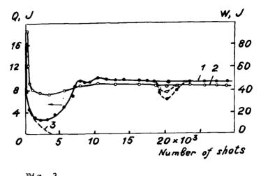
Fig. 3 Input W (1) and output Q (2) energies as a fuction of a number of shots. Gas mixture -  $CO_2$  :  $N_2 = 1$  : 1 p = 1 atm.
