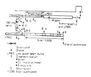
Figure -. 1 FEL Electron Beam Transport System
