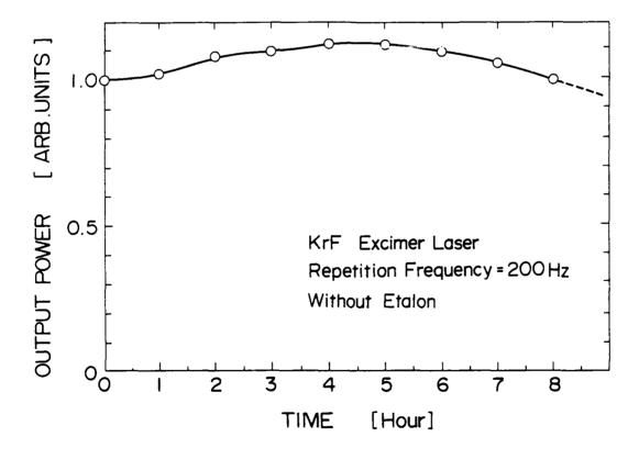
Fig. 2 Gas life-time under gas-sealed condition.
