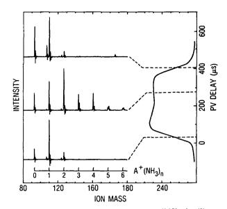
Fig. 2. 1-C REMPI TOF mass spectra (MS) of aniline-(NH<sub>3</sub>)<sub>n</sub> clusters as a function of the overlap of the laser pulse with the temporal profile of the pulsed valve (PV) output. Conditions were  $\omega_1 = 294$  nm, 0.05 mJ/pulse, 50 psi He.
