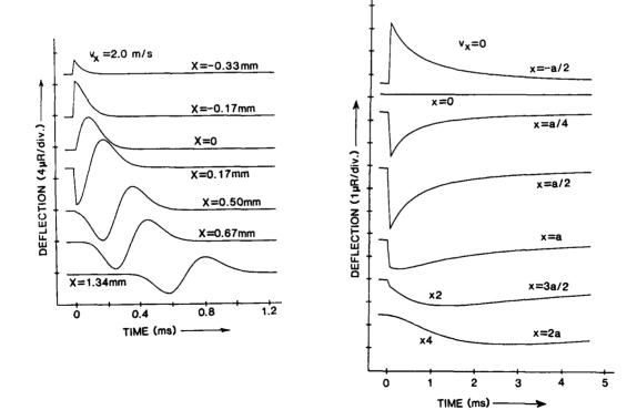
Fig. 5: Computed PTDS signals for pulsed excitation in a (a) medium moving with a velocity 2 m/s, and (b) in a stationary medium.
