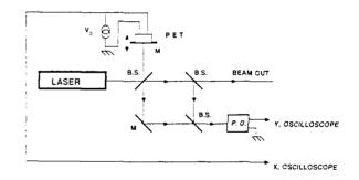
Fig. 3. Optical Spectrum Analyzer.
