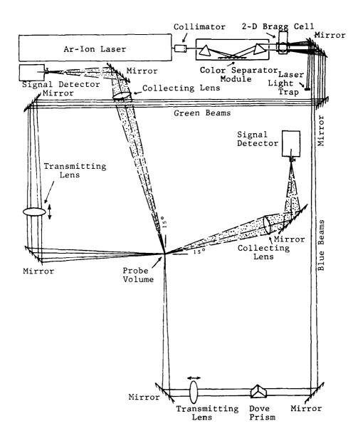
Figure 1: Three-Dimensional Laser Doppler Velocimeter System.
