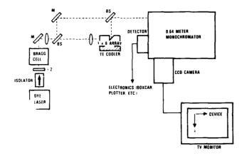
Figure 6 Experimental Arrangement for Injection Locking
