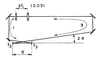
Figure 2: An elementary ring cavity
