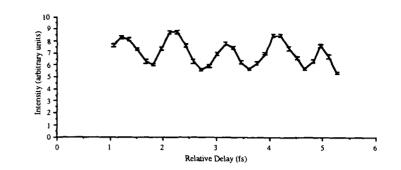
Figure 3.4 Typical set of data for the sum-frequency geometry showing signal intensity vs relative pulse delay. The x-axis has an arbitrary offset with respect to absolute zero relative delay. The sodium vapor was held at a temperature of 470 K.
