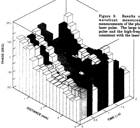
Figure 9. Results of the time-resolved laser wavefront measurements. Ten separate measurements of the phase are made during the 2- $\mu$ s laser pulse. The large temporal variation during the pulse and the high-frequency spatial variations are consistent with the laser's poor beam quality.
