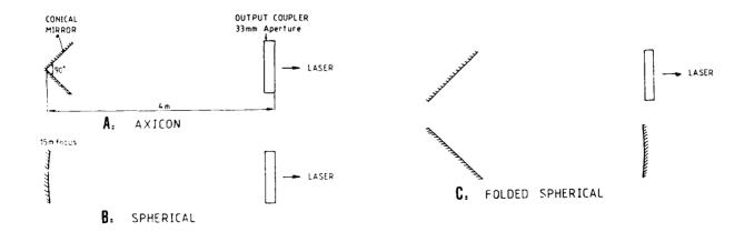
Figure 1: Resonator configurations which were investigated.
