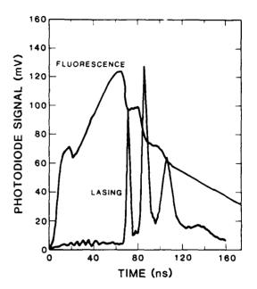
Figure 8. The temporal histories of the sidelight (upper curve) and lasing output (lower curve) of XeO, showing the multiple lasing pulses from the HR-HR cavity and the corresponding fluorescence depletions for each pulse. The mix was 30 ppm of both Xe and N<sub>2</sub>O in liquid argon.
