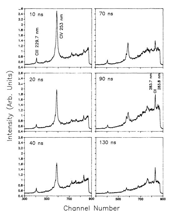
Figure 6- Time resolved UV spectra of the axial emission from a 500 um diameter, 5 cm long polyethylene capillary emitted by a 15 kV pulse. The external magnetic field applied is B=55 kG. The time delay respect to the peak of the current pulse is indicated for each spectrum.
