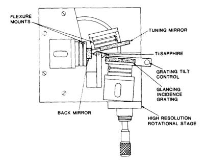
Figure 1. Single-longitudinal-mode (SLM), pulsed, Ti:Sapphire oscillator configuration.
