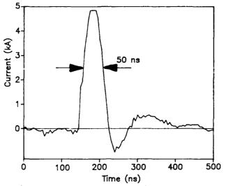
Figure 3- Current pulse measured through a 5 cm long, 500 um diameter polyethylene capillary excited by a  $40~\rm kV$  pulse from a 6.6 nF capacitor.
