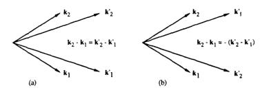
Figure 2.2 Possible ways to impose the geometries  $\mathbf{k'}_{21} = \pm \mathbf{k}_{21}$ . Note that the angles between the wavevectors are typically chosen to be a few milliradians and have been exaggerated here for the sake of clarity.
