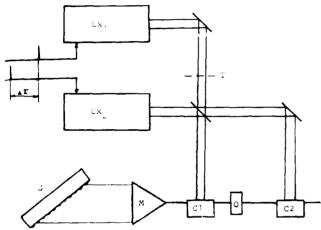
Fig. 4 The scheme of two-beam excitation of the dye laser. Ex1 and Ex2 - the excimer lasers;  $\Delta \tau$  - variable delay; T - attenuator; C1 and C2 - oscillator and amplifier dye cells; M - 40-fold multiprism beam expander; G - diffraction grating; O - output coupler.
