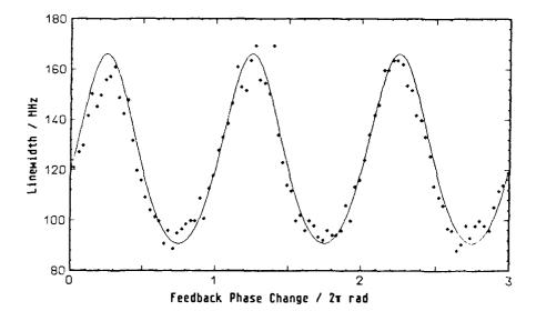
Fig. 2 Linewidth vs. feedback phase change for small feedback (C = 0.15)
