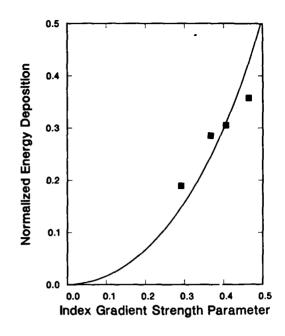
Figure 9. Normalized energy deposition (normalized pressure rise) is plotted against  $\gamma^+$  for Case A. The solid points are experimental measurements, and the line is the gasdynamic calculation. One experiment corresponds to one value of  $L_1$ .
