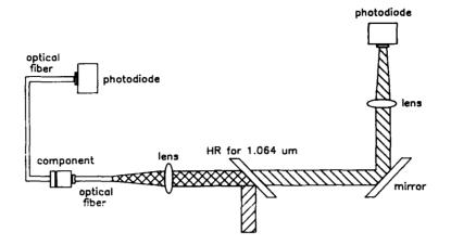
Figure 1 - Laser ignition apparatus.
