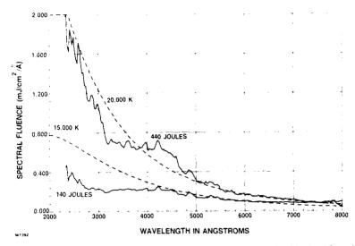
Fig. 2 Comparison of Measured Flashlamp Spectra with Blackbody Distributions
