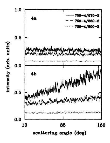
Fig. 4. Angular scattering spectra measured at ten randomly selected regions for three mullite glass-ceramic samples with 1 mm pinhole size. The spectra shown here are the sum of the ten spectra for each sample: (4a) the horizontal component, (4b) the vertical component.
