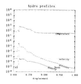
Fig. 5. Hydro profiles at 43.13 nanoseconds. Radial displacement is given in em.,  $log_{10}density$  in g/em<sup>3</sup>,  $log_{0}temperature$  in eV,  $log_{10}pressure$  in  $(1)^{12}ergs/em<sup>3</sup>$ , and  $log_{10}velocity$  in  $10^{4}$  em/nsec.
