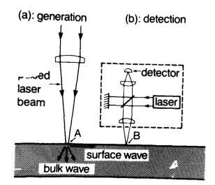
Fig. 12: Laser generation and detection of ultrasonic waves.
