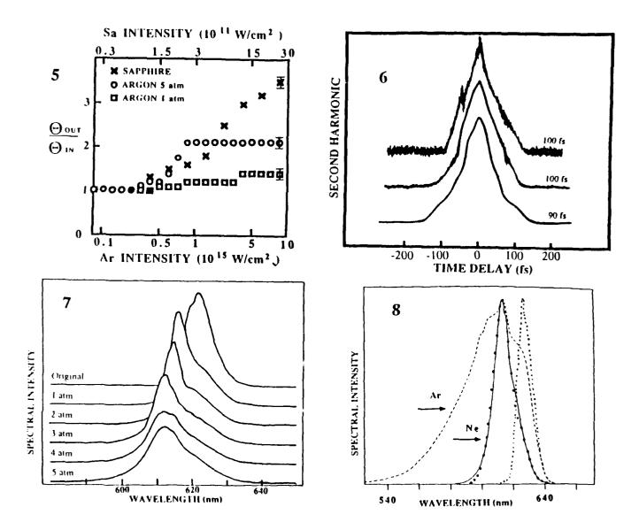
Fig. 5 Defocusing vs. peak focal intensity for sapphire, 1 atm. argon, and 5 atm. argon. The filled square and circle denote the first appearance of a breakdown spark
