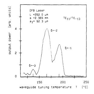
Fig. 2: (TE<sub>11</sub>/TE<sub>13</sub>)-modes of 496 µm CH<sub>3</sub>F-DFB laser with a periodic hollow metal waveguide. For parameters see text.
