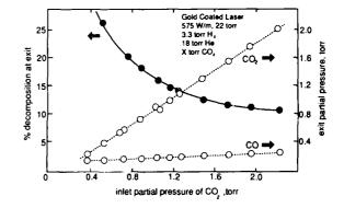
Figure 4: % CO2 decomposition as a function of inlet CO2 partial pressure for gold coated Laser A. The partial pressures of CO and CO2 at the exit are also plotted.
