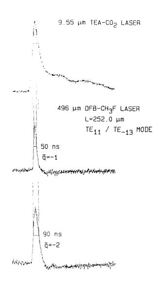
Fig. 3: Pulse shapes of the  $(TE_{11}/TE_{.13})$ -modes  $\tilde{q} = -1, -2$  of a 496  $\mu$ m CH<sub>3</sub>F-DFB laser and of the 9.55  $\mu$ m CO<sub>2</sub> pump pulse.
