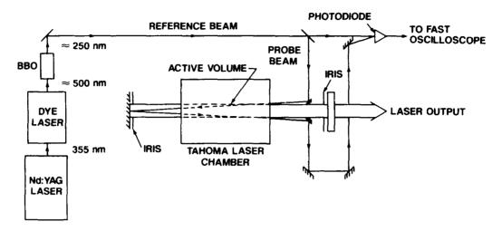
Fig. 1. Schematic of transient absorption measurement system.
