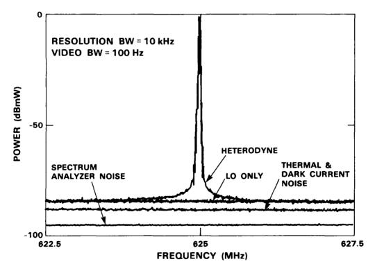
Figure 6: Spectrum of the reference laser heterodyned with an LO laser which is AO modulated by a 40 MHz sinusoidal RF drive signal.
