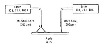
Fig. 7 - Sketch of the tests performed on a post mortem aorta segment with a bare fiber and a modified fiber. The argon laser pulse of different energy gave rise to the set of craters shown in Fig. 8.
