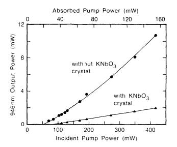
FIGURE 2: Output power at 946 nm versus diode-laser pump power with and without the  $KNbO_3$  crystal present in the cavity.
