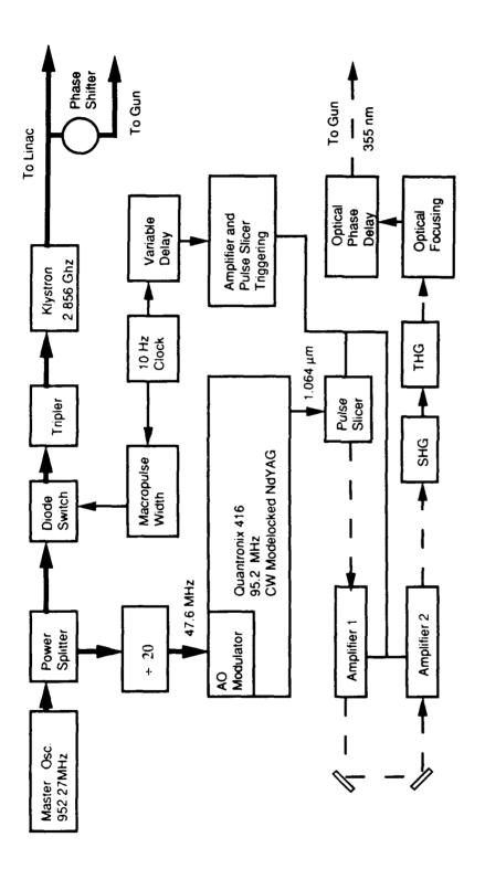
Figure #1 Schematic layout of the Nd:Yag drive laser system
