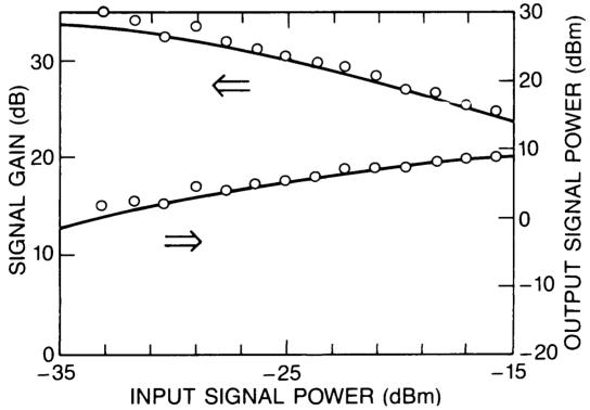
Figure 3 - Signal gain and output signal power at  $\lambda = 1.531$  µm vs. input signal power, obtained with 225 mW pump at  $\lambda = 514.5$  nm, in a lm long erbium-doped fiber amplifier.
