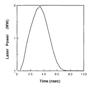
Fig.1 Calculated laser power output of the XeCl laser used by Xie, et al., in Reference 1. The gas mixture used is HCl:Xe:Ne = 2:40:5354 at P = 7.1 atm.
