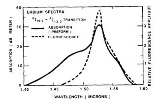
Fig. 8 Absorption and fluorescent spectra in the  ${}^{4}I_{15/2} - {}^{4}I_{13/2}$  transition for erbium in SiO<sub>2</sub> with 3.6 wt % Al<sub>2</sub>O<sub>3</sub>
