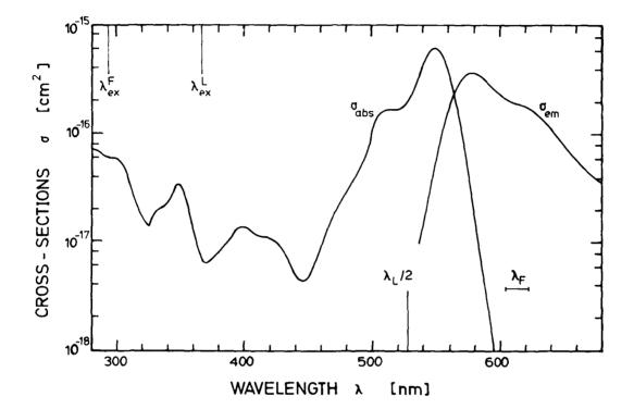
Fig.3: Absorption and emission cross-section spectrum of rhodamine B in hexafluoroisopropanol (HFIP).
