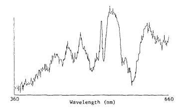
Figure 4 - Laser interaction emission spectrum of PETN.
