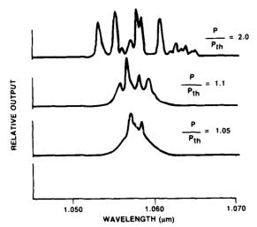
Fig. 4 The dependence of the laser spectrum on pump power above threshold  $P_{th}$  for 1 wt % Nd<sub>2</sub>O<sub>3</sub> in SiO<sub>2</sub> with 3.6 wt % Al<sub>2</sub>O<sub>3</sub>.
