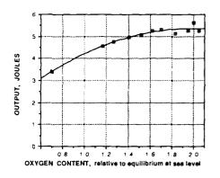
Fig. 15: The importance of Oxygen control.
