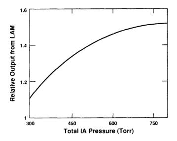
Fig. 15: Relative LAM output energy plotted vs IA laser gas pressure. Little advantage is derived from increasing the pressure beyond 700 torr for the present IA.
