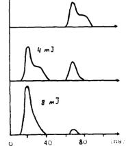
Fig. 5 Oscillograms of the dye laser oscillator output in the two-beam mode of excitation. Probing pulse energy  $E_2 = 2.5$  mJ.
