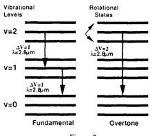
Figure 2. Short Wavelength Chemical Laser Operation
