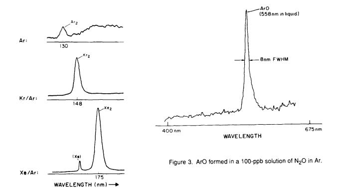
Figure 2. The noble gas dimer fluorescence spectra as seen in pure Ar, 10% Kr/Ar, and 0.01% Xe/Ar.
