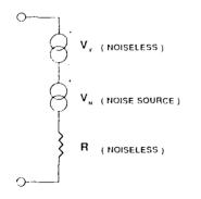
Fig. 2. Laser Input Electrical Model.
