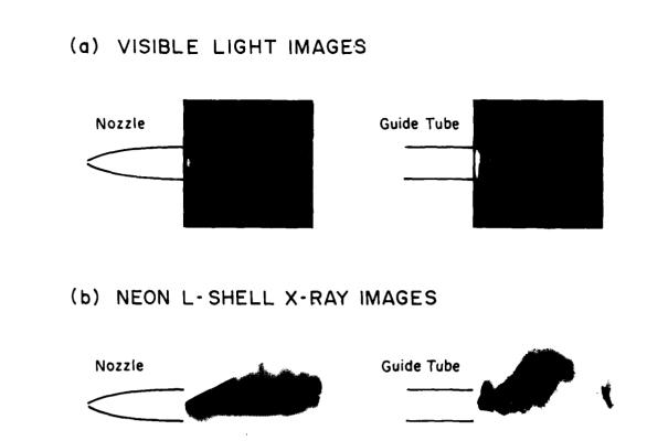
Figure 3. Images of neon from the gas puff coupled to either a mini-nozzle or a guide tube. (a) Visible-light images before implosion. (b) L-shell x-ray images of imploded neon. A transmitting screen is located 4 cm from the nozzle or guide tube.
