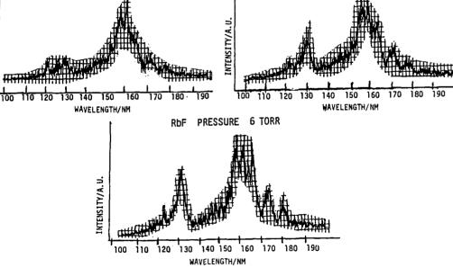
Figure 6. Pressure dependence of emission spectrum from laser produced-plasma-excited RbF vapor.
