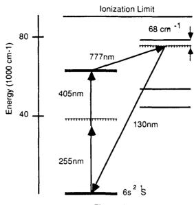
Figure 18. Generation of 130 nm Radiation by Four-Wave Mixing in Mercury Vapor
