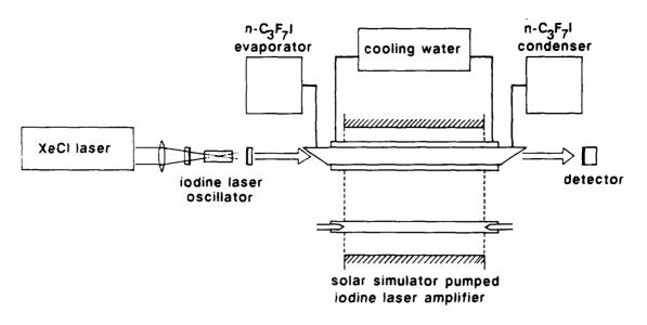
Fig. 6. Solar simulator pumped iodine laser MOPA system with the XeCl laser pumped iodine laser oscillator.
