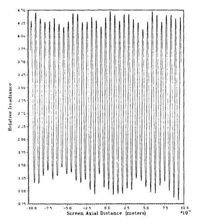
Fig. 5 Calculated interferogram resulting from the interaction of N slits  $33.34 \pm 1.21 \ \mu m$  wide.
