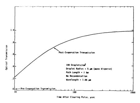
Figure 10. Optical transmission pre- and post-droplet evaporation.
