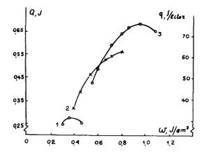
Fig.8 Output laser energy as a function of the input energy for metal (1) and perovskite (2,3) electrodes. Active volume  $-0.5 \times 0.5 \times 35$  cm; gas mixture  $CO_2$ :  $N_2$ :  $H_2 = 5$ : 5: 1; pressure - 1 atm; (1,2)  $U_0 = 20 \text{ kV}$ ; (3)  $U_0 = 23 \text{ kV}$ ;  $U_0$  is the charged voltage; the perovskite-La<sub>1-x</sub>Sr<sub>x</sub>COO<sub>3</sub>.
