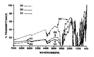
Fig. 4: Comparative transmission spectra for 90% polypropylene, 10% polycarbonate polymer blends with disperse spherical particles of typical diameters (a) 1-2 µm (b) 4-10 µm and (c) 10-20 µm.
