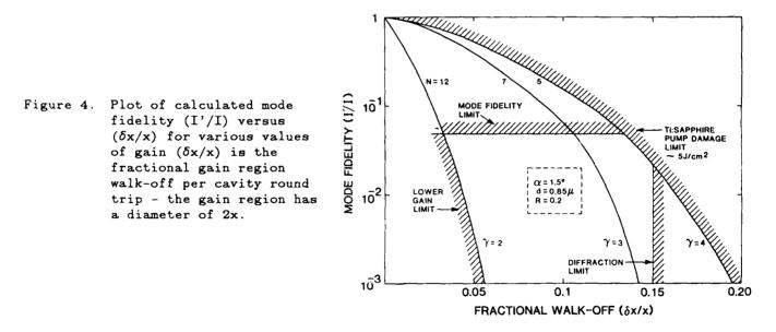
Further, diffraction limits the maximum value of  $L_2$  and  $(\delta x/x)$ . For example, we must require that the diffraction induced angular ray errors after N cavity round trips,  $\beta_N$ , be less than the angular shifts,  $\Delta \alpha$ , induced by the grating for adjacent longitudinal modes. The diffraction induced angular errors can be estimated using the Gaussian beam propagation equations. For a beam within its Rayleigh range one obtains:
