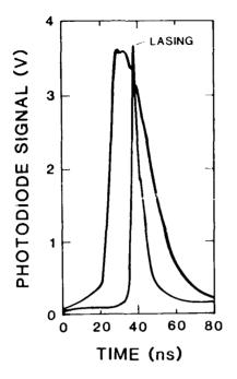
Figure 10. The Xe<sub>2</sub> time histories for sidelight fluorescence and lasing. At the moment of lasing a small depletion notch was seen in the sidelight.
