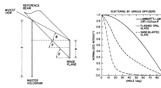
Figure 1 The disposition of the master and image plane holograms to determine the viewing angle.
