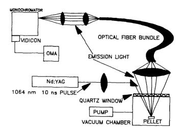
Figure 3 - Laser interaction emission spectroscopy apparatus.
