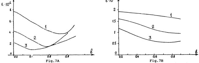
Fig.7 R.m.s. error of defocus (A) and astigmatism (B) correction by the adaptive mirror with 7 actuators vs the distance between actuators: 1 - A=Rm, 2 - A=0.8Rm, 3 - A=0.6Rm.
