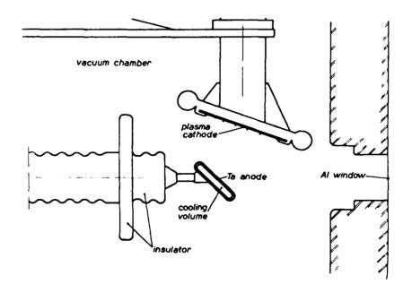
Fig. 1 - Vertical section of the X-ray diode
