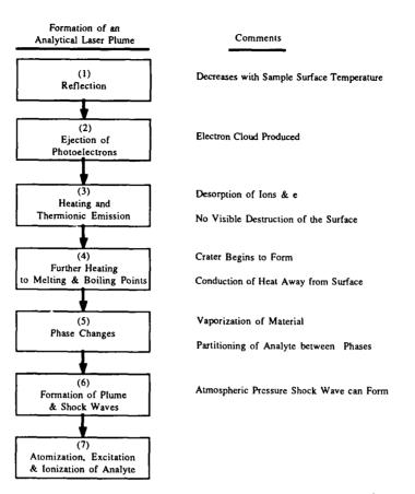
Figure 2. Schematic diagram of steps which can occur in the laser vaporization of a solid sample<sup>6</sup>.
