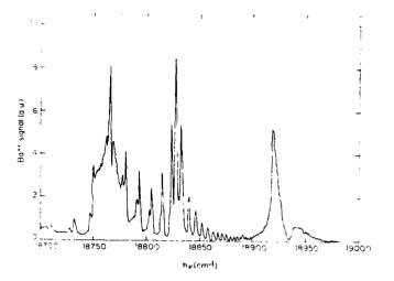
Figure 3 - Ba<sup>++</sup> production for laser frequencies from 18700 to 19000 cm<sup>-1</sup> There are three strong resonances, corresponding to the  $5d_{3/2}$ - $7s_{1/21}$ ,  $5d_{3/2}$ - $8p_{1/2}$ , and  $5d_{3/2}$ - $8p_{3/2}$  Ba<sup>+</sup> transitions, and the Ba<sup>+</sup>  $5d_{3/2}$  -nd four photon Rydberg series
