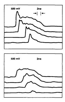
Fig. 3: The intensity at which the SBS cell reaches threshold is adjusted by changing the  $SF_6$  pressure to produce variable pulse widths from the front end.
