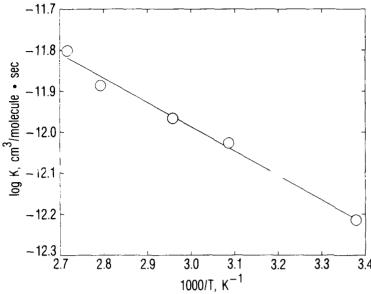
Fig. 5. Arrhenius plot of collision dissociation rate coefficients in He and Ne vs  ${\rm T}^{-1}\,\times\,10^3$  .
