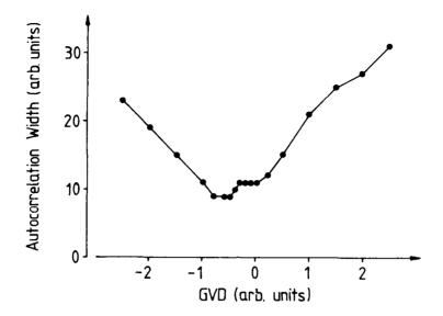
Figure 7. Theoretical variation of autocorrelation FWHM with intracavity GVD.
