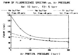
Figure 5. Fluorescence full spectrum bandwidth plotted as a function of krypton partial pressure for different buffers (He, Ne and Ar)
