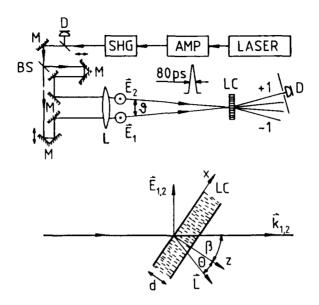
Fig.1: Selfdiffraction arrangement (M:Mirror, BS:Beamsplitter, LC:Liquid Crystal, D:PIN-10 Diode, L:Lens f = 1000 mm) and liquid crystal orientation (L:director, K<sub>1,2</sub>:wave vectors of incident beams, E<sub>1,2</sub>:optical field strengths).
