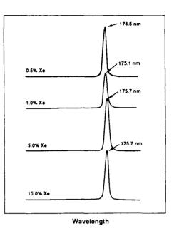
Figure 11. The red shift of the lasing wavelength of  $Xe_2$  as a function of the xenon concentration in the argon host.
