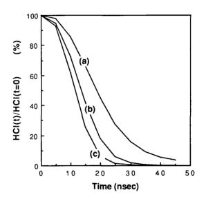
Fig.6 Depletion of HCl molecules for various peak values of the discharge-current. (a):  $J_{peak} = 10 \text{ kA}$ , (b):  $J_{peak} = 20 \text{ kA}$ , (c):  $J_{peak} = 30 \text{ kA}$ .
