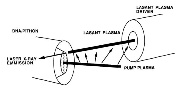
Figure 2. Physics International's Approach to Photopumped X-ray Laser Scheme.
