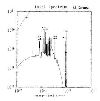
Fig. 6. Emission spectrum at 43.13 nanoseconds. The instantaneous power (ergs/ sec-cm-keV) is given as a function of photon energy (keV). Selected emission lines are identified.
