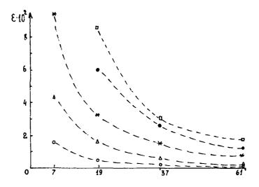
Fig.8 R.m.s. error of correction of aberrations by the adaptive mirror with hexagonal arrangement of actuators vs the number of actuators:  $\circ$  - defocus,  $\Delta$  - spherical aberration,  $\Box$  - distortion,  $\bullet$  - coma, # - astigmatism.
