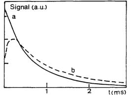
Fig. 4 - Theoretical time dependence of the collinear detection signal in a low absorbing thick sample with a pulsed excitation at t = 0 and for two pump-probe beams distances :
