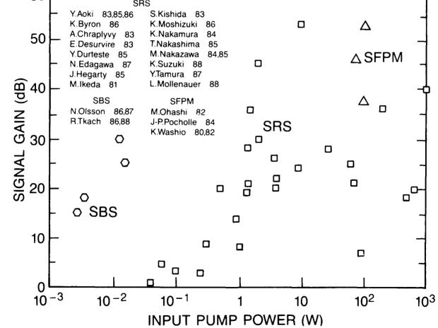
Figure 1 - Maximum gains vs. launched pump power reported for nonlinear fiber amplifiers. SFPM: stimulated four photon mixing, SRS: stimulated Raman scattering, SBS: stimulated Brillouin scattering.
