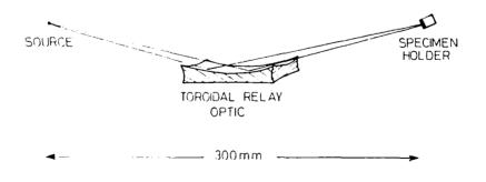
Fig.3 X-ray Focussing Element
