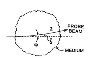
Fig. 4: Deflection of a probe beam propagating in an inhomogeneous medium.
