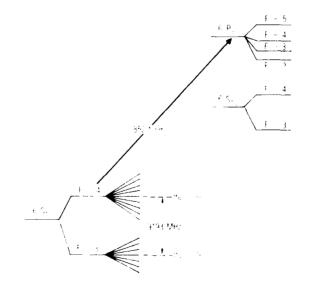
Figure 1. Energy level diagram for Cs133
