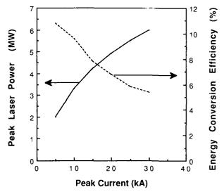
Fig.3 Calulated peak laser power output and energy-conversion-efficiency of the XeCl laser pumped by hypothetical discharge currents as functions of peak value of the discharge current. The gas mixture used is HCl:Xe:Ne = 2:40:5354 at p = 7.1 atm.
