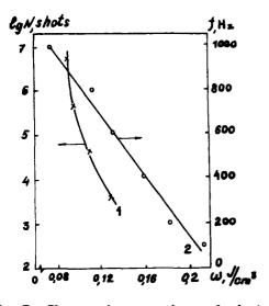
Fig.7 The maximum number of shots N (1) and maximum excitation pulse repetition frequency f (2) as a function input energy. Gas mixture  $-CO_2$ : N<sub>2</sub> : He = 1 : 1 : 8. Gas pressure - 1 atm. Discharge pulse duration - 250 ns; f = 400 Hz
