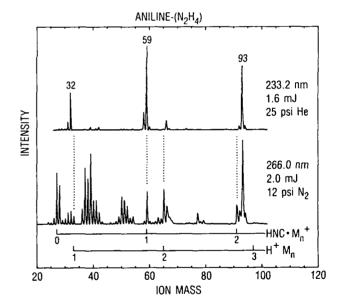
Fig. 6. 1-C REMPI/MS of A- $(N_2H_4)_n$  clusters for different excitation conditions. The appearance of the fragment clusters  $\text{HNC} \cdot (N_2H_4)_n^+$  is evidence for a dissociation-induced charge transfer mechanism. Numbers over peaks denote amu.
