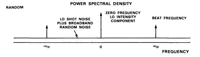
Figure 3: Heterodyned detector output power spectrum with random PM or or AM of the LO. The reference or received signal is assumed to be a monochromatic laser or tone signal at radian frequency  $\omega_{IF}$  from the optical carrier frequency.
