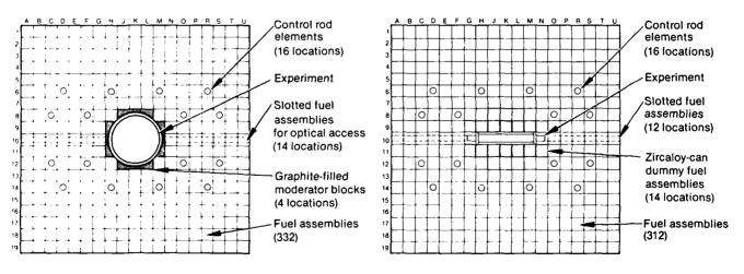
Figure 10. TREAT core configuration for original version of future NPL experiment.
