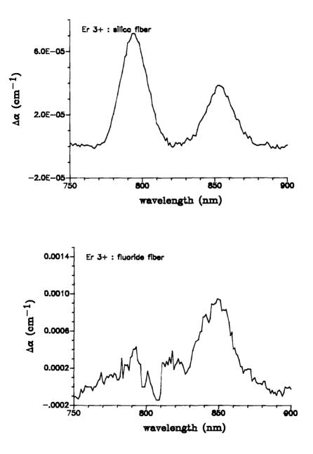
Figure 1. ESA difference spectra for Er<sup>3+</sup> in germania doped silica fiber (upper) and ZBLAN fiber (lower). The absence of the 800 nm ESA band in ZBLAN fiber indicates closely similar GSA and ESA intensities in the fluoride glass.
