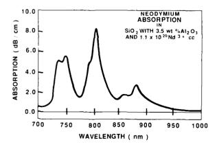
Fig. 2 Infrared absorption spectrum of 1.5 wt  $\% \text{ Nd}_2\text{O}_3$  in SiO<sub>2</sub> with 3.5 wt  $\% \text{ Al}_2\text{O}_3$
