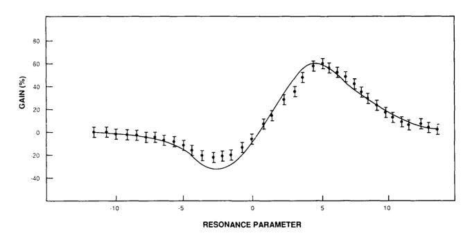
Figure 2. Power amplifier small signal gain as a function of the resonance parameter. The solid curve is a FELEX simulation.
