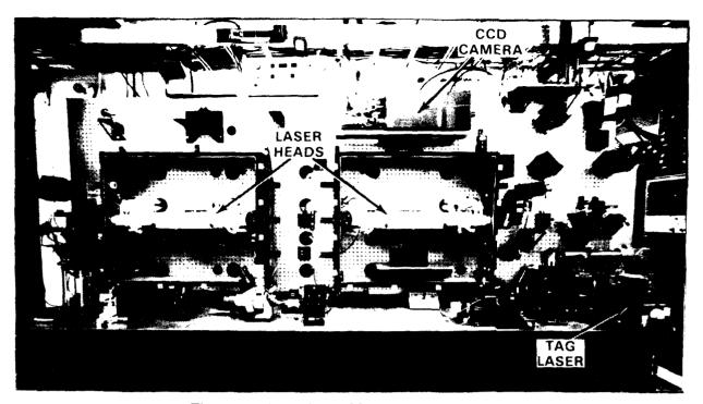
Figure 1. A single flashlamp-pumped, pulsed dye laser mounted on a vertical optical bench at Lincoln Laboratory. The CCD camera is used for measuring the far-field energy distribution of the laser The integrated-optics wavefront sensor is mounted on the horizontal portion of the optical bench.
