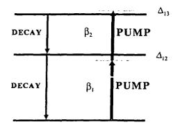
Fig.3 - Three level system which can show inversion for large intermediate level detuning.
