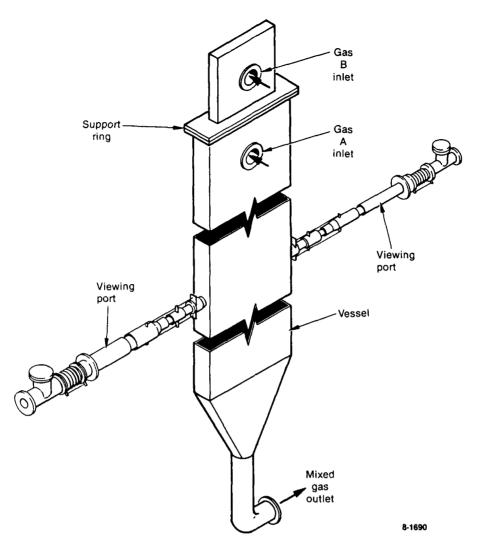
Figure 9. Original configuration of future NPL experiment.
