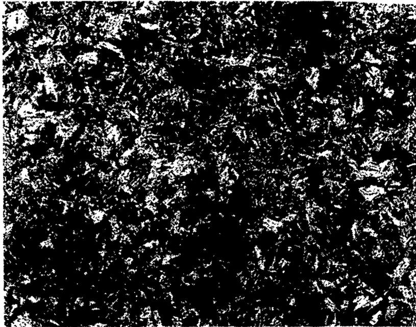
Fig. 4.2 Microstructure (x100) of high strength fine grain size condition of steel (HF).
