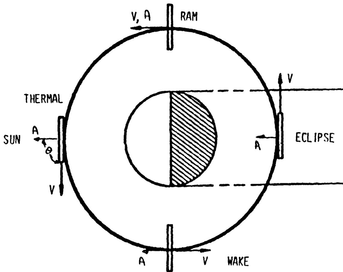
Figure 4.5 Changes in Environmental Conditions Over Orbit
