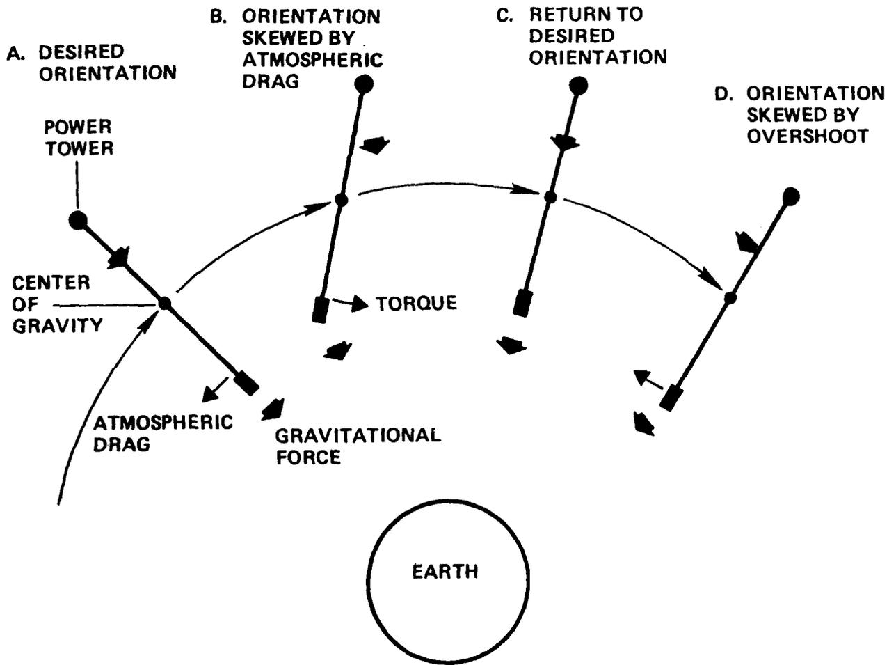
Figure 4.11 Drag Torques on Long, Unsymmetric Space Structures
