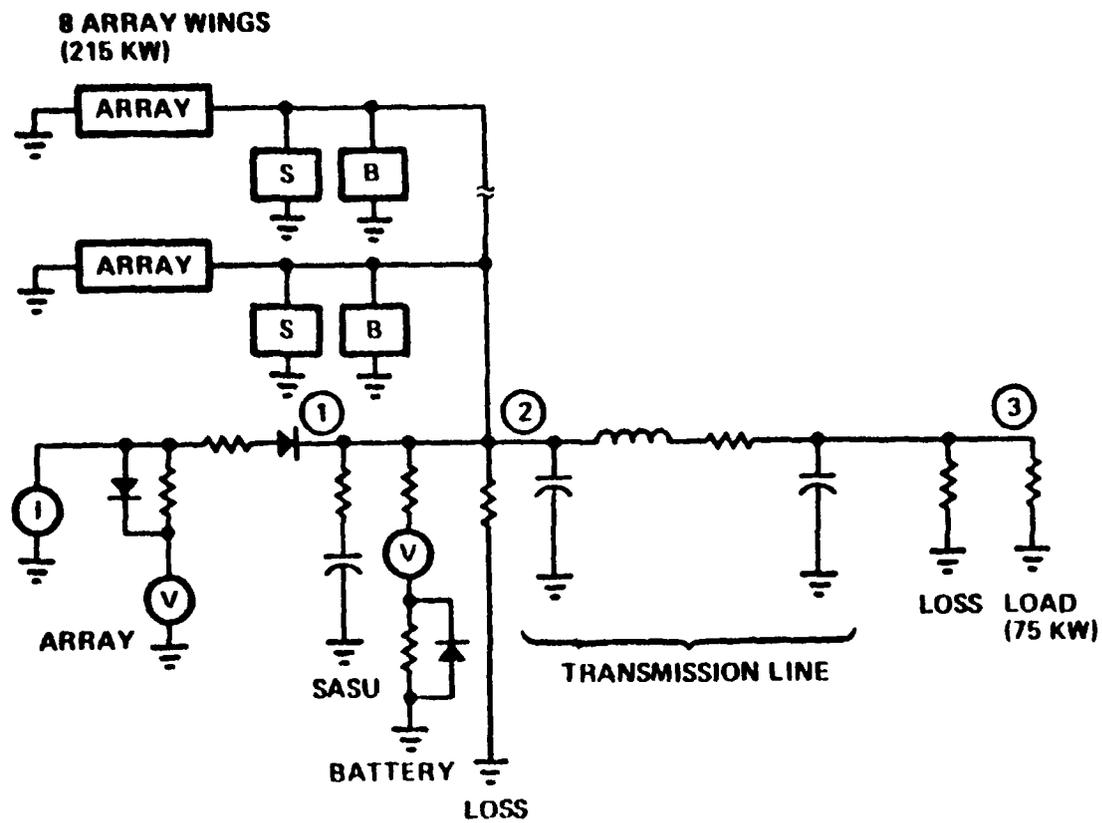
Figure 4.7 Discharge Transient Circuit Model (DC Generation/DC Transmission)
