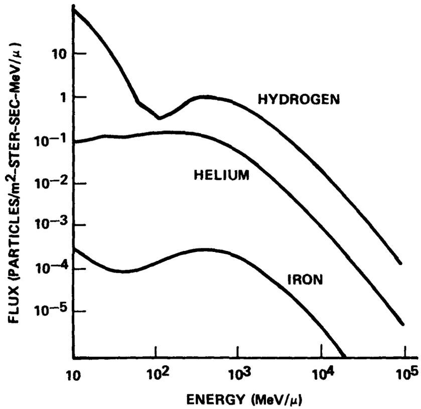
Figure 4.9 Maximum Cosmic Ray Environment: Free Field During Solar Minimum
