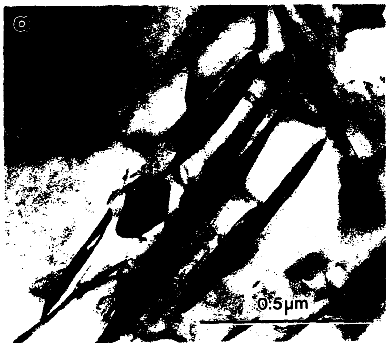
Fig. 10. (a) Needles observed in alloy annealed at 700^{\circ}\text{C} and (b) identified as the L1_0 phase.
