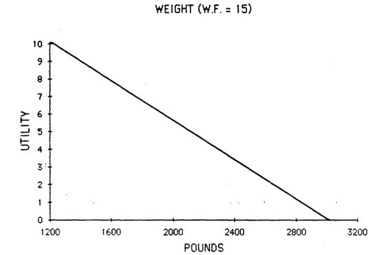
Figure 5.3-8. Utility Function for Weight, 19.5 Ton Vehicle
