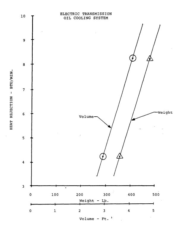
Figure 5.2-16. Electric Transmission Oil Cooling System Estimates
