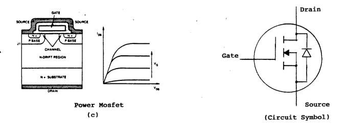
Figure 5.7-1. Power Semiconductor Devices, characteristics, and Circuit Symbols
