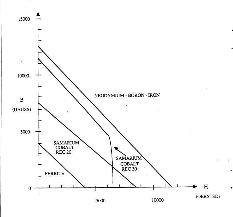
Figure 5.7-7. Demagnetization Chart of Magnetic Materials
