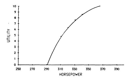
Figure 5.3-1. Utility Function for Sprocket Power, 19.5 Ton Vehicle
