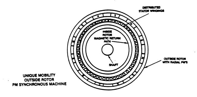
Figure 5.4-12. Unique Mobility Traction Motor Cross Section
