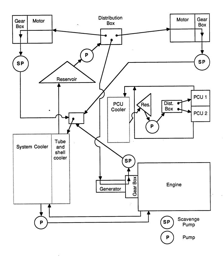
Figure 5.4-25. Cooling System Flow Diagram for Garrett Concepts
