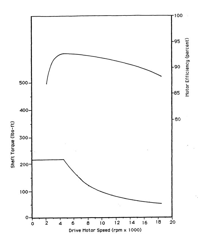
Figure 5.4-8 Torque and Efficiency Versus Speed for 192 Horsepower Garrett PM Motor
