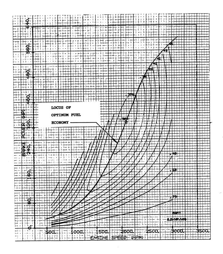
Figure 5.4-37. Fuel Map for VTA-903T Engine
