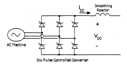
Figure 5.4-30. PM AC Machine with Controlled Converter
