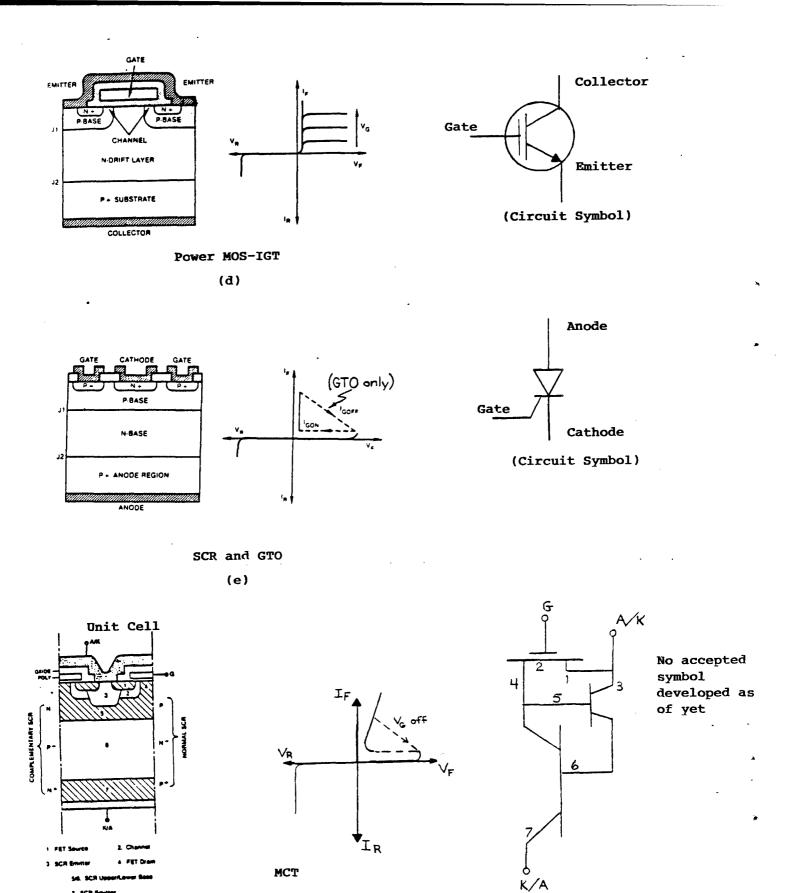
Figure 5.7-1. Power Semiconductor Devices, characteristics, and Circuit Symbols (Continued)
