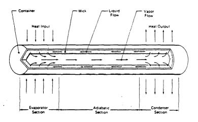
Figure 5.7-16. The Heat Pipe
