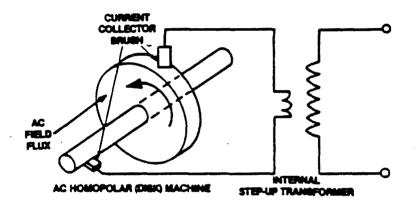
Figure 5.2-8. AC Homopolar Machine
