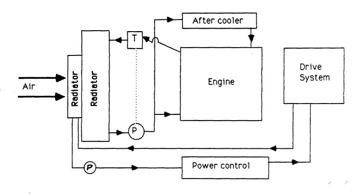
Figure 5.4-28. Cooling System for Unique Mobility Concepts
