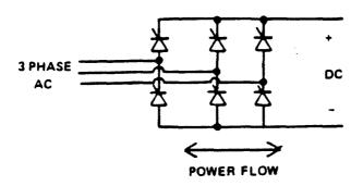
Figure 5.4-3. Rectifier Bridge Schematic
