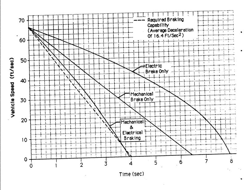
Figure 5.4-57. Brake System Performance
