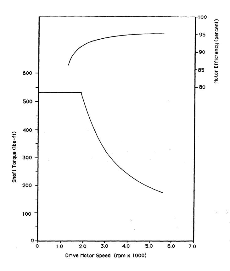
Figure 5.4-4. Torque and Efficiency Versus Speed for 192 Horsepower ACEC DC Motor
