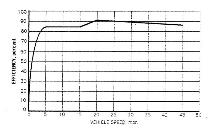
Figure 5.4-23. Efficiency of 40 Ton Unique Mobility Concept IV-2
