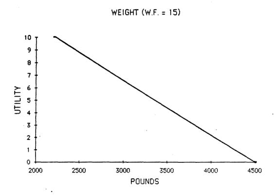
Figure 5.3-9. Utility Function for Weight, 40.0 Ton Vehicle
