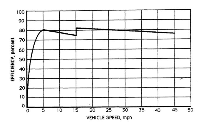
Figure 5.4-22. Efficiency of 40 Ton Garret Concept I-3
