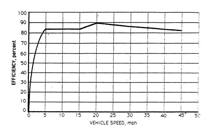
Figure 5.4-21. Efficiency of 19.5 Ton Unique Mobility Concept IV-2
