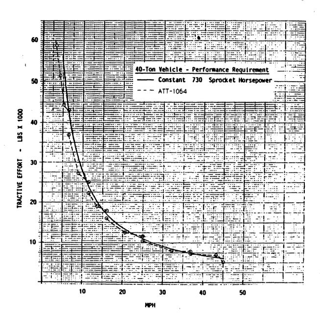
Figure 5.5-4. Tractive Effort for ATT1064 Transmission, 40.0 Ton Vehicle
