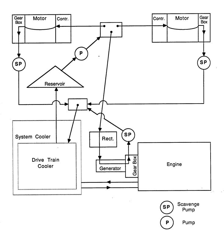
Figure 5.4-29. Cooling System Flow Diagram for Unique Mobility Concepts
