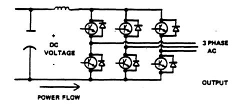
Figure 5.4-11. Transistor Inverter Schematic
