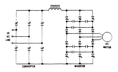
Figure 5.2-13. Converter/Inverter Type PCU
