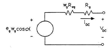
Figure 5.4-31. DC Equivalent Circuit of a Permanent Magnet Generator Operating into a Current Source Controlled Converter
