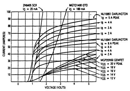
Forward Conduction Characteristics 0.5 V/Div. 10 A/Div.  $T_C = 25^{\circ}C$ Pw = 300  $\mu$ s, f = 60 Hz
