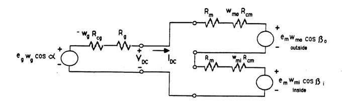
Figure 5.4-34. AC Equivalent Circuit of ACEC Drive
