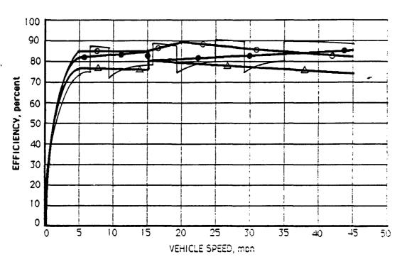
Figure 5.5-1. Comparison of Efficiency for Electric and Mechanical Transmissions of the 19.5 Ton vehicle Category
