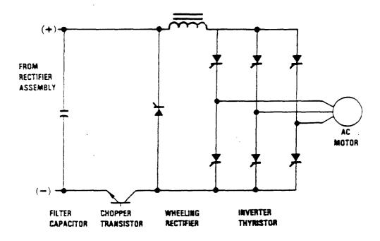
Figure 5.2-12. Chopper/Inverter Type PCU
