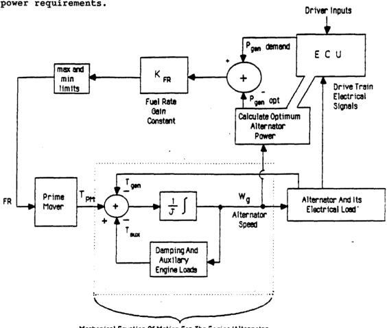
Mechanical Equation Of Motion For The Engine/Alternator
