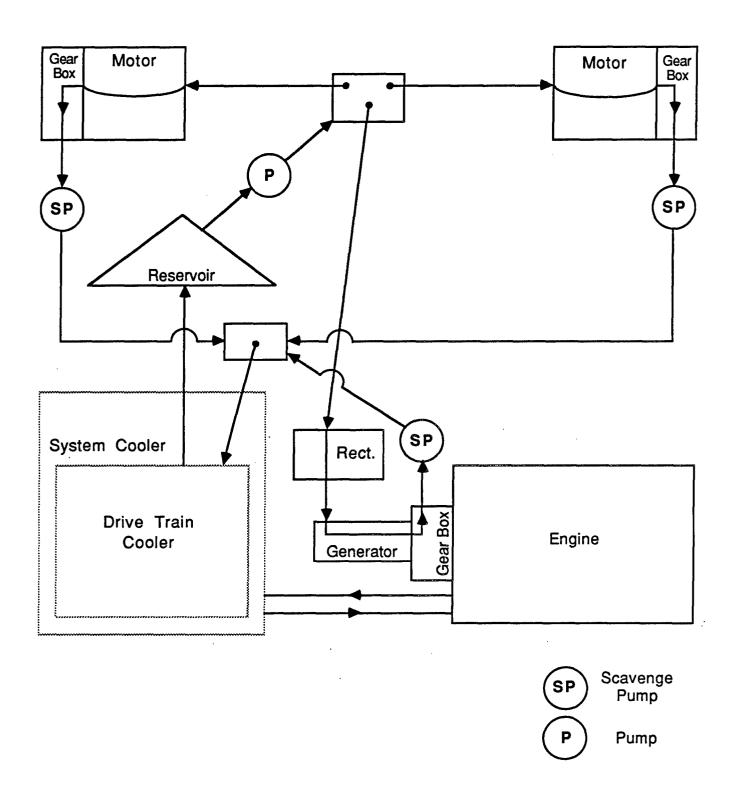
Figure 5.4-27. Cooling System Flow Diagram for ACEC Concept
