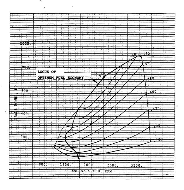
Figure 5.4-38. Fuel Map for AD1000 Engine
