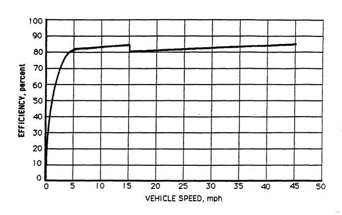
Figure 5.4-19. Efficiency of 19.5 Ton ACEC Concept I-5
