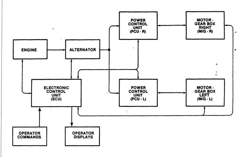
Figure 5.2-14. Electronic Control Concept for Electric Propulsion System
