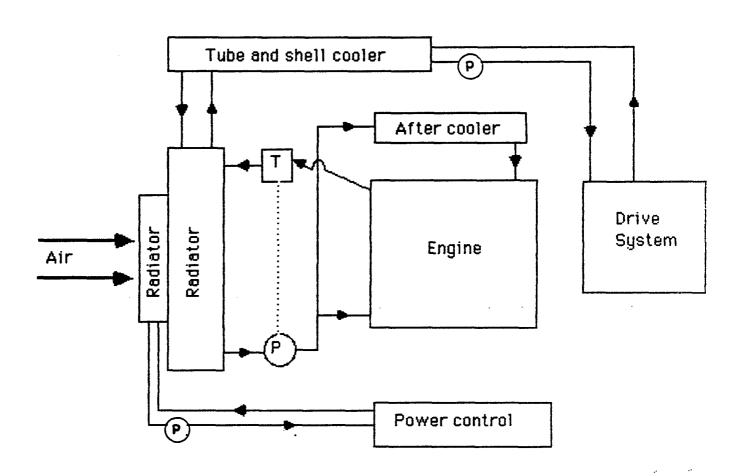
Figure 5.4-24. Cooling System for Garrett Concepts
