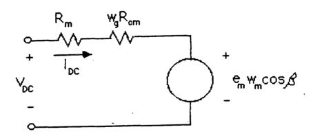
Figure 5.4-32. DC Equivalent Circuit of a Permanent Magnet Motor Operated from a Current Source Controlled Converter
