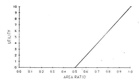
Figure 5.3-4. Utility Function for Skid-Out Capability
