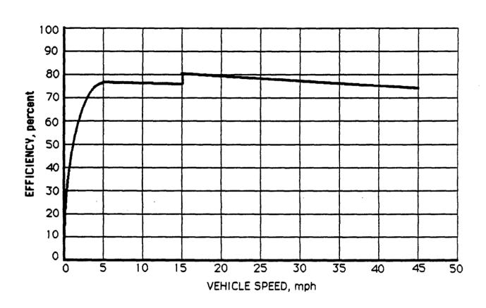
Figure 5.4-20. Efficiency of 19.5 Ton Garrett Concept I-10
