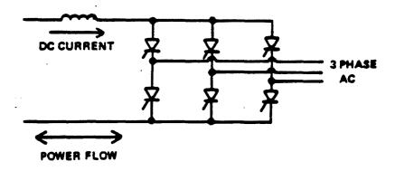
Figure 5.4-7 SCR Inverter Schematic
