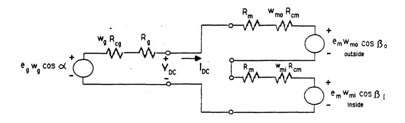
Figure 5.4-53. An Equivalent Electrical DC Circuit of the Garrett 19.5 Ton Concept Electric Drive Train
