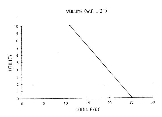
Figure 5.3-5. Utility Function for Volume, 19.5 Ton Vehicle
