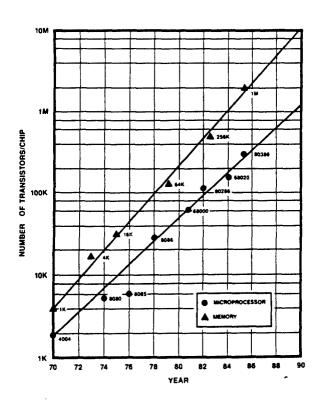
Figure 5.7-11. Number of Transistors Per Chip Versus Time
