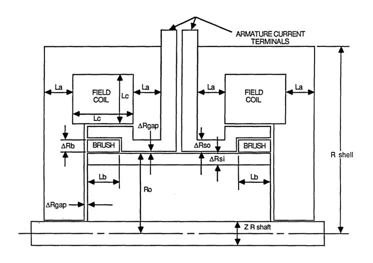
Figure 5.7-22. Diagram of Homopolar Machines
