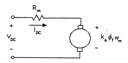
Figure 5.4-33. DC Equivalent Circuit of a DC separately Excited Machine
