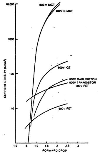
Comparison of high gain turn-off device forward drop. The IGT and MCT are calculated based on the same identical doping and life-time profiles.
