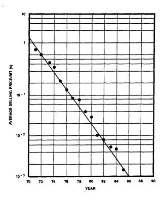
Figure 5.7-12. Cost of Computing Power Versus Time
