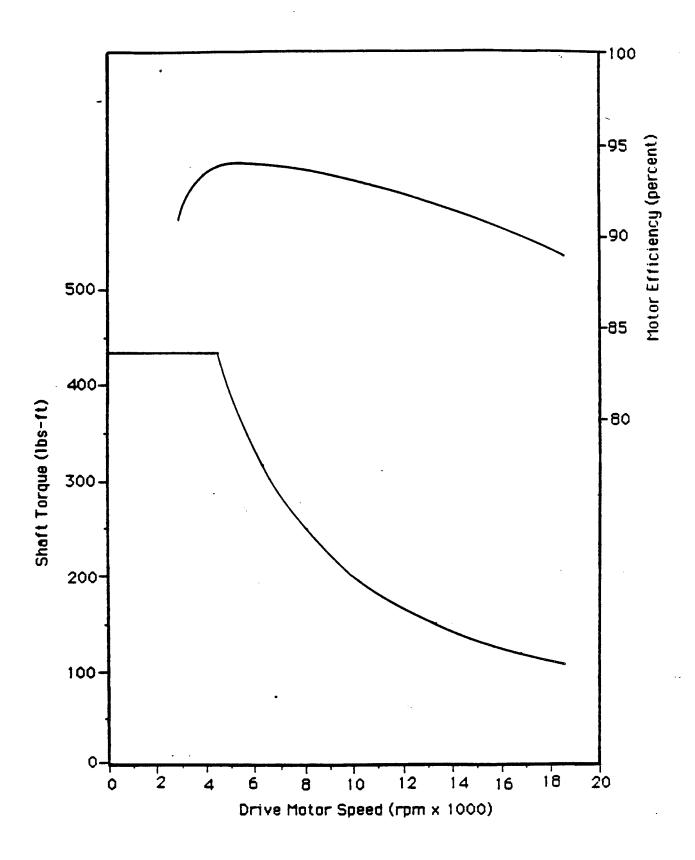
Figure 5.4-16. Torque and Efficiency Versus Speed for 384 Horsepower Garrett PM Motor
