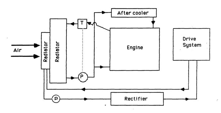
Figure 5.4-26. Cooling System for ACEC Concept
