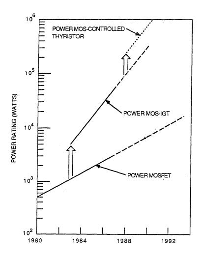
The increase of the power handling capability of power MOS devices with progress in technology and the introduction of new device types
