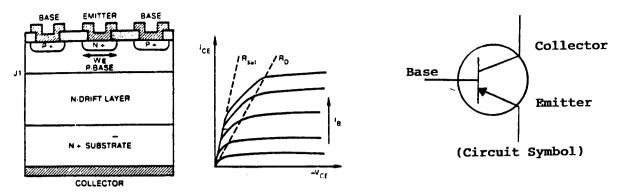
Power Bipolar Transistor (a)
