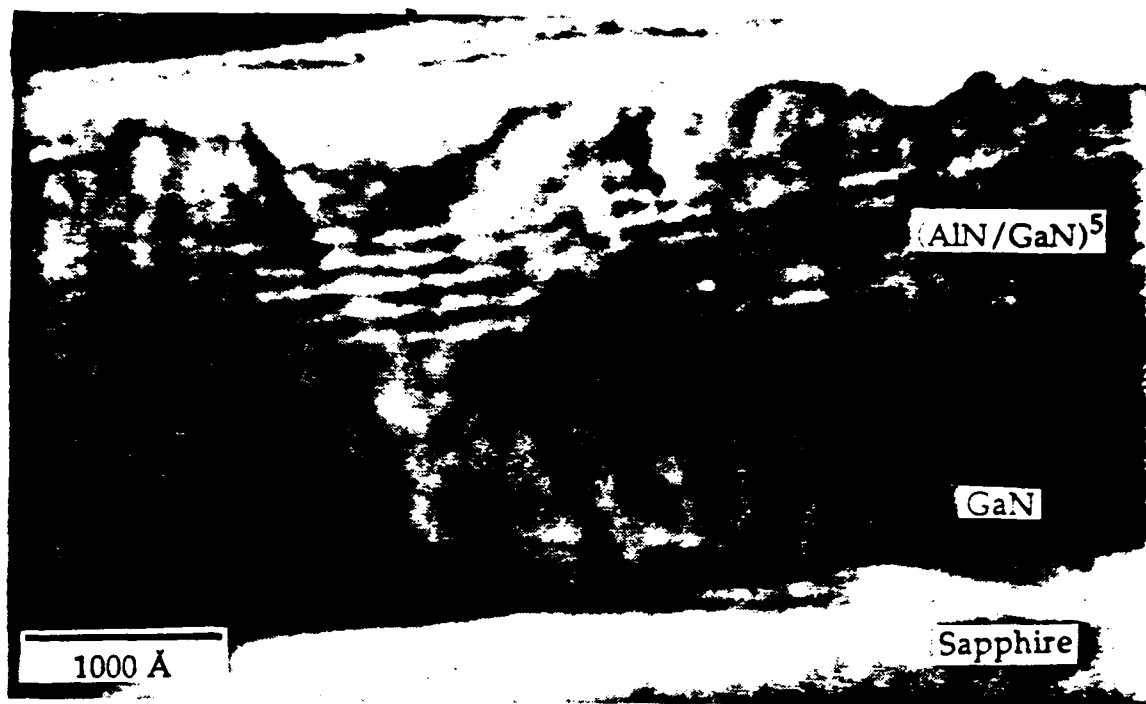
Figure 10. Cross-section TEM micrograph. Note the presence of the five AlN/GaN double layers (each single layer \approx 50-60 Å thick).
