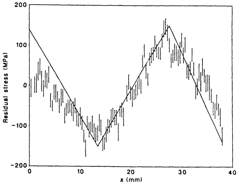
FIG. 19 AVERAGED SPATE AND STRAIN GAUGE STRESSES ACROSS BEAM CONTAINING RESIDUAL STRESSES
