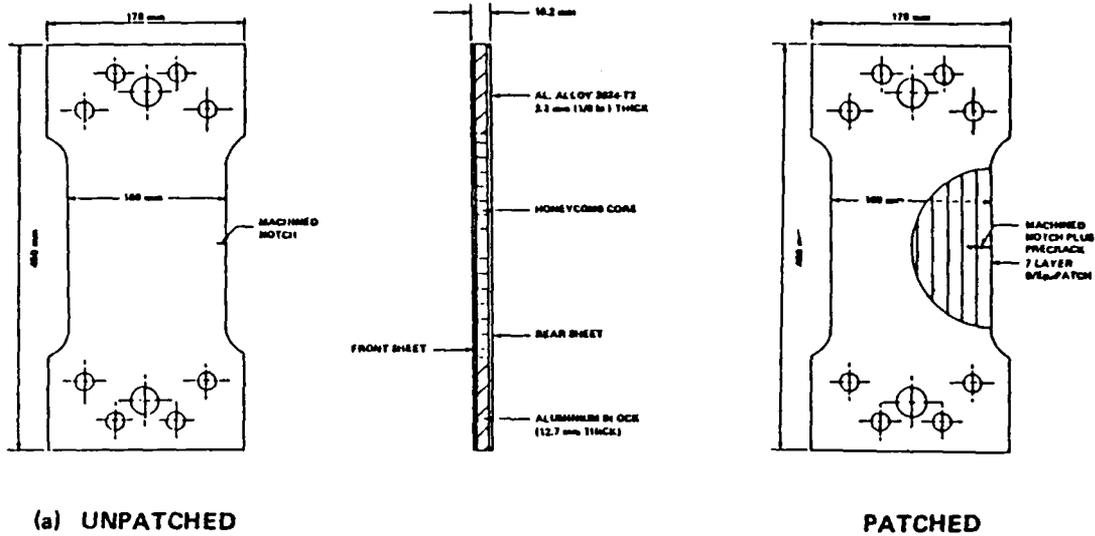
FIG. 21 UNPATCHED AND PATCHED HONEYCOMB TEST PANELS
