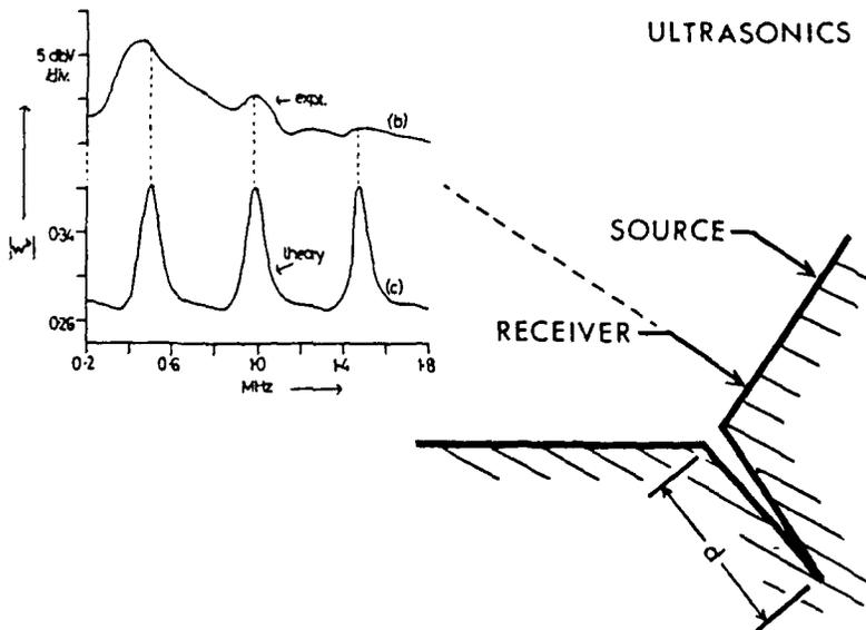
FIG. 28 DEPTH MEASUREMENT OF CORNER CRACKS USING ULTRASONIC RAYLEIGH WAVES
