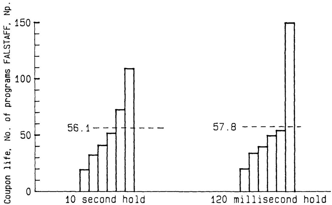
FIG. 24 EFFECT OF HOLD TIME ON LIFE OF IMPACT-DAMAGED COMPOSITE COUPONS UNDER FALSTAFF LOADING
