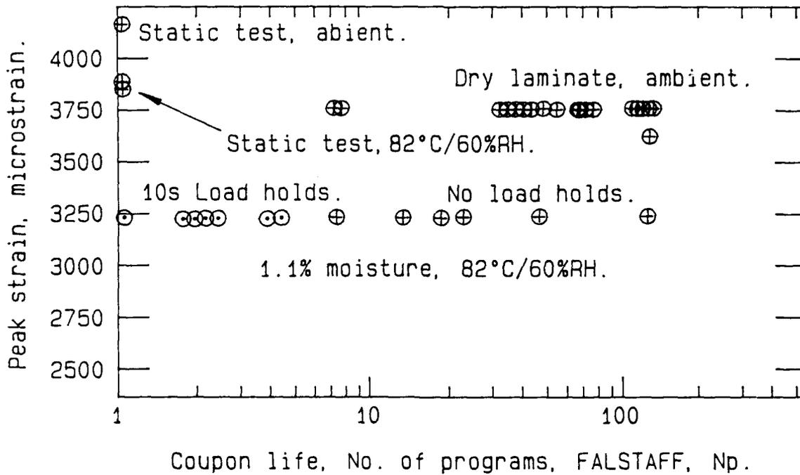
FIG. 26 EFFECT OF HOLD TIME ON FATIGUE LIFE OF 56-PLY XAS-914C LAMINATES
