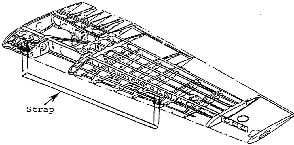
FIG. 11 CESSNA SERIES 400 SPAR REINFORCEMENT STRAP
