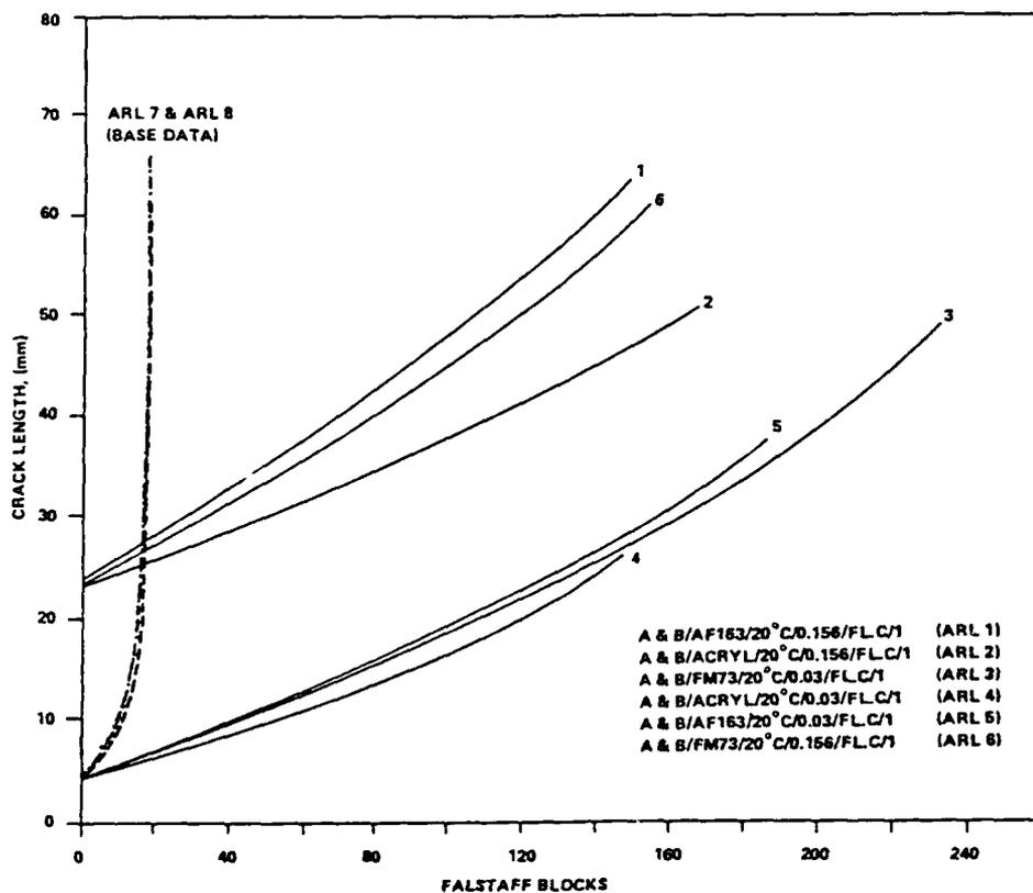
FIG. 22 CRACK GROWTH OF UNPATCHED AND PATCHED TEST PANELS
