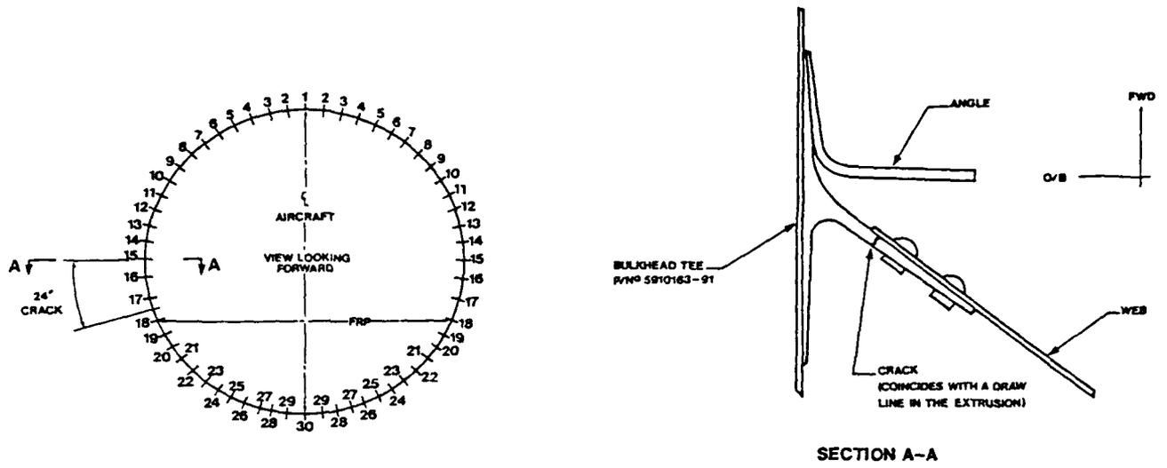
FIG. 9 DOUGLAS DC-9 REAR PRESSURE BULKHEAD ATTACHMENT
