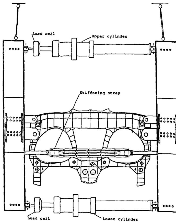
FIG. 6 F/A-18 BULKHEAD FATIGUE TESTING RIG
