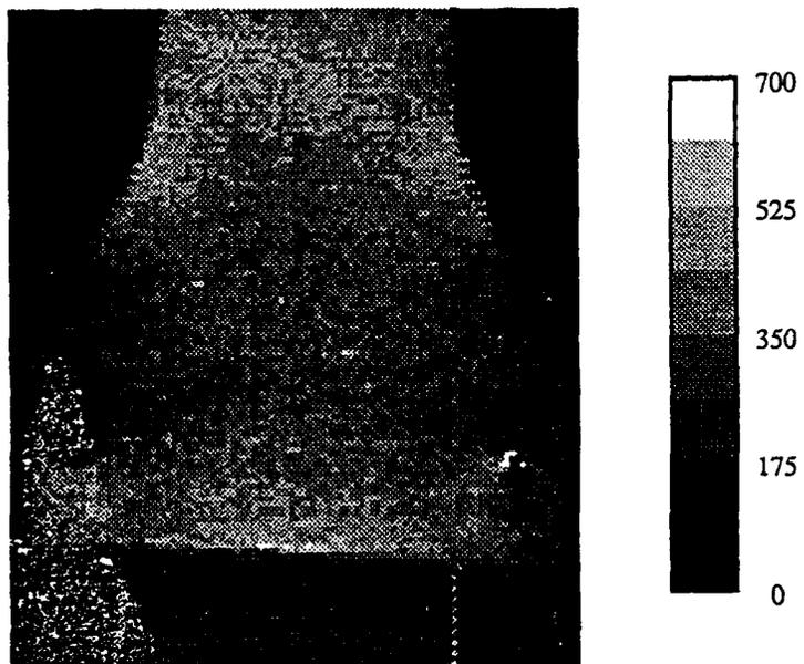
FIG. 8 SPATE SCAN OF F/A-18 F143 FILLET STRESSES
