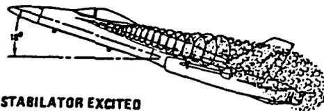
FIG. 4 VORTEX LOADING OF F/A-18 EMPENNAGE
