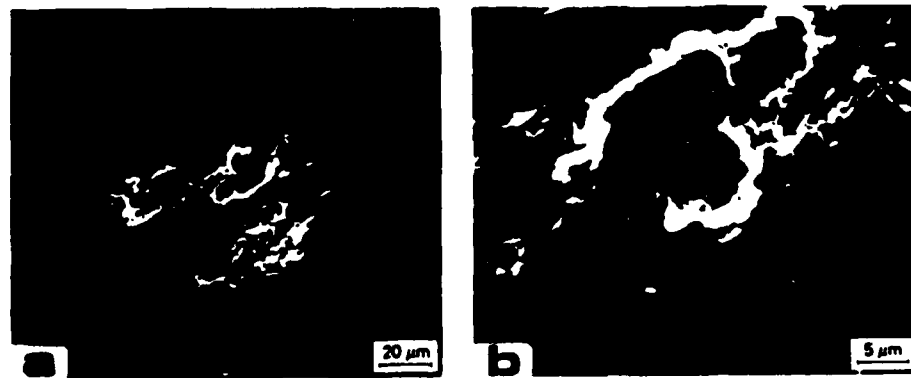
Fig. 5. (a) Worn surface of a chromium pin (lubricated test; normal load, 2 N; distance slid, 0.37 m (10 rev)). (b) Higher magnification of (a). The arrows show the sliding direction.
