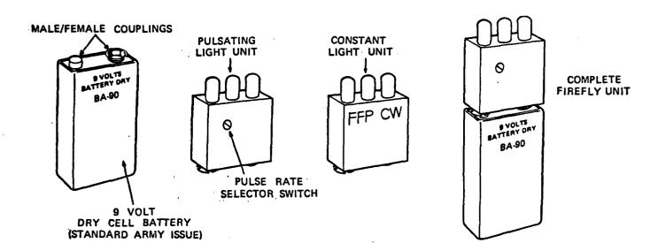
Figure E-1 The Firefly infrared emission device.
