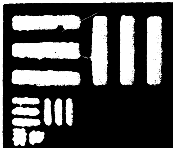
FIGURE 5a. Optical microscope image of the resolution test pattern. The pattern is etched in a 1000 \text{ \AA} free standing gold film and consists of lines and gaps of nominal widths 5 \mu\text{m} , 2 \mu\text{m} , and 1 \mu\text{m} . Over-etching has produced smaller lines and larger gaps.
