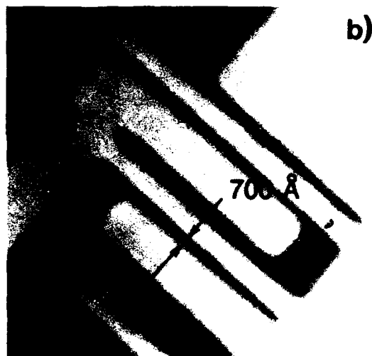
Figure 2.(a) A soft x-ray image, taken at 45\text{\AA} wavelength, of the gate level pattern associated with an experimental 0.1 micron MOSFET under development at IBM. The 1,000\text{\AA} (0.1 micron) gold bars are clearly resolved. The gold pattern is supported by an x-ray transmissive silicon nitride membrane of approximately 1,000\text{\AA} thickness. The image shown is one portion of a repetitive pattern which is approximately 30 microns across. (b) A soft x-ray image of two levels of the same MOSFET showing further pattern detail, including a clearly resolved 700\text{\AA} gap (0.07 micron) between gold fingers.
