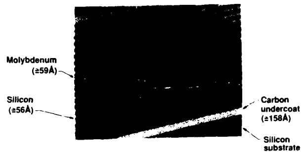
Figure 1(a): TEM micrograph of a Mo/Si multilayer mirror designed for x-ray laser cavity at 206.3\text{\AA} and 209.6\text{\AA} .
