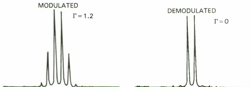
Figure 2-13. Spectral profiles of dual-carrier 1.319- \mu\text{m} laser radiation both before and after demodulation with an external cavity modulator. The external modulator was operated 180° out-of-phase and with the same depth of modulation as the intracavity modulator.
