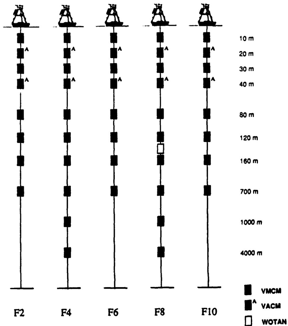
Figure 14. Mooring schematic for the FASINEX surface moorings.
