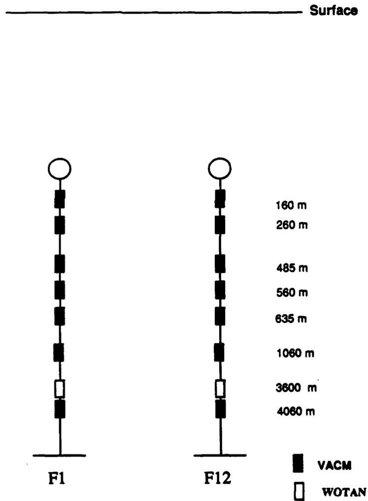
Figure 15. Mooring schematic for the FASINEX subsurface moorings.
