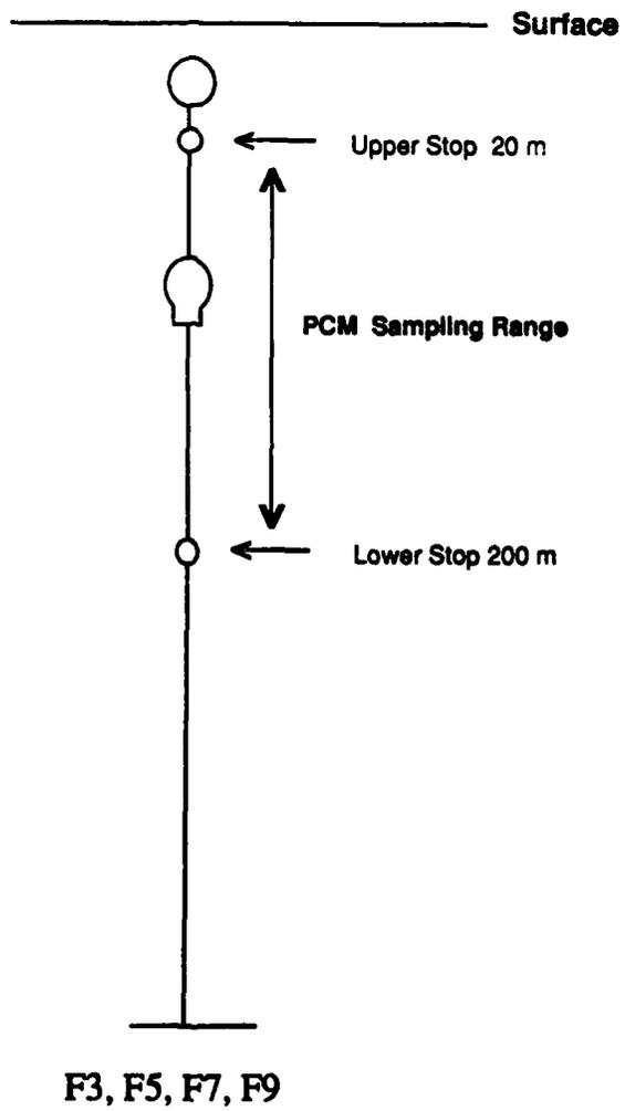
Figure 16. Mooring schematic for the PCM moorings.
