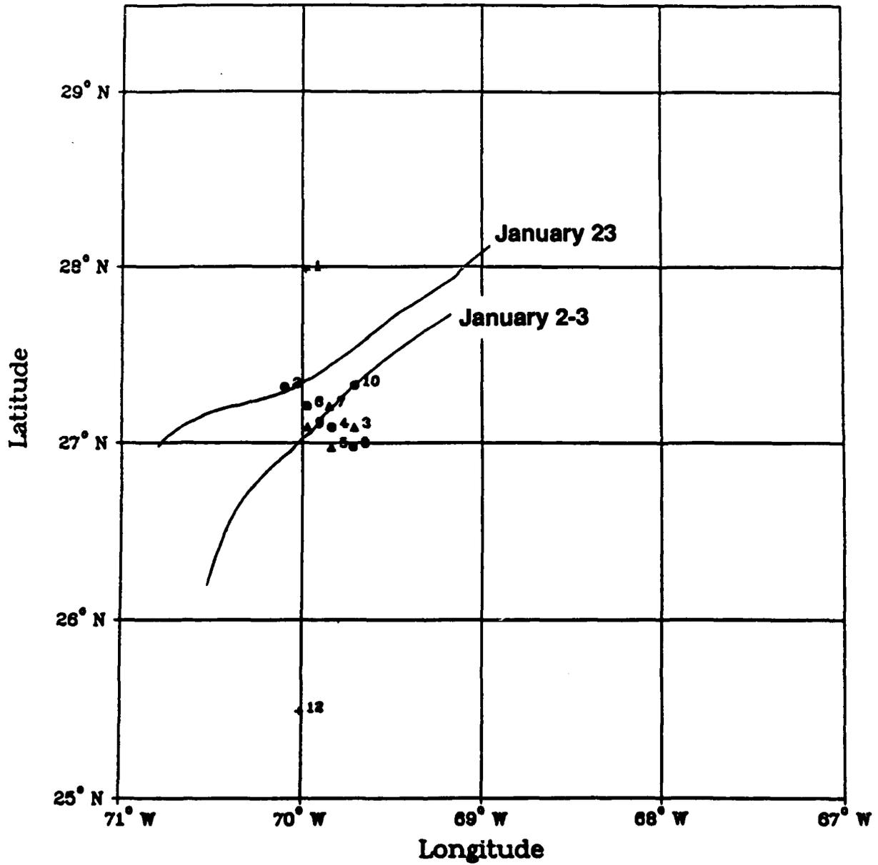
Figure 7. Anchor positions for the FASINEX surface and PCM moorings, showing their location relative to the frontal feature during the deployment cruise.
