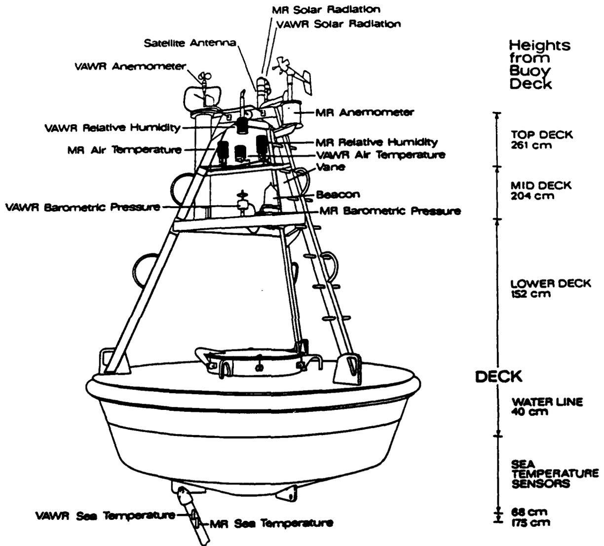
Figure 13. Meteorological sensors on FASINEX buoy.
