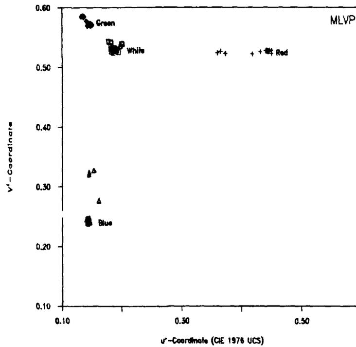
Figure 22. Variations in Chromaticity Among Display Sectors. Measurements of chromaticity at maximum output for three primaries and white at the center of each of nine equal sectors of the display. Top: Talaria SLVP; bottom: MLVP. Measurements made in June 1988.
