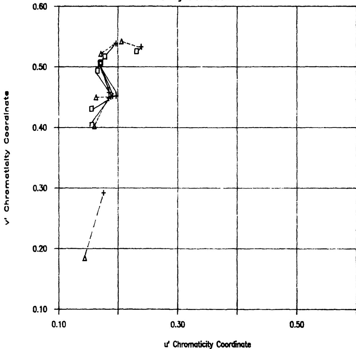
Figure 6. Chromaticity Points of the Nine Colors from the Scene Color Study. Crosses show the colors as measured on the modelers' Mitsubishi CRT, squares as measured in the dome AUI, and triangles as measured in the dome background. Corresponding points in the CRT and AUI displays are connected by solid lines; corresponding points in the CRT and background displays are connected by dashed lines.
