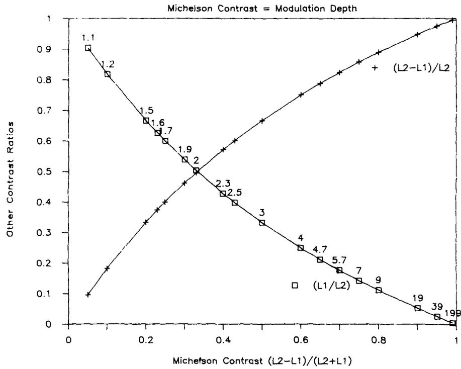
Figure B-1. Relation of L/D Ratio, Luminance Ratio, and Raster Response to Michelson Contrast.
