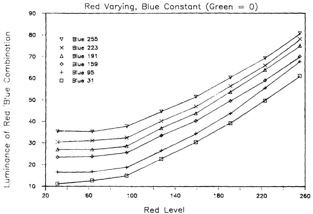
Figure 17. Talaria Test for Red/Blue Independence. Top: luminance output as a function of blue video level; separate curves are for different video levels of the red primary. Bottom: luminance output as a function of red video level; separate curves are for different video levels of the blue primary. Measurements made in June 1987; green primary at zero for all curves.
