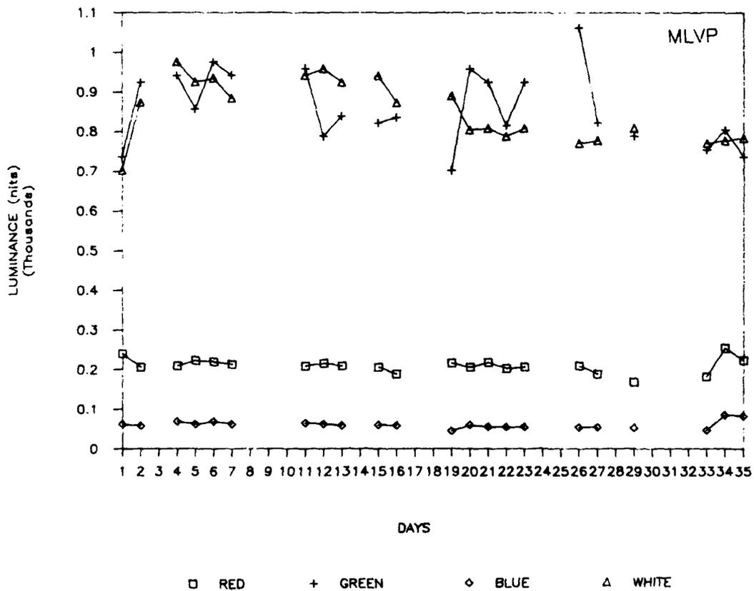
Figure 24. Day-to-Day Variations in LVP Output Luminance. Measurements were made over a 35-day period at maximum output of three primaries and white. Top: Talaria SLVP; bottom: MLVP.
