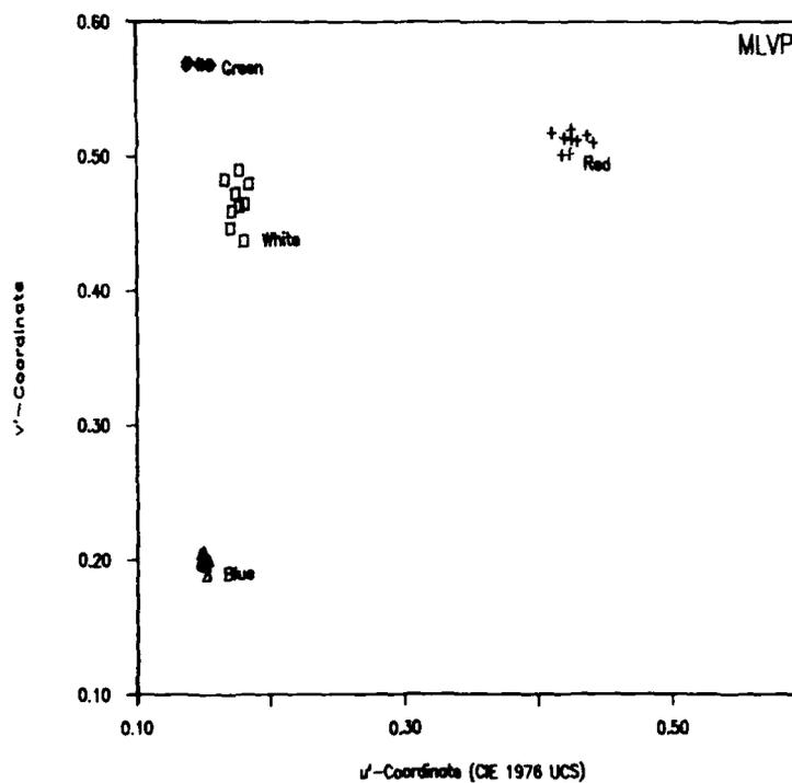
Figure 25. Day-to-Day Variations in LVP Chromaticity. Top: Talaria SLVP; bottom: MLVP. This figure may be compared with Figure 22, but it should be remembered that the data in Figure 22 derive from June 1988, after the MLVP had been upgraded and the SLVP had been supplied with a new light valve. Measurements for this figure were made in November and December 1987.
