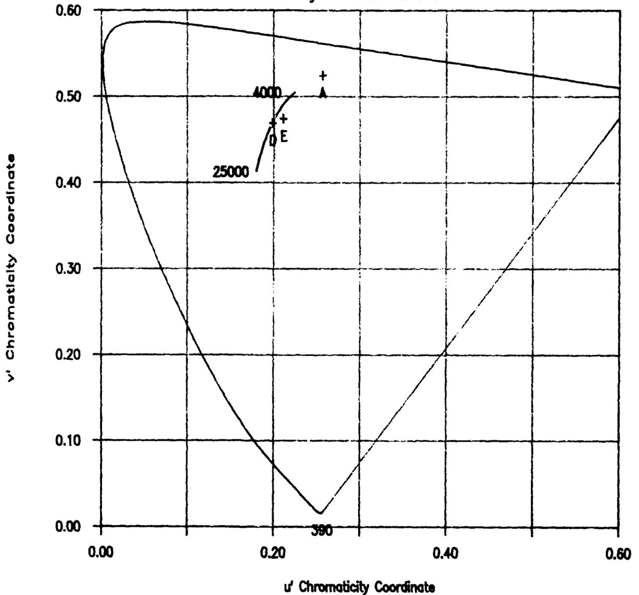
Figure 5. Spectrum Locus and Purple Boundary in the 1976 CIE Uniform Chromaticity Space (UCS). Also shown are the Planckian locus between 4,000° and 25,000°K, the chromaticity points of illuminants A and D65, and the chromaticity point for an equal energy spectrum (at E). This space is a linear transformation of the space shown in Figure 4.
