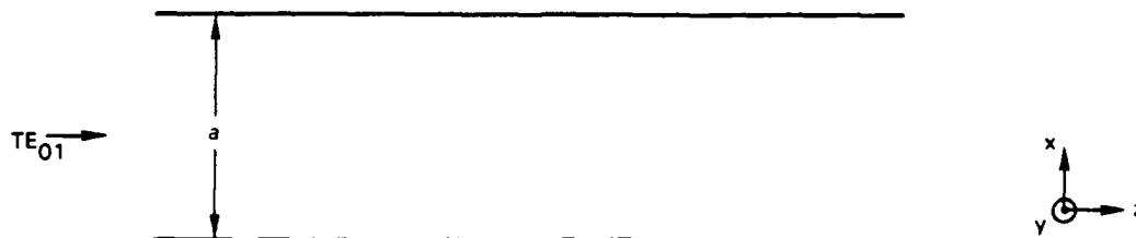
FIGURE C-1. Geometry for the Simple Parallel-Plate Waveguide With No Discontinuities.
