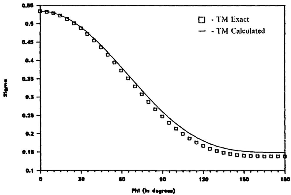
Figure 40. Cylinder, TE and TM Case,  $k_0a = 0.5$ ,  $\epsilon_r = 25.6$
