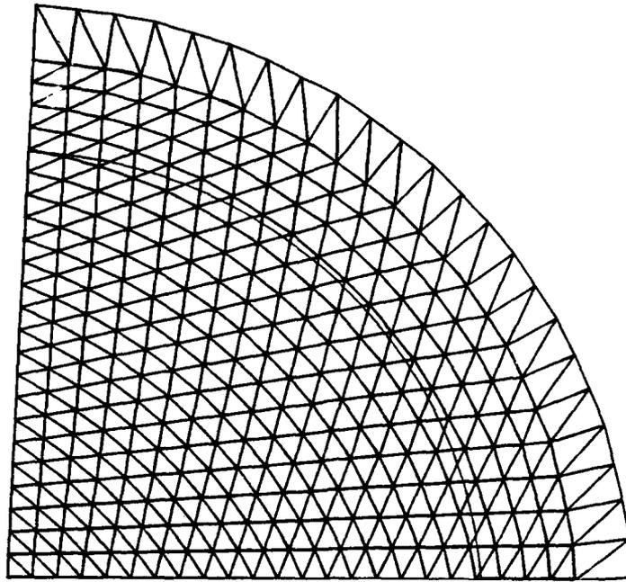
**Figure 44. Partial Mesh with Inner Radius Curve**
