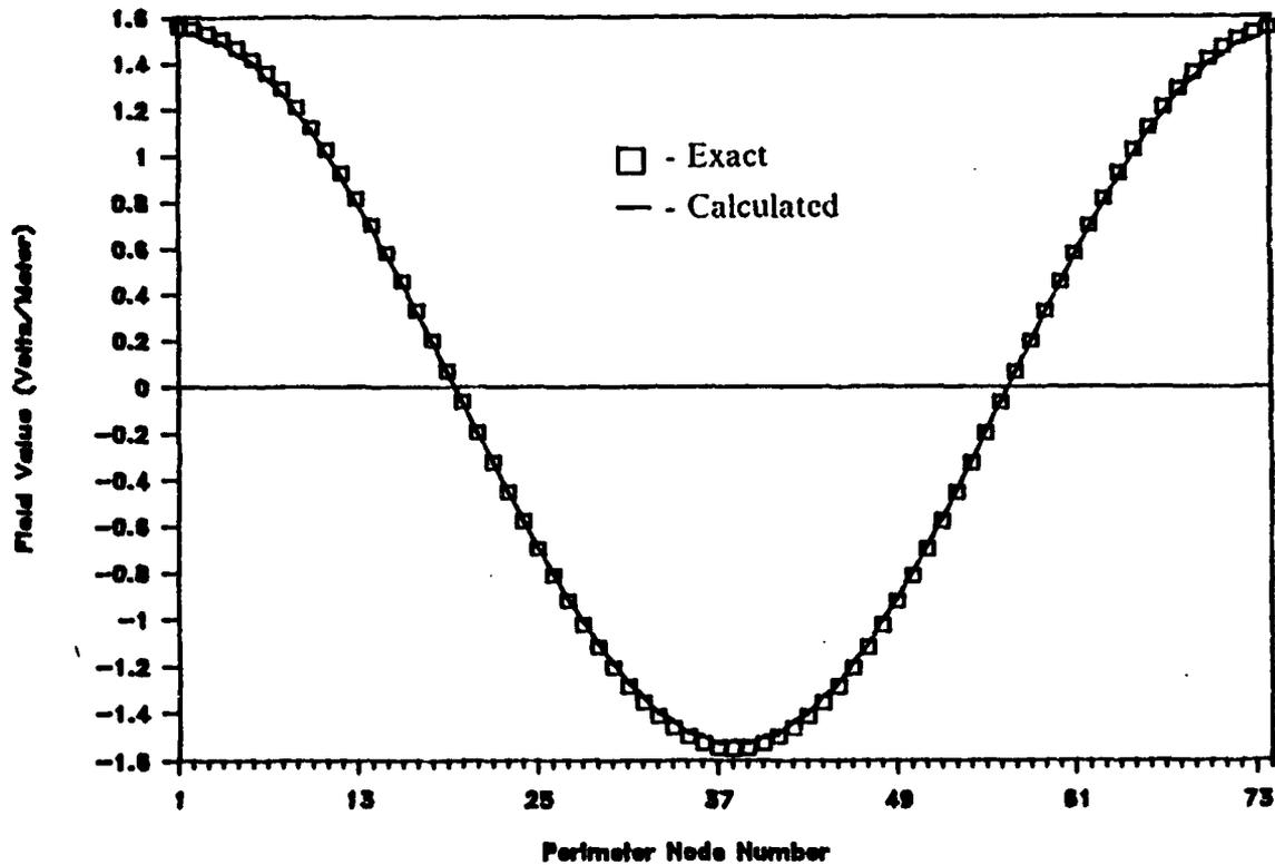
Figure 35. Typical Cylindrical Mode Boundary Value Problem Result
