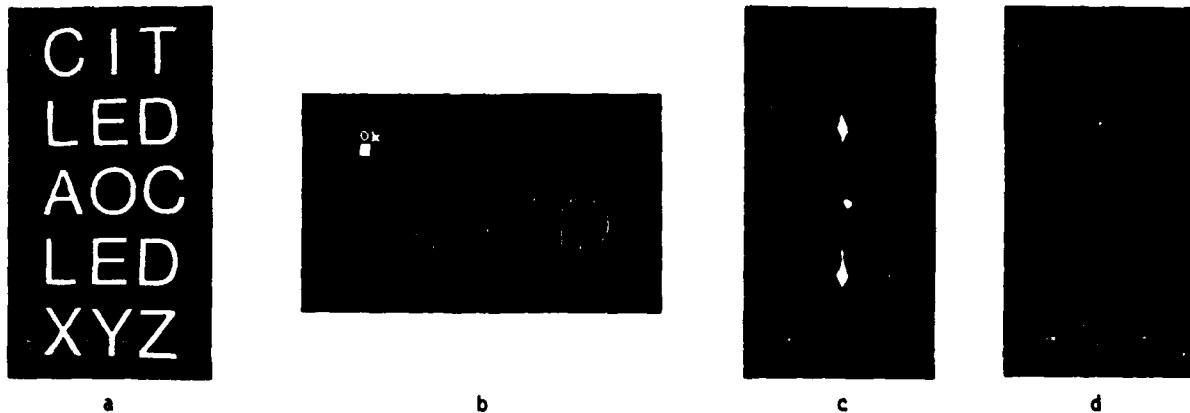
Figure 9. Experimental demonstration of incoherent LED correlator. (a) Input. (b) Reference image. (c),(d) Correlation output.
